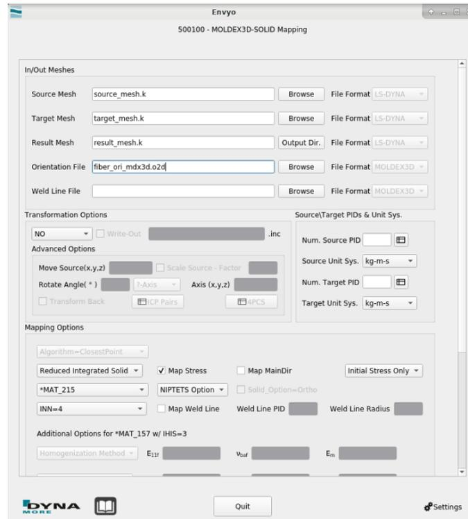
Fig.8: Envyo GUI für Moldex3D to solid element mapping
