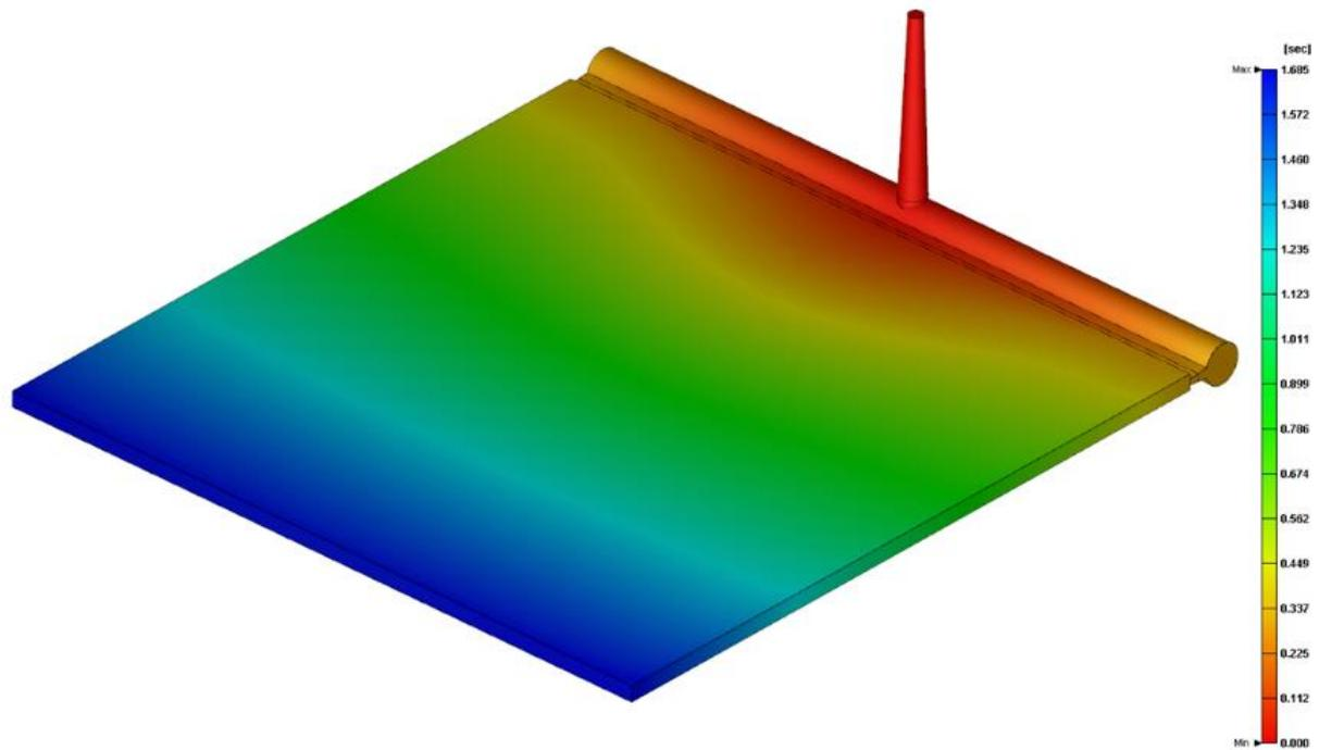
Fig.3: *Melt front time, time for melt front to reach a certain position, injection gate and runner also visible*
