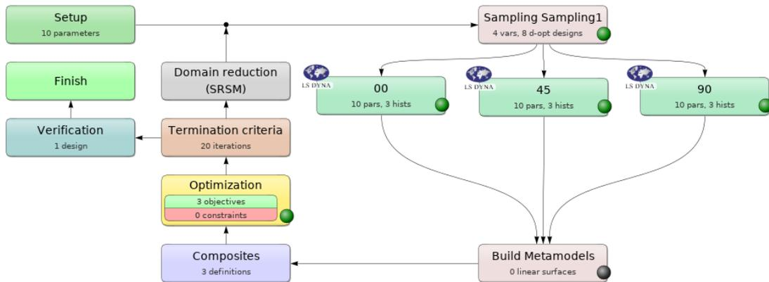
Fig.13: LS-OPT setup of the hardening calibration.
