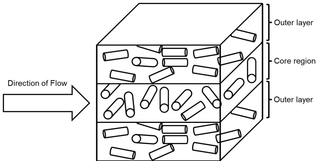
Fig.1: Simplified depiction of the flow induced through thickness anisotropy in fiber orientation
