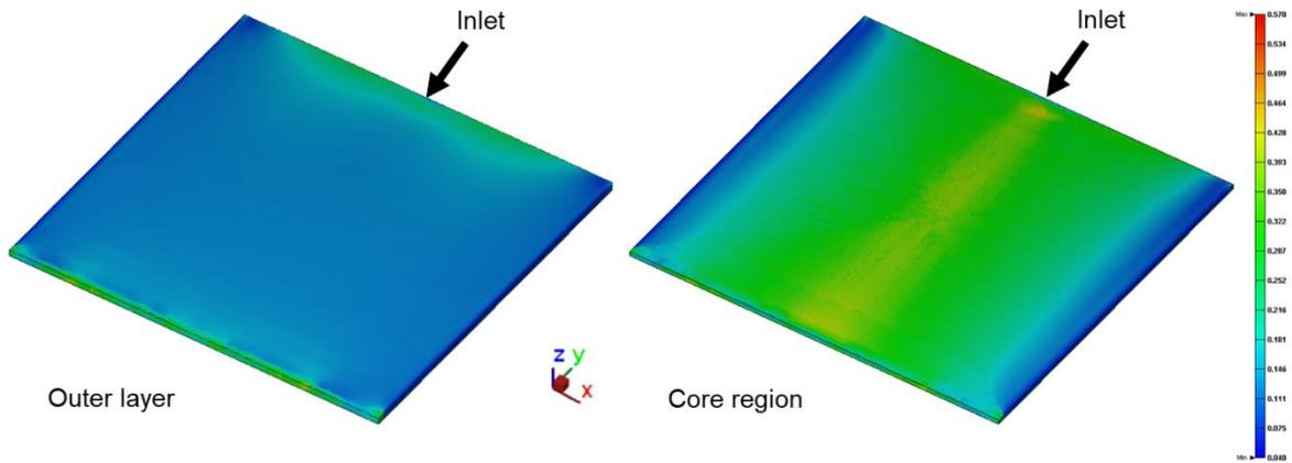
Fig.5: Degree of fiber orientation in the X direction, cut at 75 % thickness (outer layer) and at 50 % thickness (core region)
