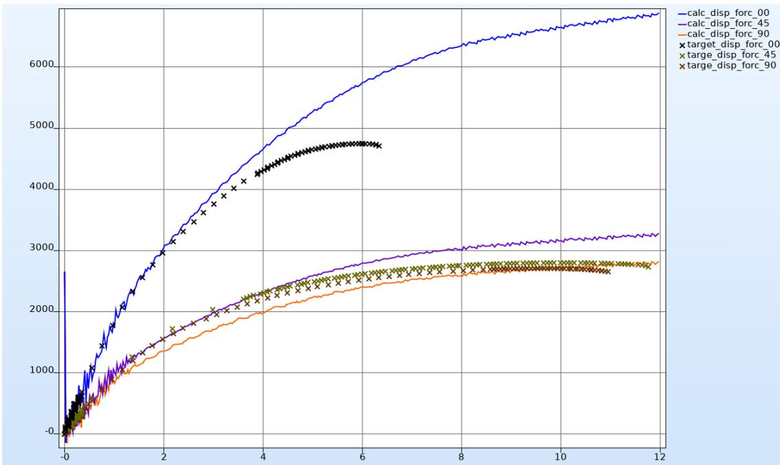
Fig.16: Comparison of simulation and experimental results using the manually found optimum hardening.
