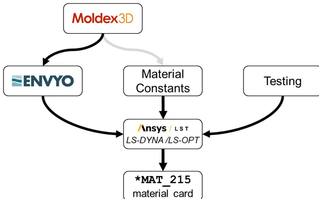
Fig.2: Flow chart of the methodology for characterization of the material
