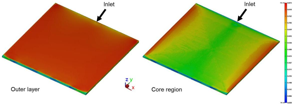
Fig.4: Degree of fiber orientation in the Y direction, cut at 75 % thickness (outer layer) and at 50 % thickness (core region)
