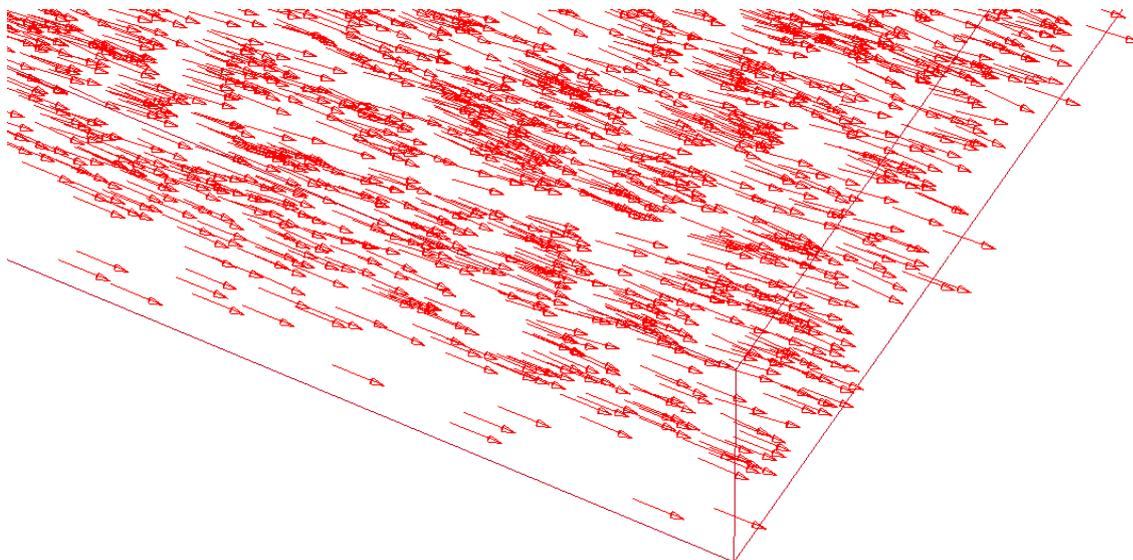
Fig.9: Sample of mapped fiber result in viewed LS-PrePost for the 0° specimen
