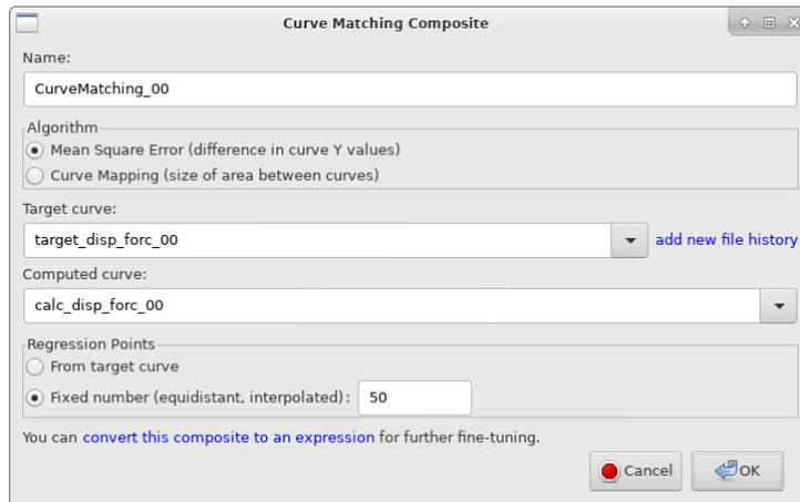
Fig.12: Setup of curve matching composite in LS-OPT.
