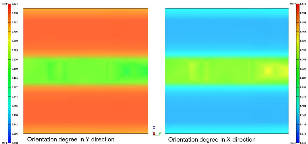
Fig.6: Degree of fiber orientation through the thickness, cut view is at middle of the plate normal to the X direction
