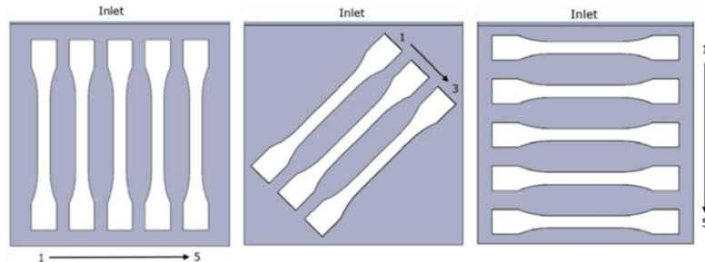
Fig.10: Specimen cut out for 0°, 45°, and 90°
