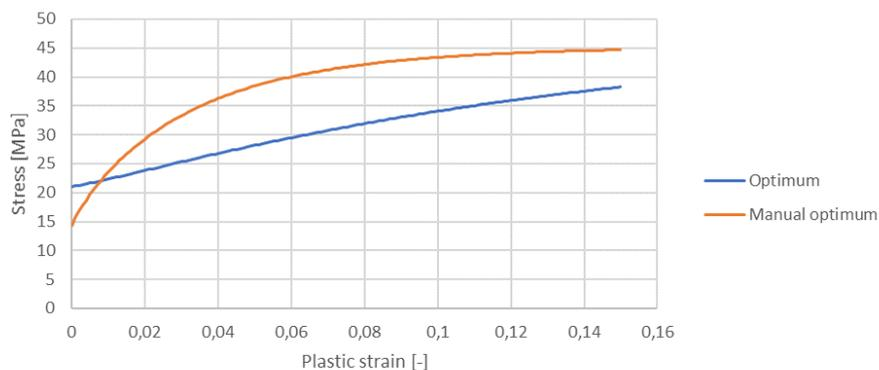
Fig.14: Hardening curves retrieved by the optimization and the manual calibration using the approximate histories function, respectively.
