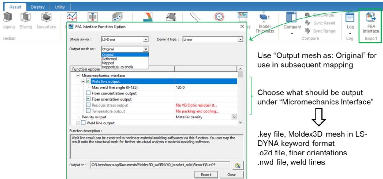
Fig.7: FEA/Micromechanics interface in Moldex3D
