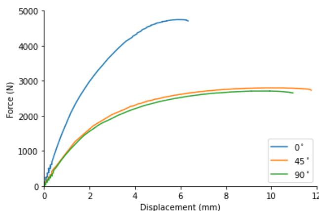
Fig.11: Force vs. displacement for 0°, 45°, and 90° oriented tensile specimens
