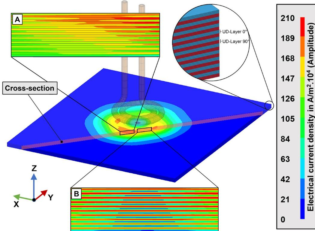
Fig.14: Distribution of current density at different locations of the laminate: **A** at crossover areas; **B** between crossover areas.
