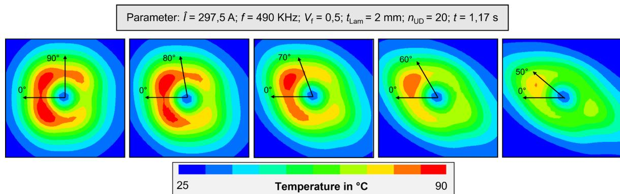
Fig.17: Influence of ply orientation in the laminate on the resulting heating pattern on the backside of the laminate.
