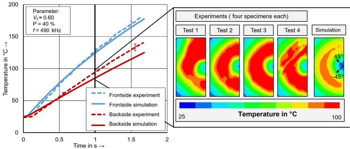
Fig.12: Comparison of simulation and experimental heating curves at front and back side of NCF-60% laminate (left) and heating patterns on back side at  $t = 1 \text{ s}$ .
