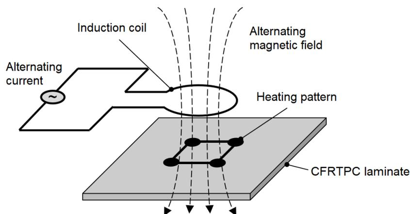
Fig. 1: Setup for induction heating of CFRTPC laminates according to [2].
