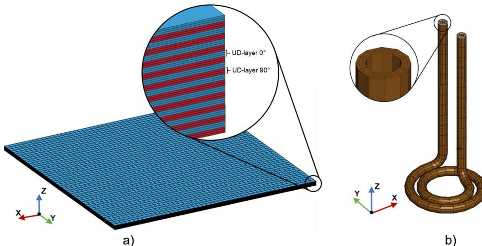
Fig.8: Mesh geometry of a) the laminate using the example of a 20-ply 0/90 NCF laminate. Each UD ply has three elements in the thickness direction and 50 elements in the X and Y direction and b) the pancake coil inductor
