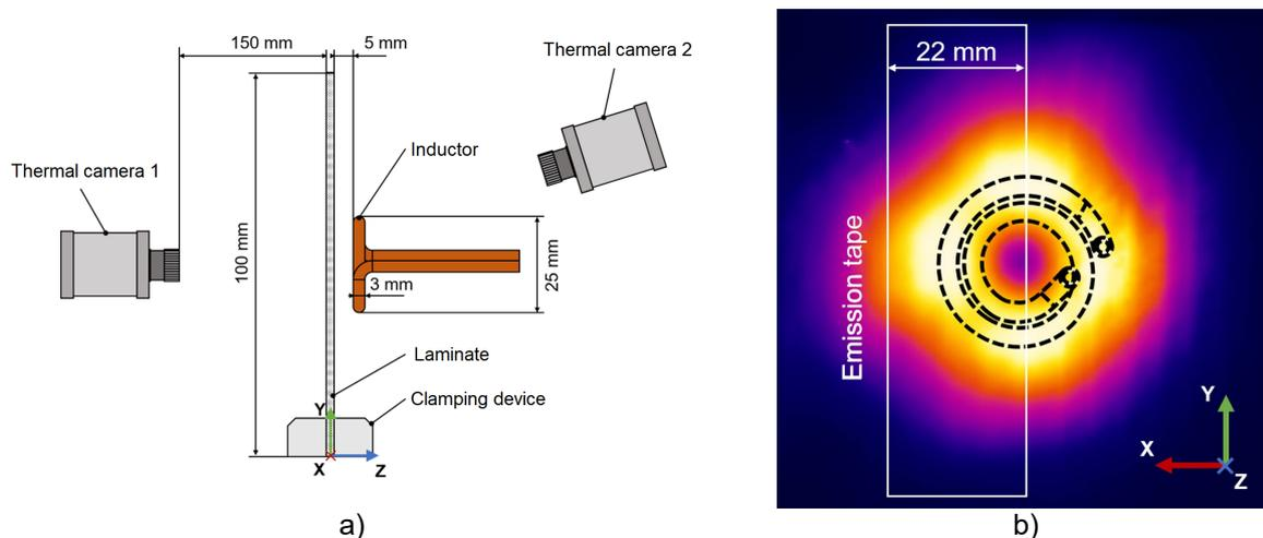
Fig.9: Overview of the experimental setup of the validation tests a) (side view) and b) positioning of the emission tape using the example of the back of the laminate relative to the contour of the inductor located on the opposite side of the laminate (Thermal camera 1 view).
