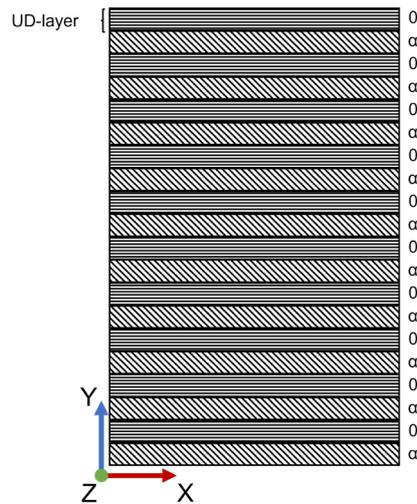
Fig.16: Schematic representation of the layer structures used for the investigation of the influence of the layer orientation on the laminate heating behavior.
