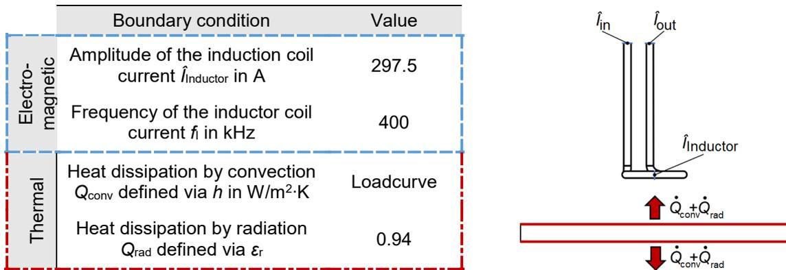
Fig.6: Overview and schematic representation of the electromagnetic (blue) and thermal (red) boundary conditions defined in the LS-DYNA® FE model.
