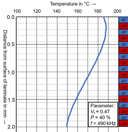
Fig. 13: Temperature curve in thickness direction of the laminate at the point of maximum temperature development. The thickness of the laminate is 2.3 mm.
