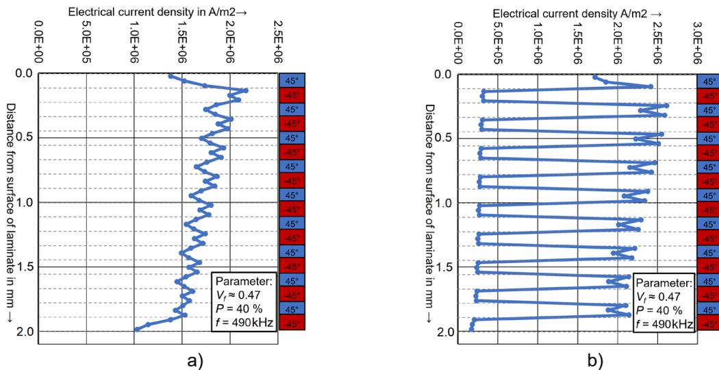
Fig.15: Course of the current density in the thickness direction of the laminate between the crossover areas (a), area **A**, Figure 14) and at the point of maximal heating (b), area **B**, Figure 14).
