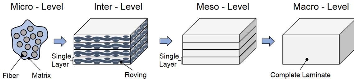
Fig.5: Different levels of material homogenization considered for the FE modeling of CFRTPCs [5].
