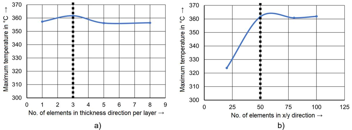
Fig.7: Influence of the number of elements in the thickness direction per UD- ply a) and elements in-plane of the laminate b) on the maximum temperature developed in the laminate.
