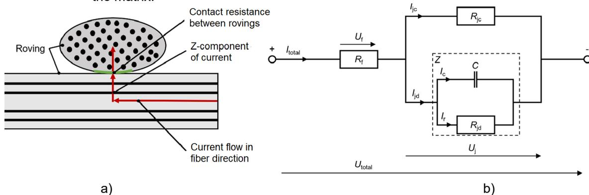
Fig.4: Schematic representation of a) the current flow when changing the fiber orientation and b) its representative electrical circuit.
