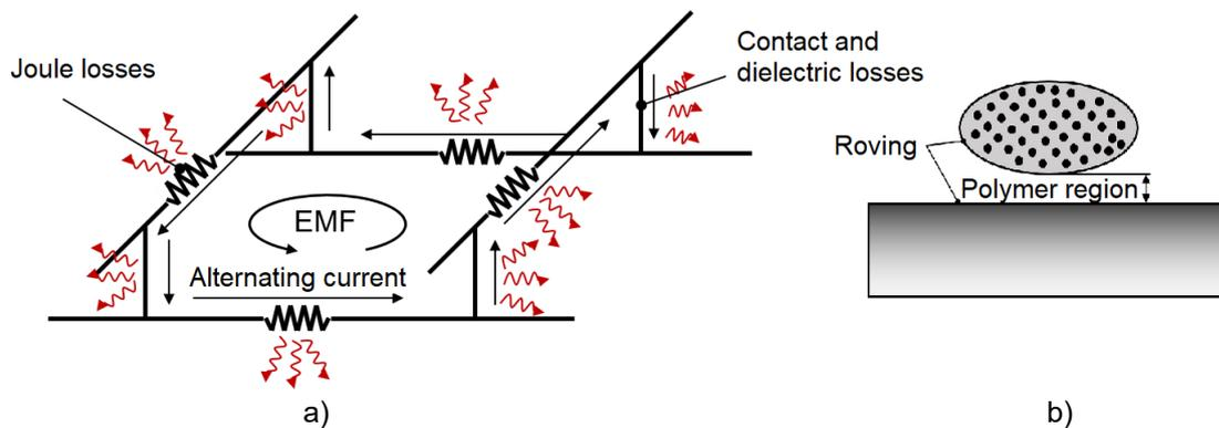
Fig.2: a) Model of a conductor loop with the joule, contact and dielectric losses according to [3] and b) the polymer region in which dielectric losses occur according to [4].
