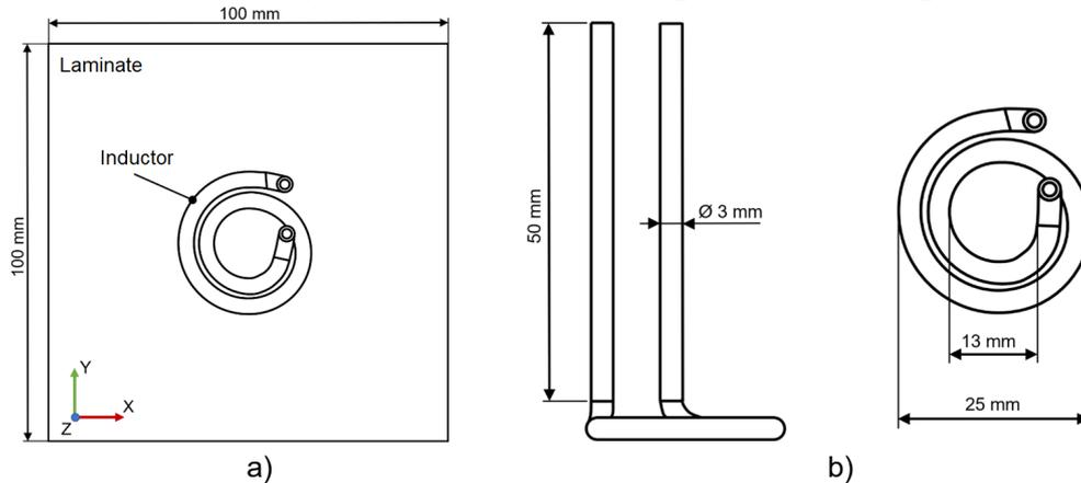
Fig.3: Schematic representation of a) the complete FE model and b) the induction coil geometries.
