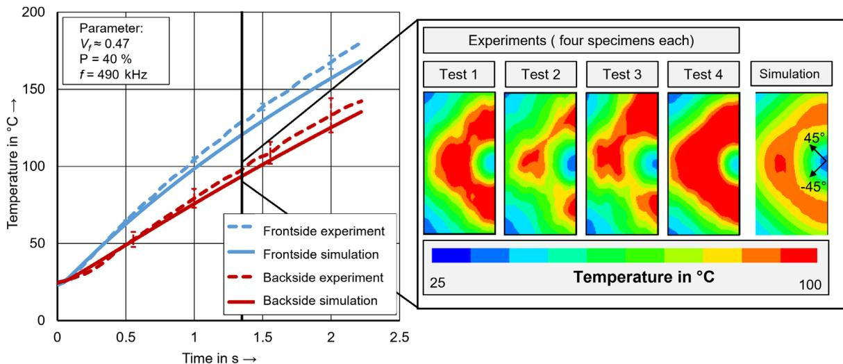
Fig. 11: Comparison of simulation and experimental heating curves at front and back side of NCF-47% laminate (left) and heating patterns on back side at  $t = 1.3\text{ s}$ .
