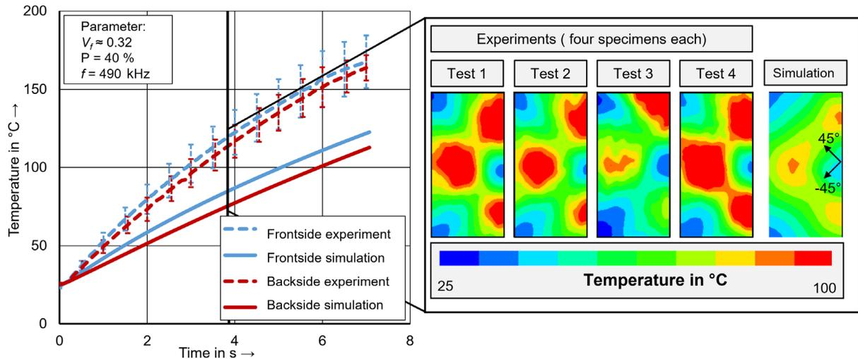
Fig. 10: Comparison of simulation and experimental heating curves at front and back side of NCF-32% laminate (left) and heating patterns on back side at  $t = 3.9\text{s}$ .
