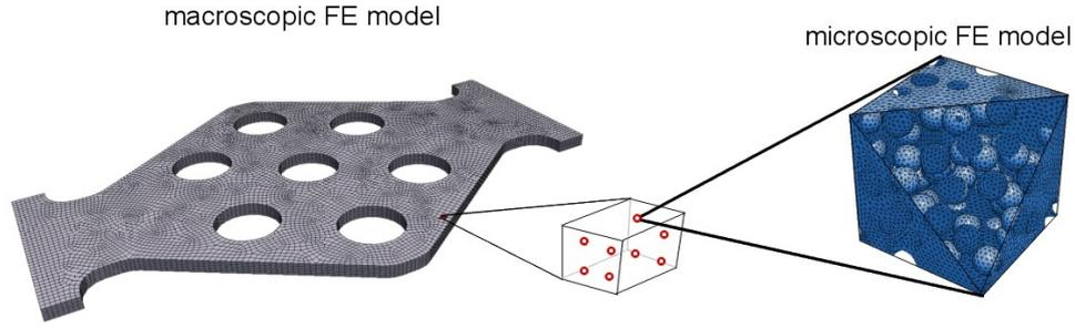
Fig 1. Illustration of the implementation of the FE<sup>2</sup> framework
