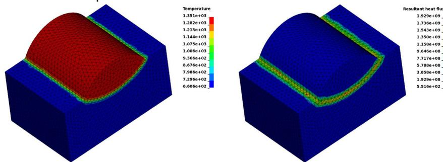
Fig 7. Homogenized response of two-phase structure.
