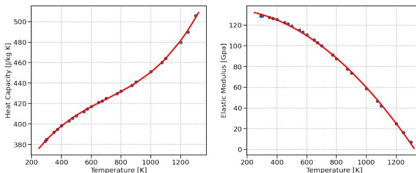
Fig 4. Temperature dependent material parameters of OFHC.
