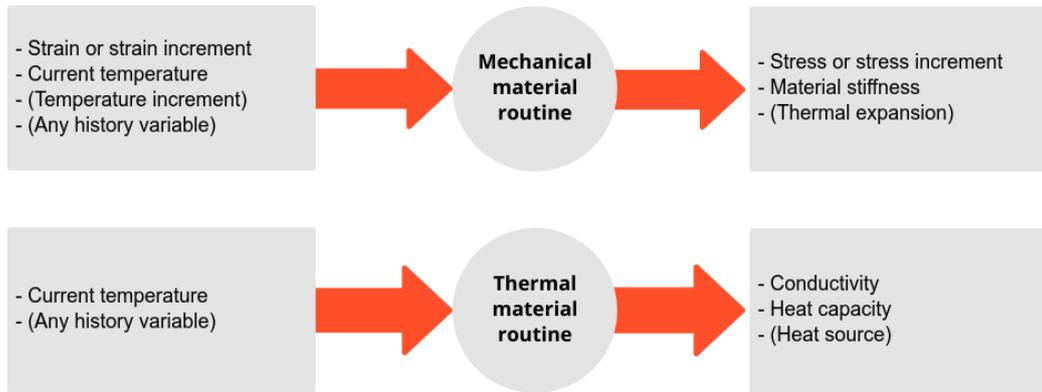
Fig 2. Illustration of how material routines are called.
