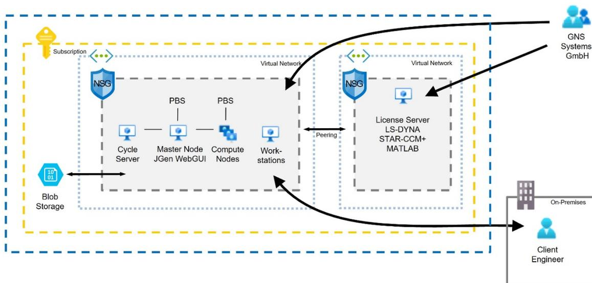
Fig. 1: Overview of the Cloud Architecture
