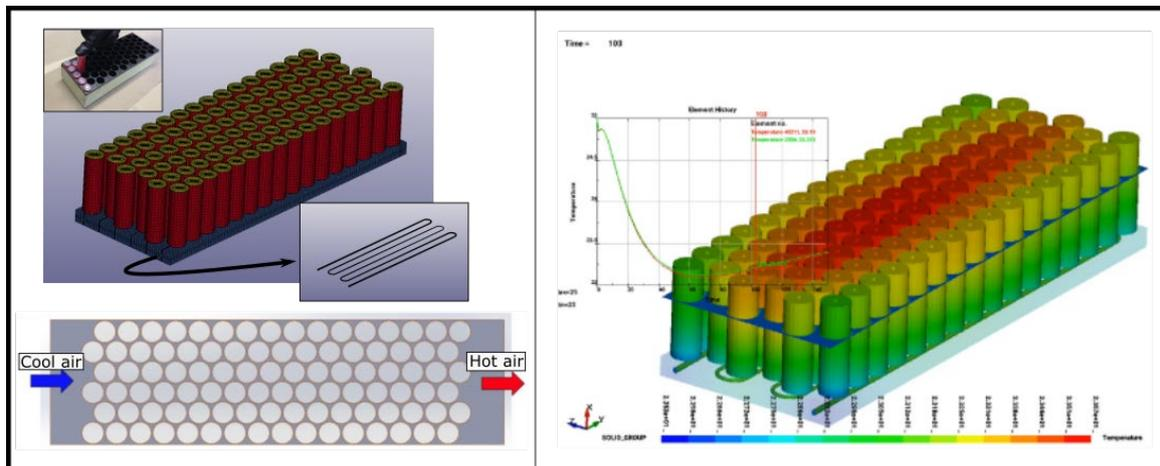
Fig.5: Battery pack cooling using air and a liquid flowing inside the serpentine.
