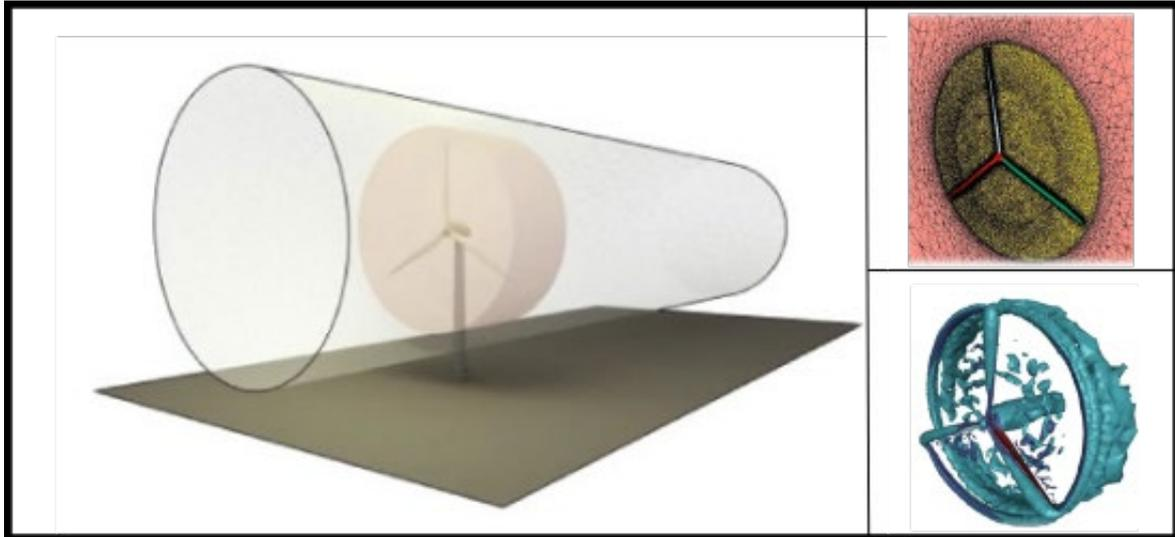
Fig.1: Wind turbine with sliding mesh domain shown in red. Left: details of the mesh used for the simulation (top) and results (bottom).
