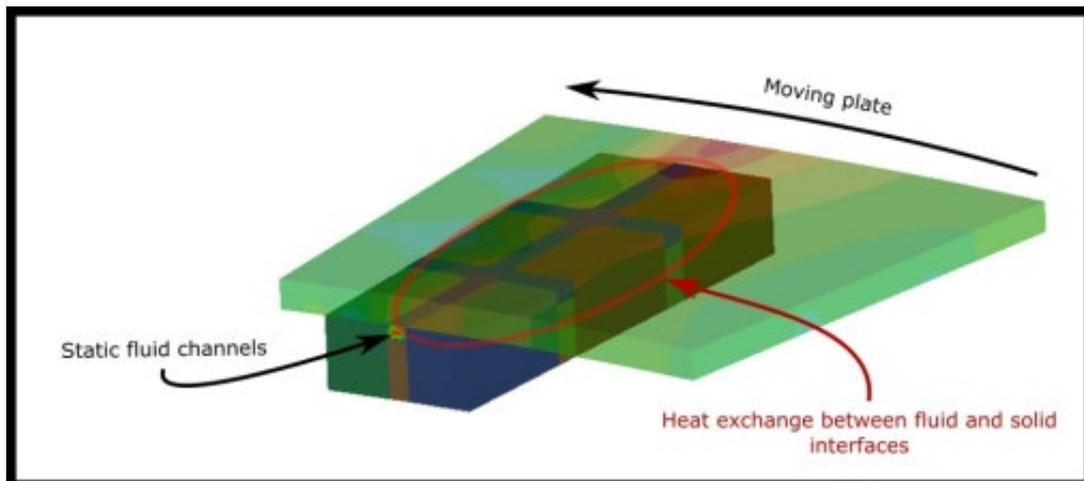
Fig.7: Clutch cooling simulation. The heat generated through friction between the moving plate and the pad is cooled down using fluid channels.
