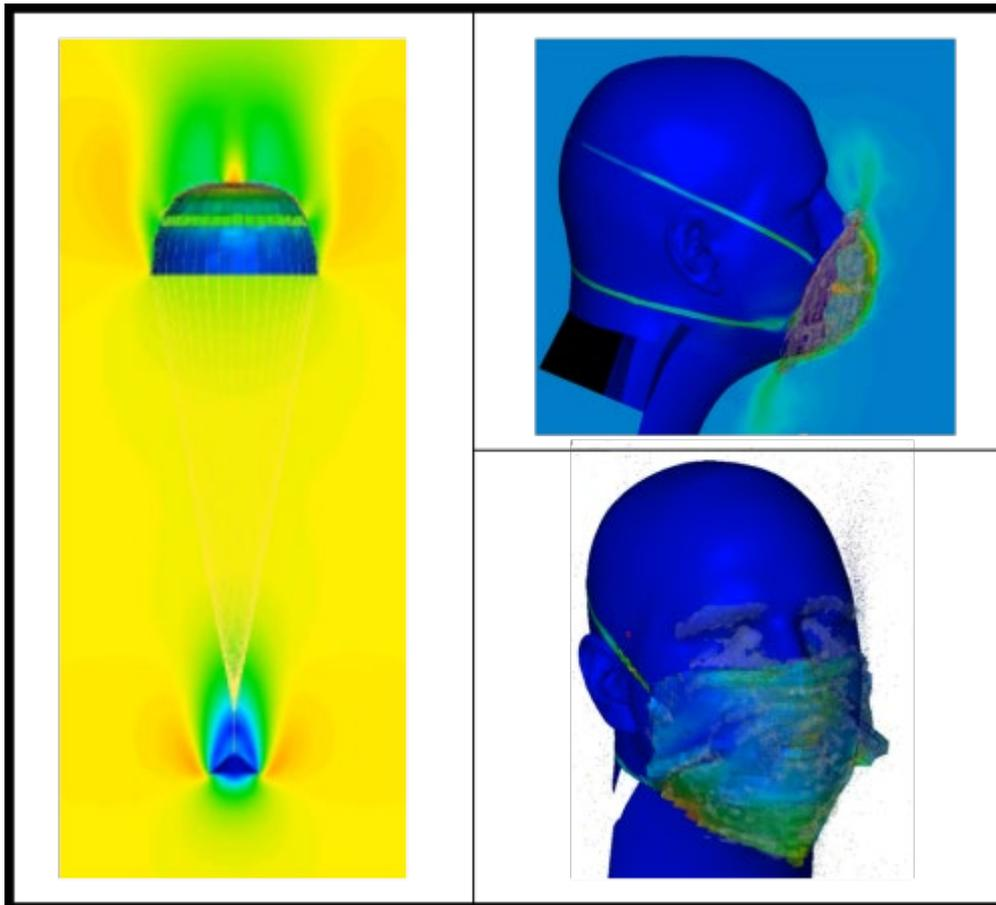
Fig.3: FSI simulation of a parachute (left) and face masks using porous models on membranes.
