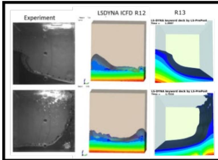
Fig.6: Comparisson between experiment, R12 and the improved R13 solution for the level set.
