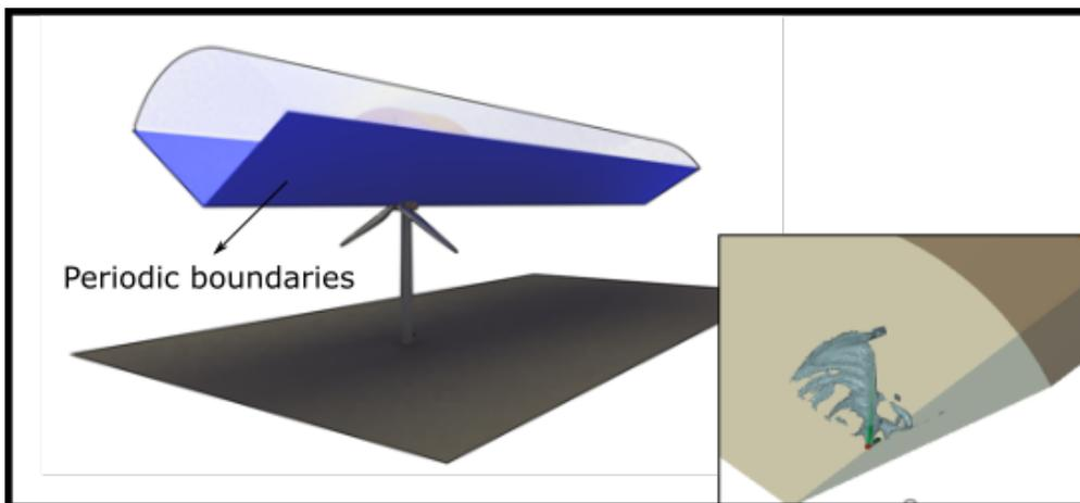
Fig.2: Wind turbine with a periodic boundary domain. Left: iso-surface of fluid velocity for the one blade simulation result.
