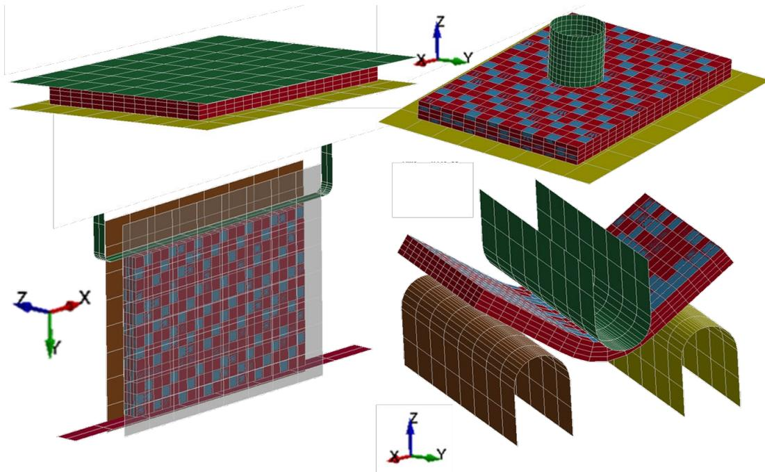
Fig.4: Experimentally investigated and simulated load case scenarios for the simplified model approach of pouch cells
