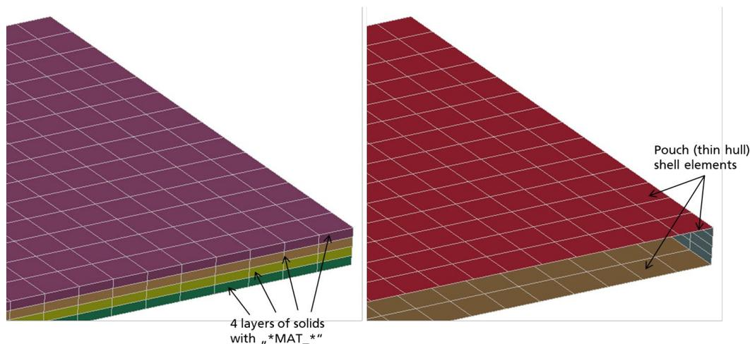
Fig.3: Principle setup and element discretization for the simplified model of a pouch cell
