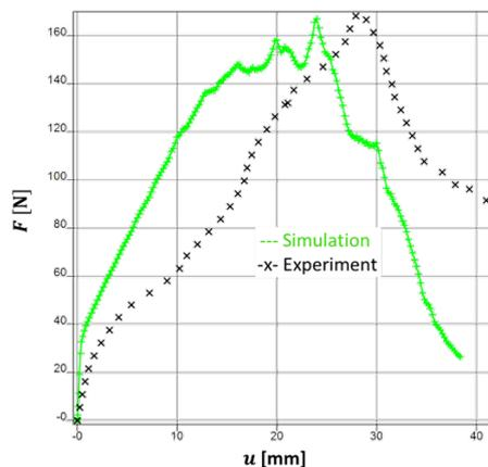
Fig.9: Comparison between simulation and experiments of force-displacement curves for three-point bending test by using `*MAT_MODIFIED_HONEYCOMB`
