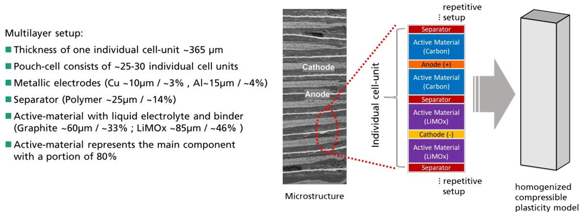
Fig.1: Typical layered setup of a cell-unit within Li-ion battery.
