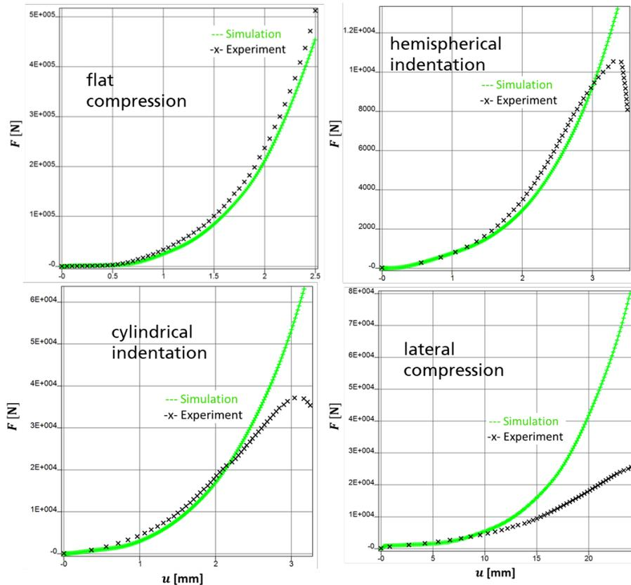
Fig.5: Comparison between simulation and experiments of force-displacement curves for different load cases by using \*MAT\_CRUSHABLE\_FOAM
