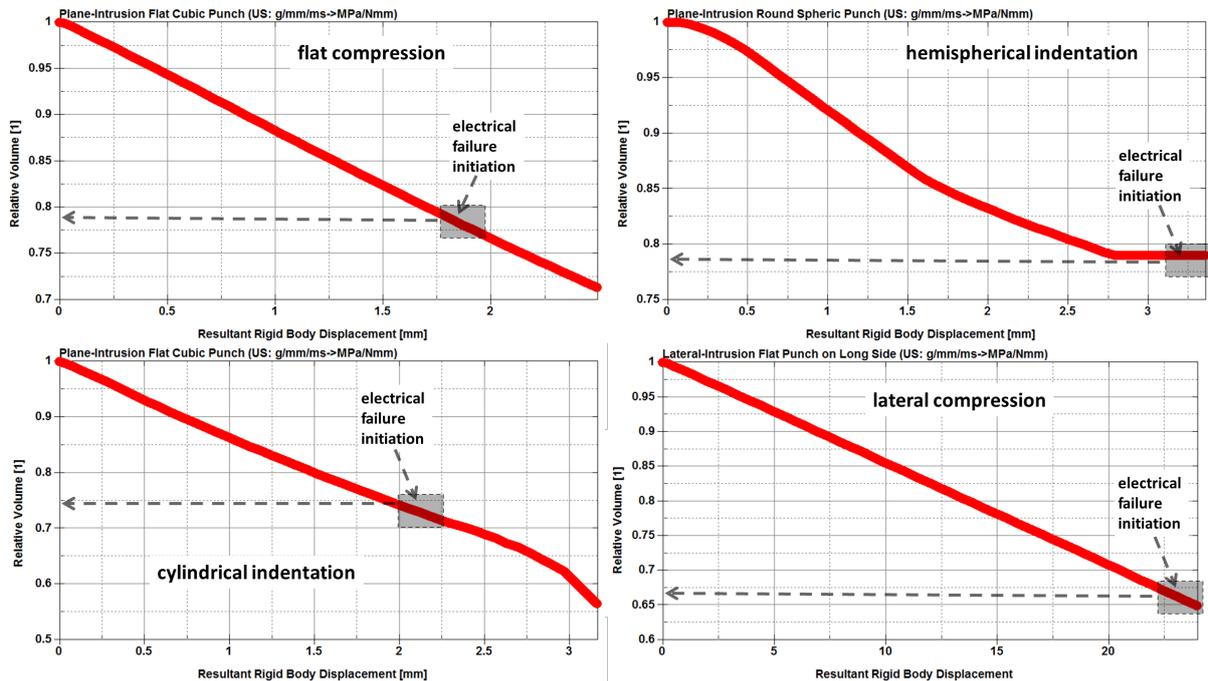
Fig.10: Comparison of (initial) electrical short circuits (grey rectangular) in relation to the evolution of relative volume (directly related to volumetric stain) for different load case scenarios
