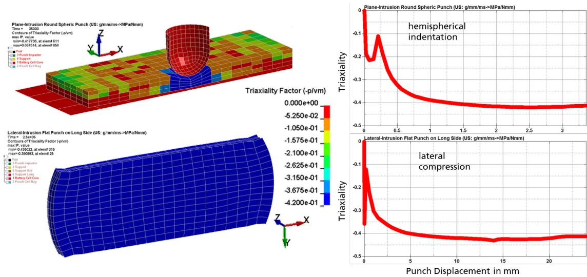
Fig.7: Triaxialities for hemispherical indentation and lateral directed compression (left) and the corresponding evolution of Triaxialities (right)
