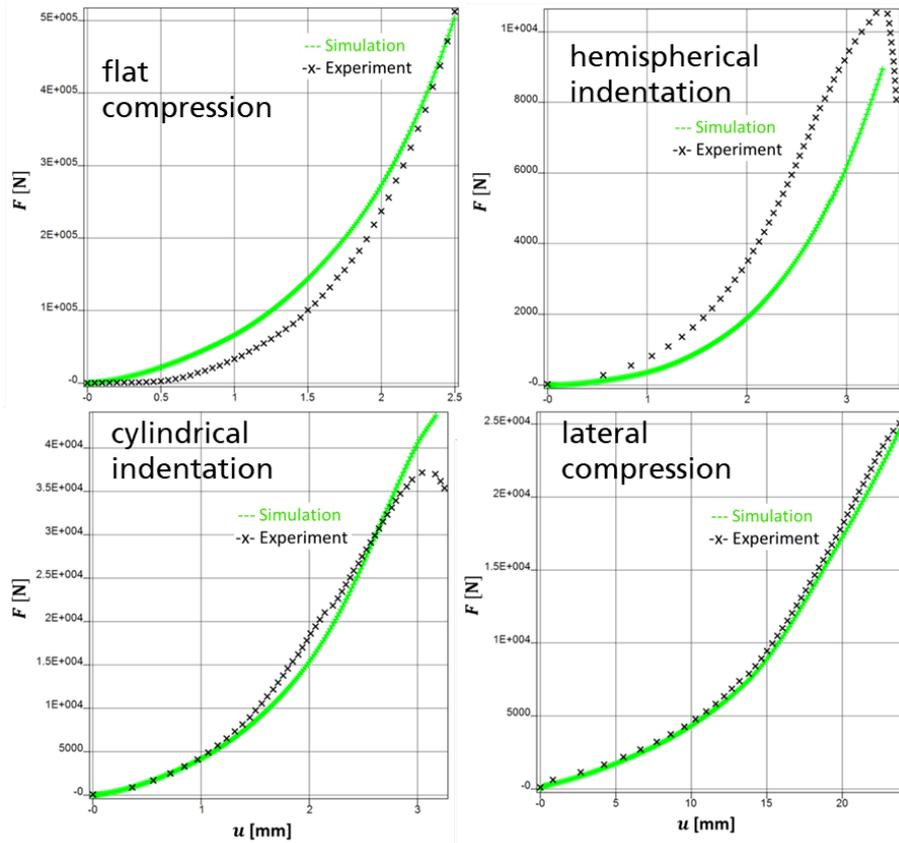
Fig.8: Comparison between simulation and experiments of force-displacement curves for different load cases by using `*MAT_MODIFIED_HONEYCOMB`
