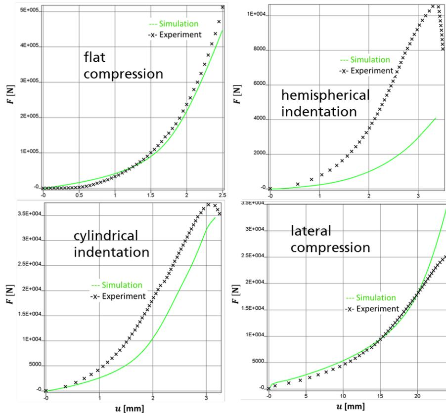
Fig.6: Comparison between simulation and experiments of force-displacement curves for different load cases by using **\*MAT\_CSCM**
