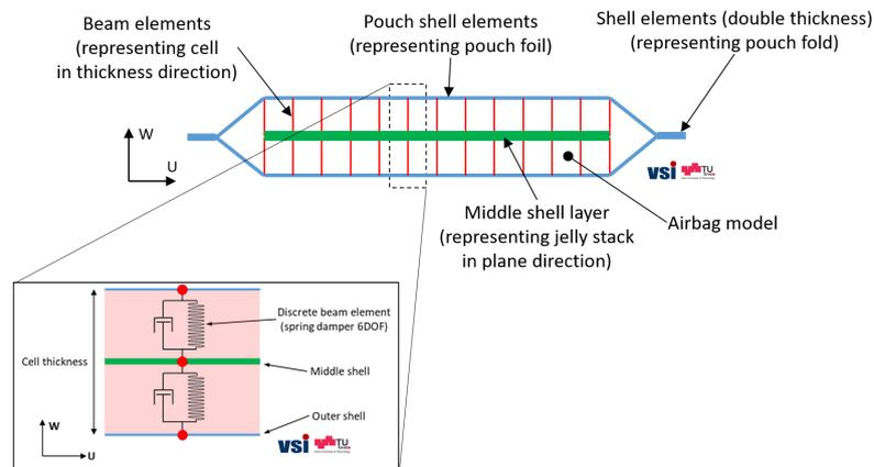
Fig.3: Concept of the Simplified Applicable Model
