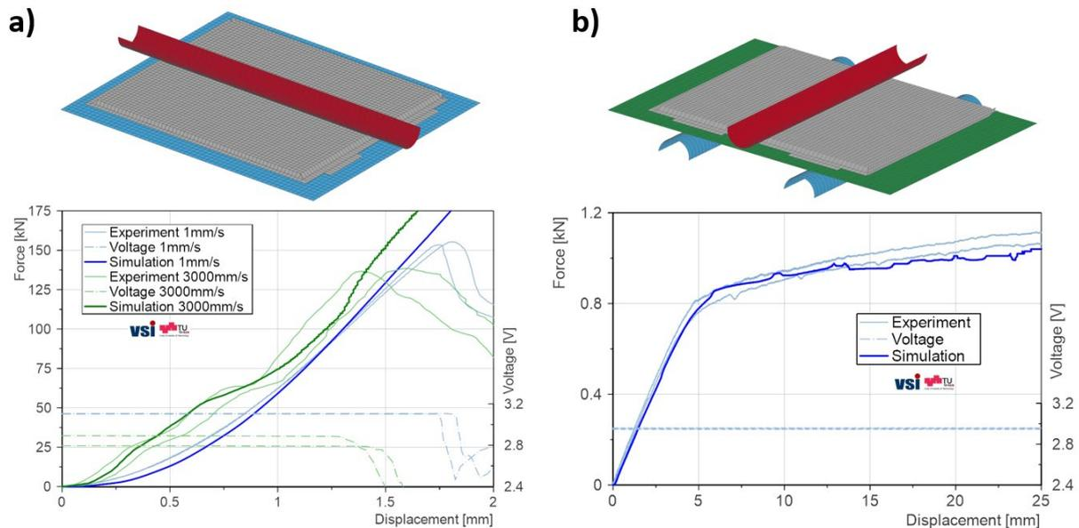
Fig.5: SAM results a) cylindrical indentation test - long side b) 3-Point bending test
