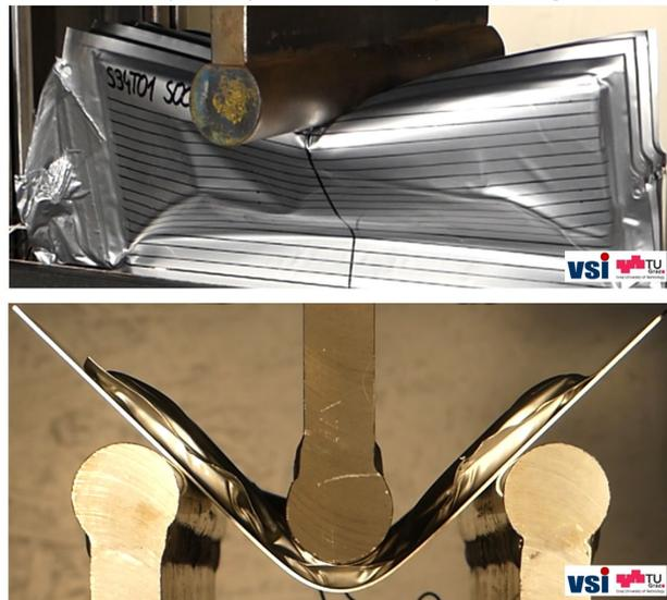
Fig.4: Top: Lateral indentation test Bottom: 3-Point bending test
