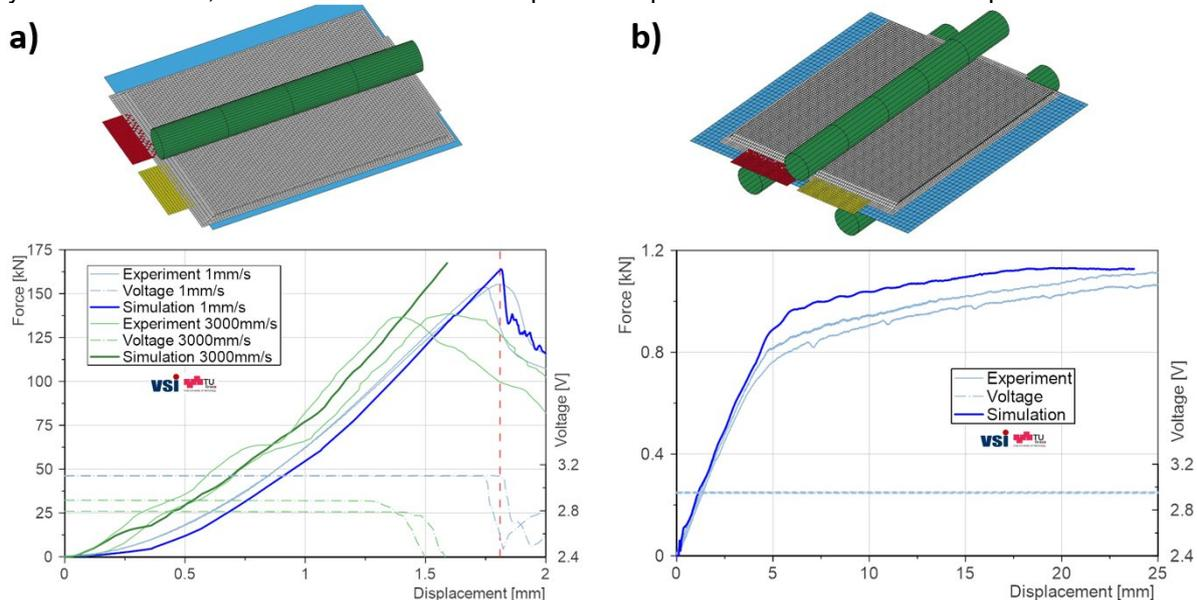
Fig.2: DLM results a: cylindrical indentation test - long side b: 3-Point bending test
