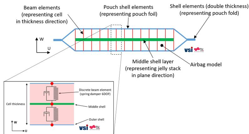
Fig.3: Concept of the Simplified Applicable Model
