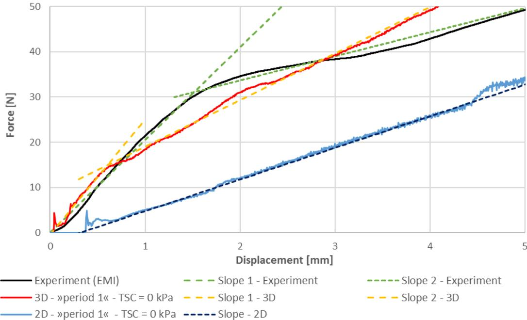
Fig. 7: Comparison of the slopes of the force curves for the first 5 mm of experiment, 2D and 3D model with »period 1«.
