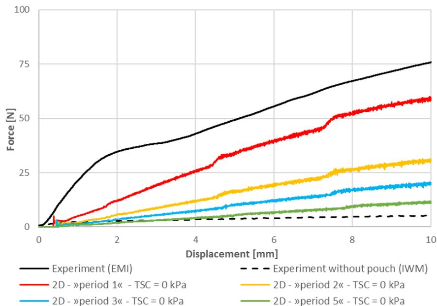
Fig. 6: Force-displacement curve simulated with different layer resolutions (2D) compared to cell bending experiments with (solid line) and without a pouch (dashed line).
