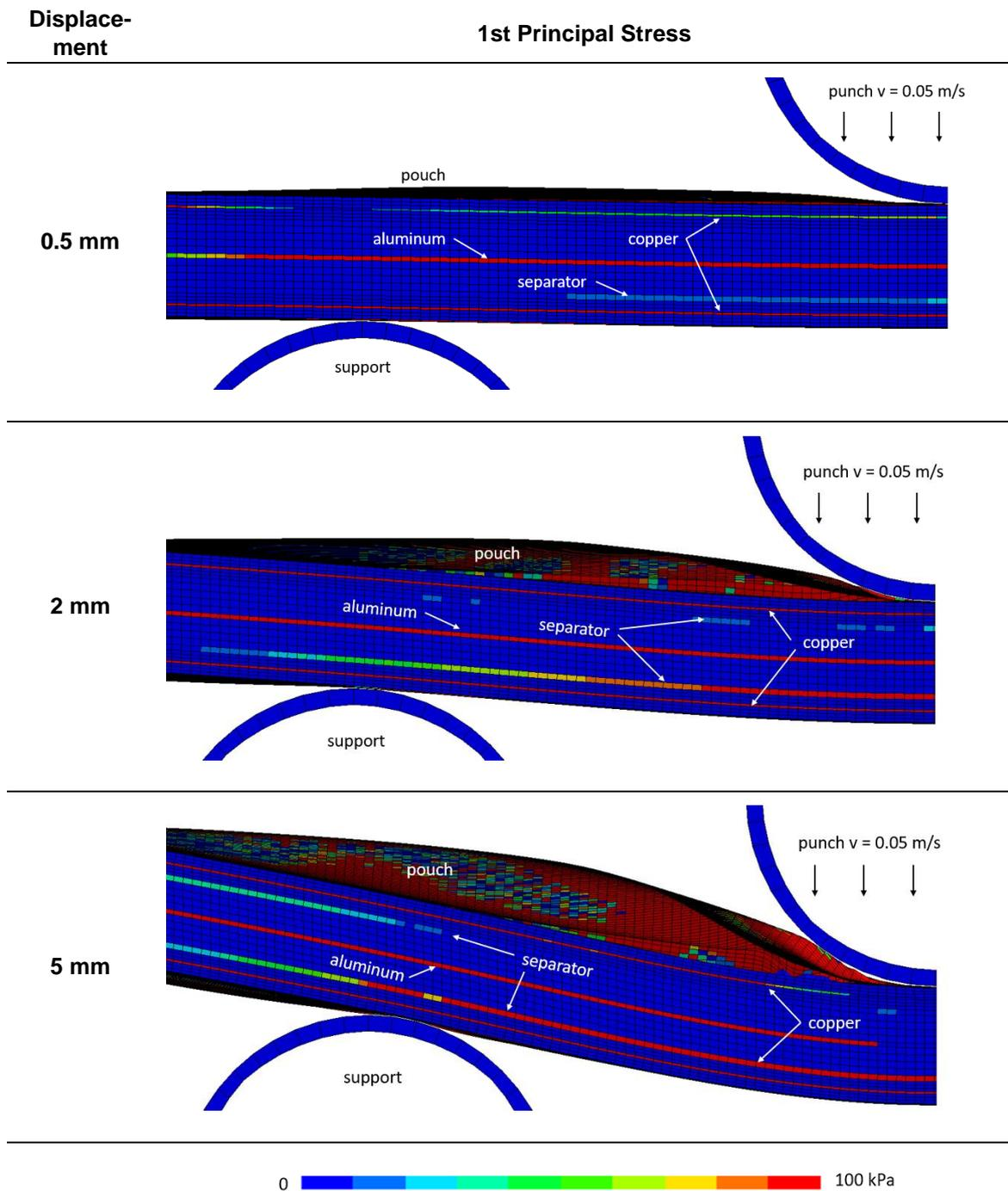
Fig. 5: First principal stress in the pouch cell for different displacements (cut-off at 0 and 100 kPa). Highest stresses occur in the stiff metal foils (aluminum and copper). Tensile stresses in these layers on top and bottom side of the cell.
