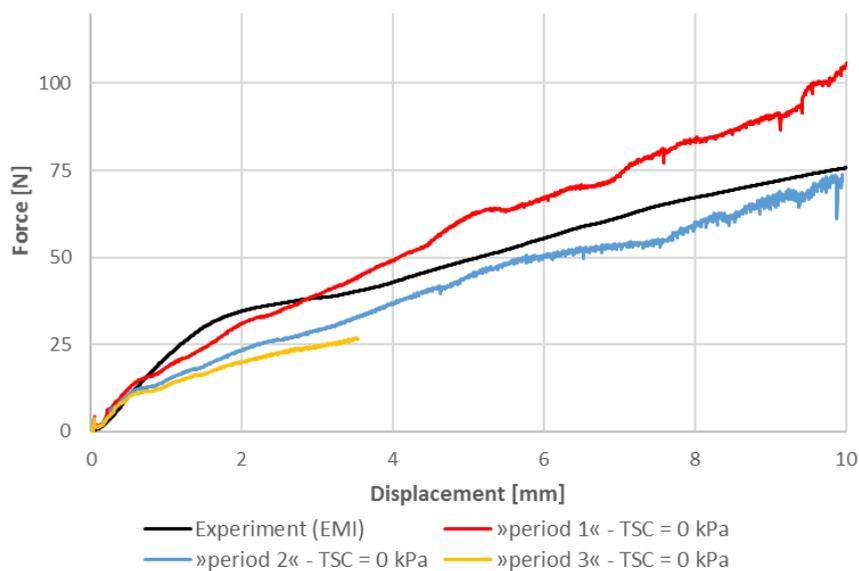
Fig. 4: Force-displacement curve simulated with different layer resolutions (3D) in comparison with the bending experiment.
