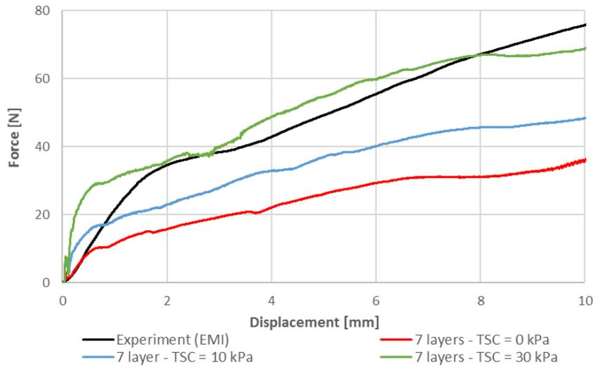
Fig. 10: Influence of the tensile stress cutoff (TSC) in *\*MAT\_CRUSHABLE\_FOAM* for the partly homogenized model with 7 metal layers.
