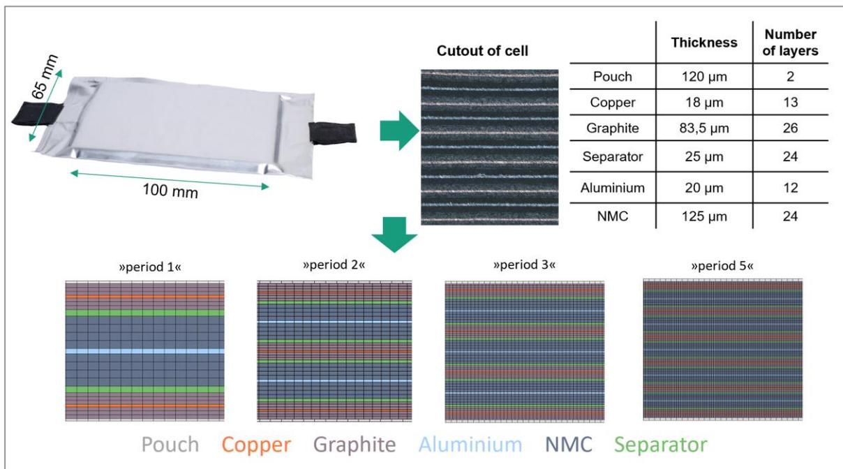
Fig. 1: Size and layers of the experimentally investigated pouch cell (top) as well as layer resolution in the simulation model (bottom).
