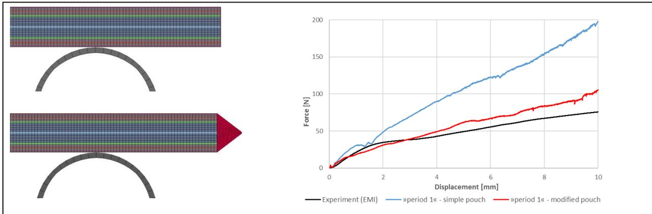
Fig. 3: Influence of the geometry of the pouch (colored in red on the left) on the simulated force-displacement curve (right). Closely surrounded box (left top) leads to higher forces compared to a more realistic approach (left bottom). Simulations with “period 1” resolution of the layered structure and  $TSC = 0$  kPa.
