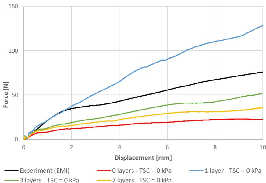
Fig. 9: Force-displacement curve simulated with a partly homogenized model for different numbers of internal metal layers.
