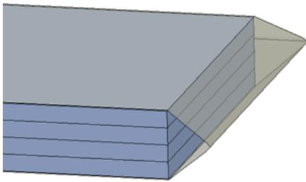
Fig. 8: Cutout of a partly homogenized model for a battery cell with a semi-transparent pouch.
