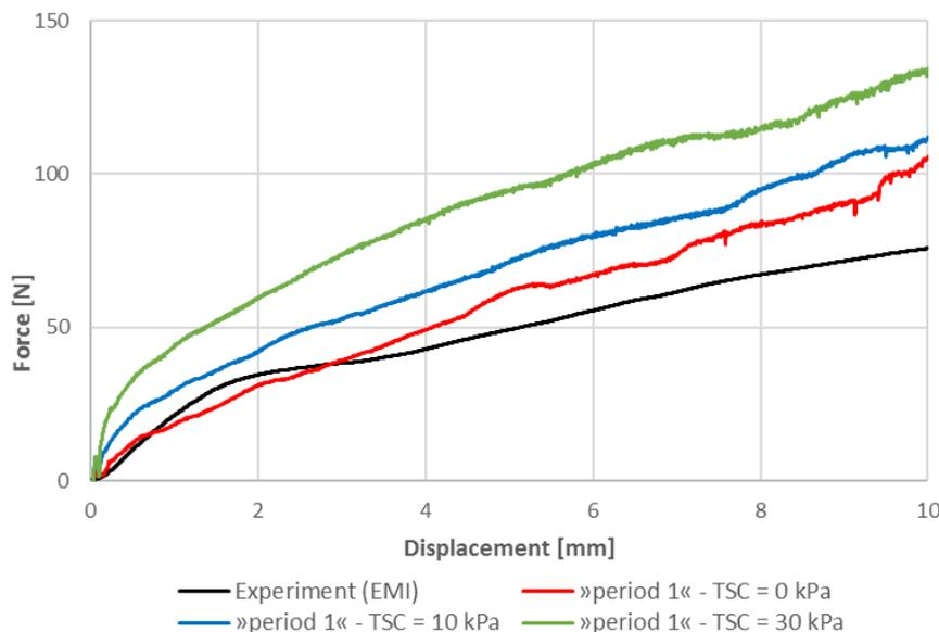
Fig. 2: Variation of the tensile stress cutoff (TSC) in the `*MAT_CRUSHABLE_FOAM` influences the force in the simulated bending-test. Simulations with »period 1« resolution of the layered structure.
