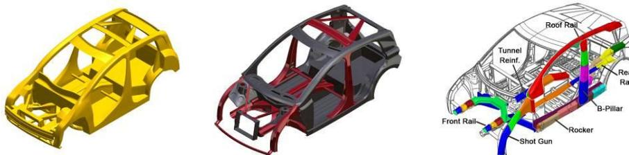
**Figure 13: LF3G optimization, reference body structure and structural sub-systems**
