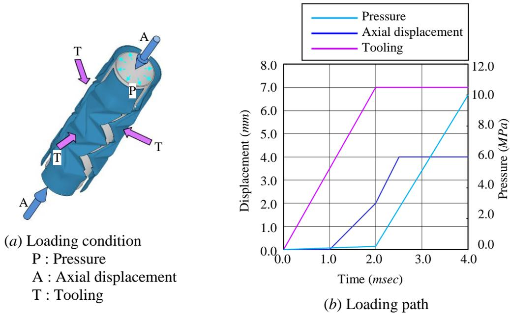
Fig.19 Loading condition and history for the hydroforming simulation
