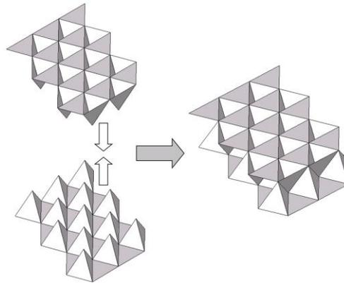
Fig.1 Combined truss core panel
