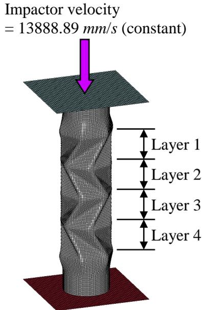
Fig.21 Crush simulation model
