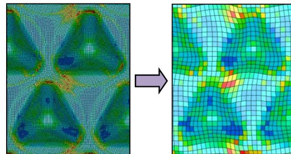
Fig.10 Mapping of stress, strain and thickness distribution from the fine mesh to the coarse mesh
