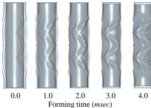
Fig.20 Deformation of the tube during the forming process
