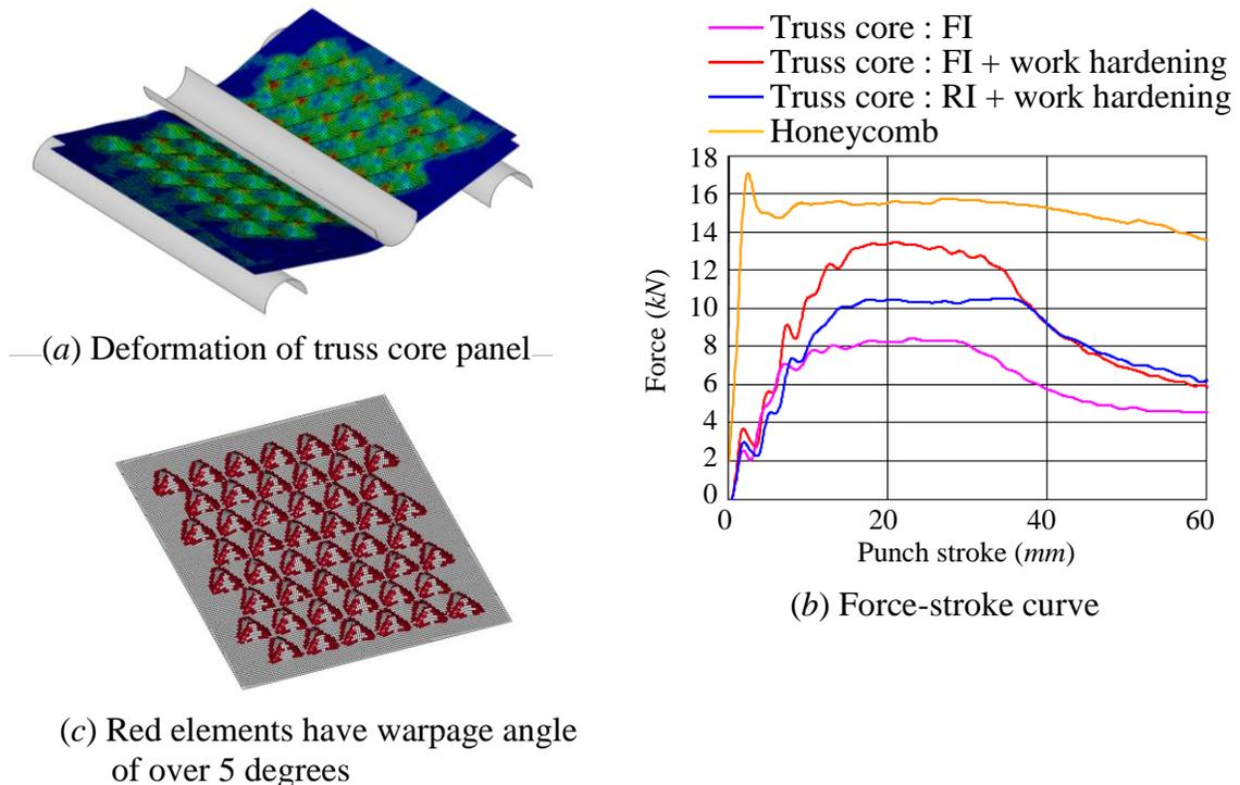
Fig.13 Results of three point bending simulation
