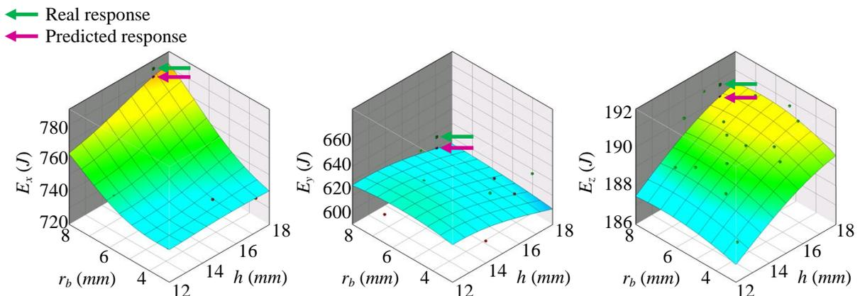
Fig. 16 Response surface of absorbed energy vs design variables  $h$  and  $r_b$  using RBF
