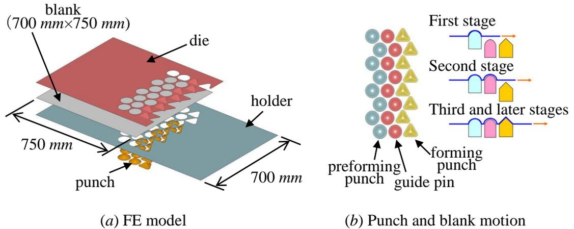
Fig.7 Multi-stage forming simulation
