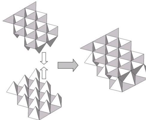
Fig.1 Combined truss core panel
