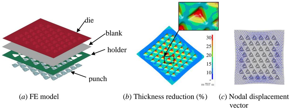
Fig.6 Single stage forming simulation
