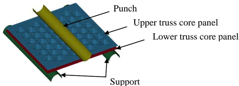
Fig.11 Truss core panel model configuration for three point bending simulation
