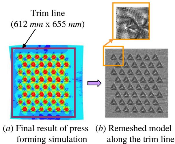
Fig.9 Trimmed model from formed geometry obtained by multi-stage press forming simulation
