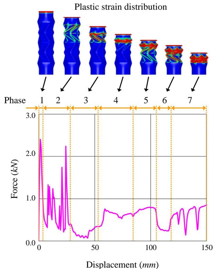
Fig.22 Force-displacement curve of the origami tube
