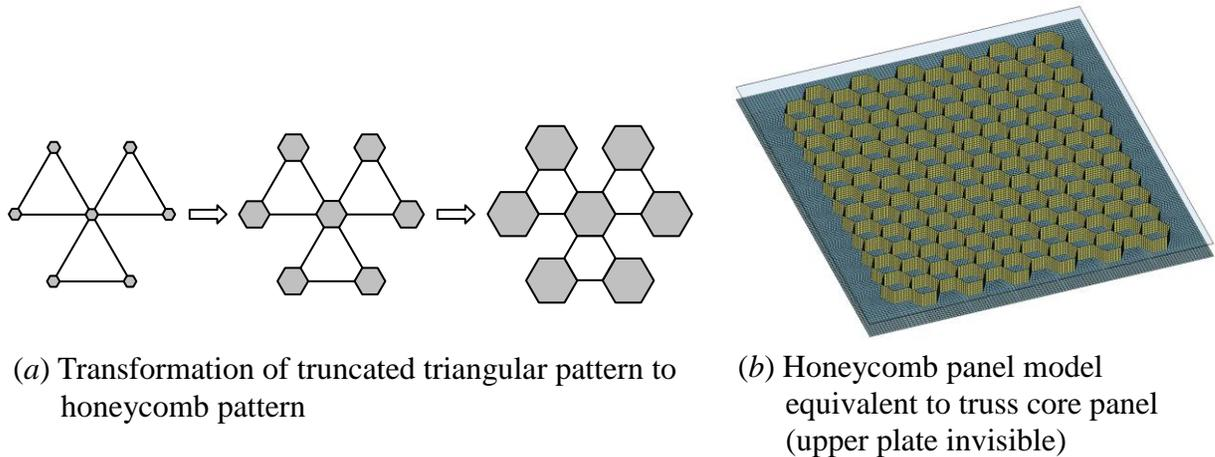
Fig.12 Honeycomb panel and truss core panel have a similarity
