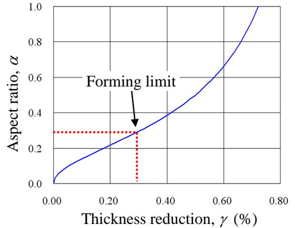
Fig.3 Aspect ratio ( $h/a$ ) versus thickness reduction
