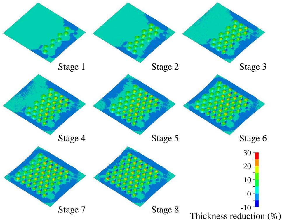
Fig.8 Forming sequence of multi-stage press forming of truss core panel
