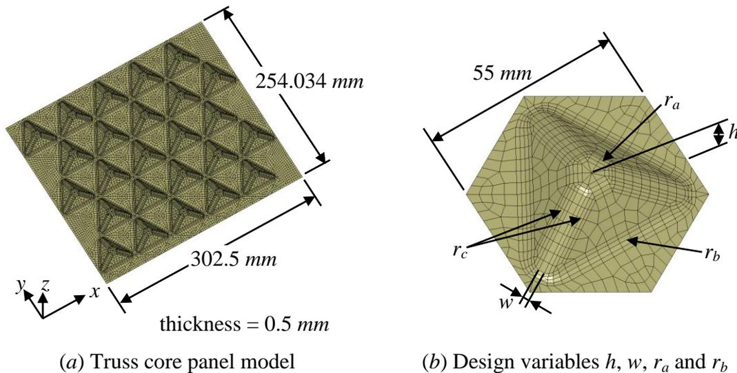
Fig. 15 Truss core panel FE model and design variables for shape optimization
