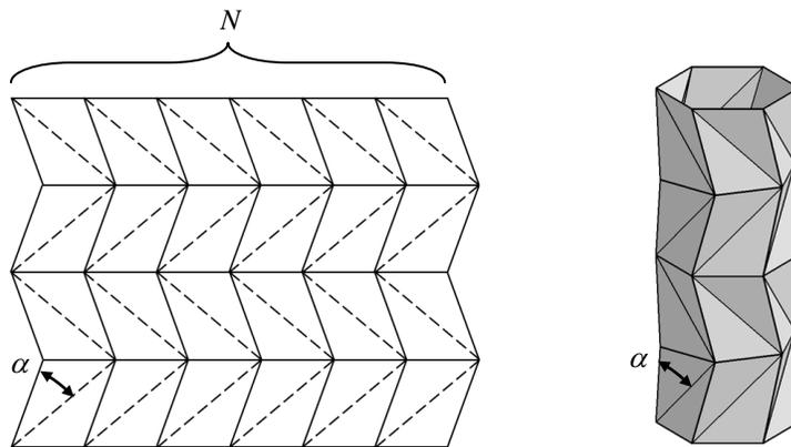
Fig.18 Development view and folded shape of reversed spiral origami tube. Solid lines in the development view are mountain fold and broken lines are valley fold.
