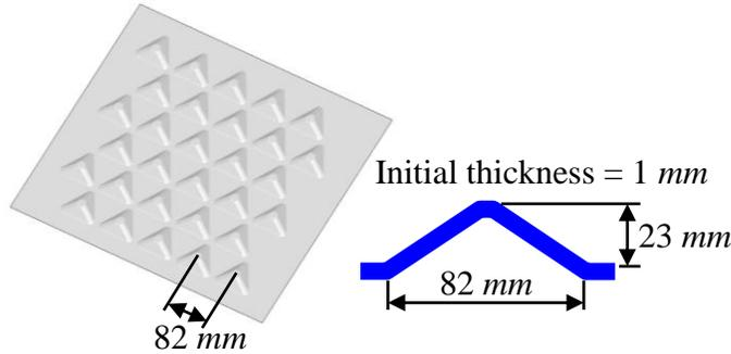
Fig.4 Geometry and dimensions of truss
