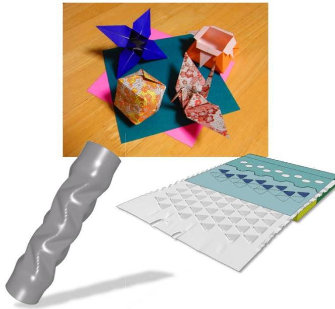
Examples of traditional origami (upper), truss core panel (right) and reversed spiral origami tube (left)
