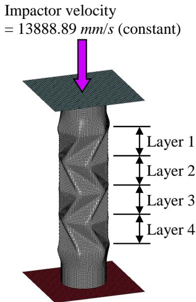
Fig.21 Crush simulation model
