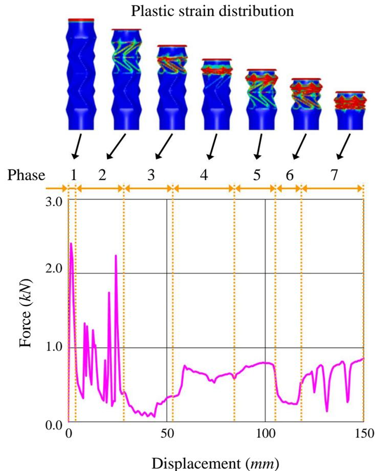
Fig.22 Force-displacement curve of the origami tube
