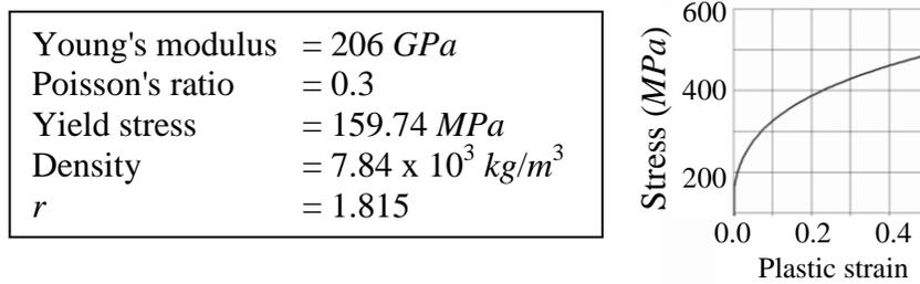
Fig.5 Material properties and stress-strain curve
