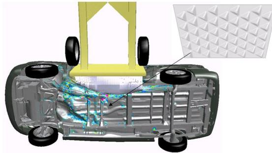
Fig.14 Candidate parts to adopt truss core panel (FE model courtesy of NCAC)[4]
