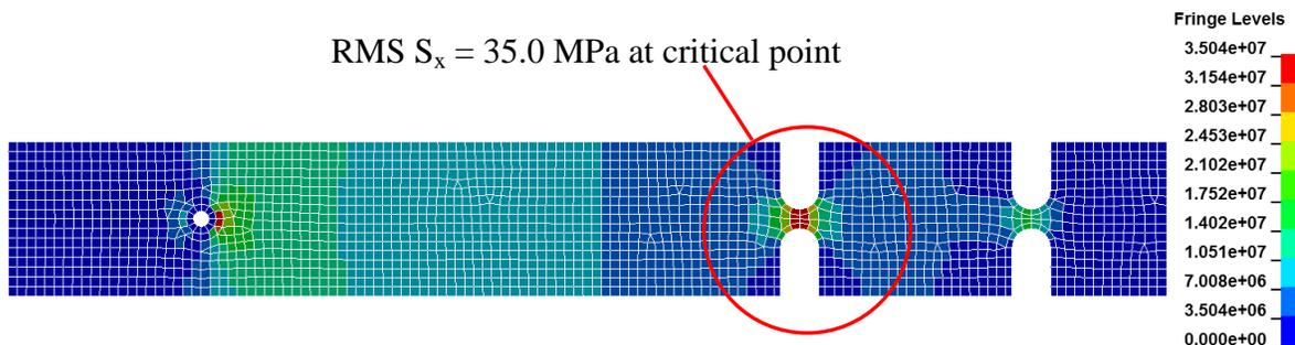
Figure 9 – RMS of  $S_x$  stress in the local element axis
