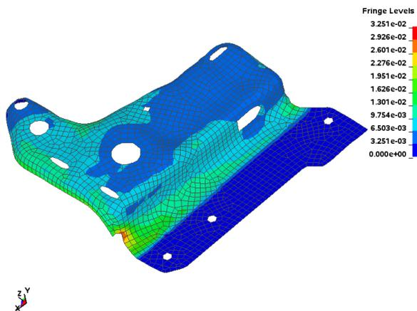
Figure 3 – RMS of Von-Mises stress
