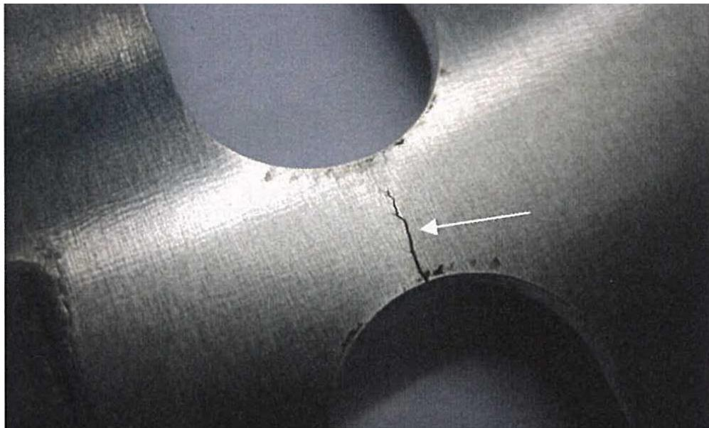
Figure 13 - Failure at the notched point in experiment
