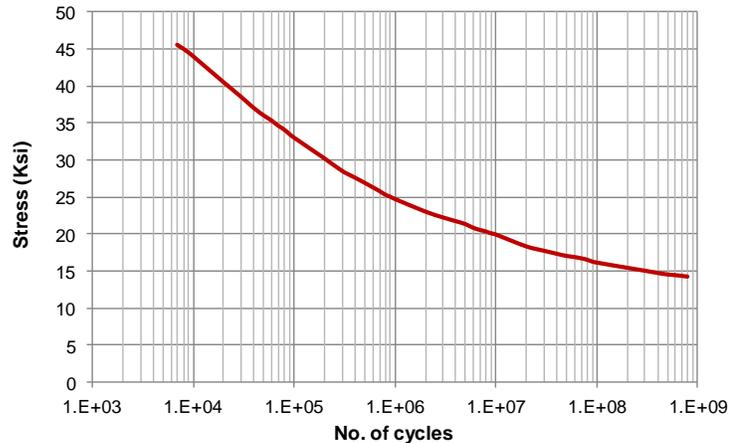
Figure 2 – S-N fatigue curve
