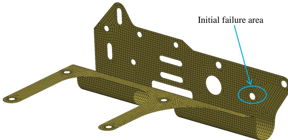
Figure 15 – broken support
