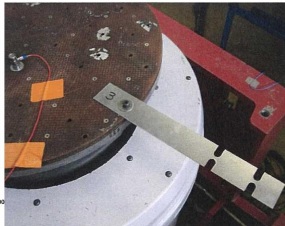
**Figure 7 – beam on the shaker table**
