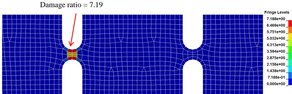
Figure 12 - Cumulative damage ratio by Steinberg's method
