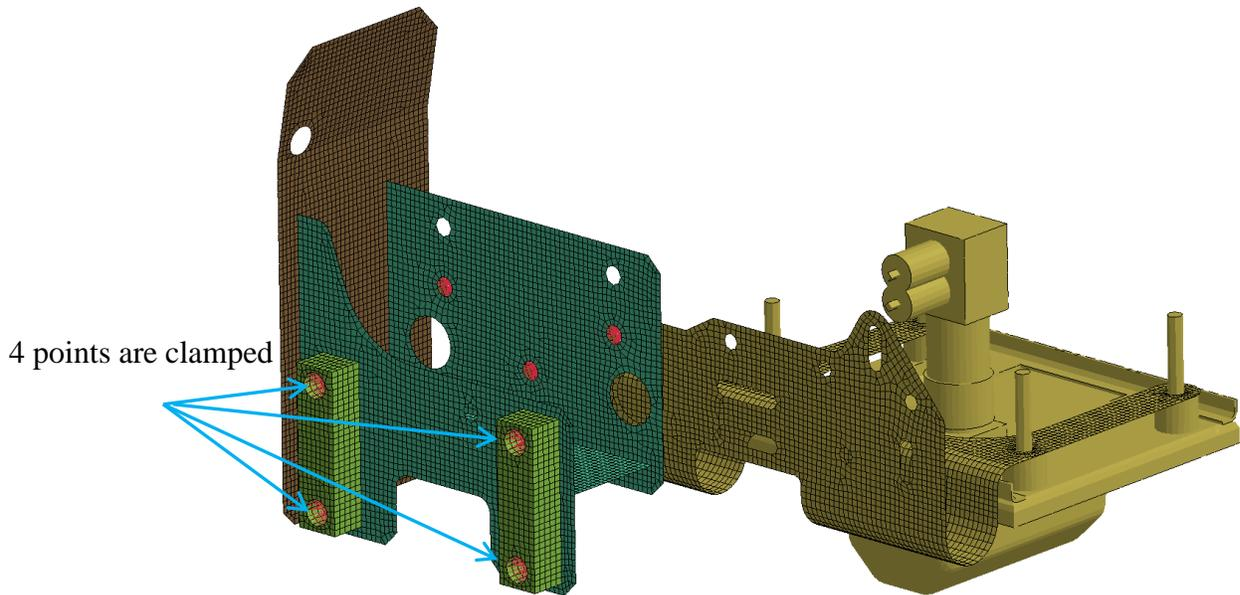
Figure 14 (b) – back view of the support antenna model
