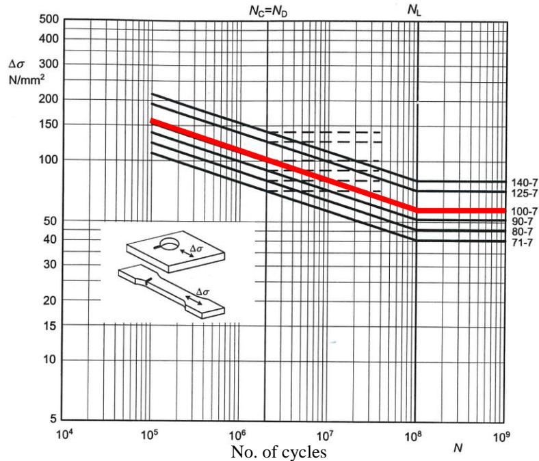
Figure 8 – S-N fatigue curve used for the notched aluminum beam
