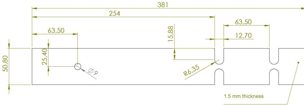
**Figure 5 – aluminum beam using for the shaker table experiment**
