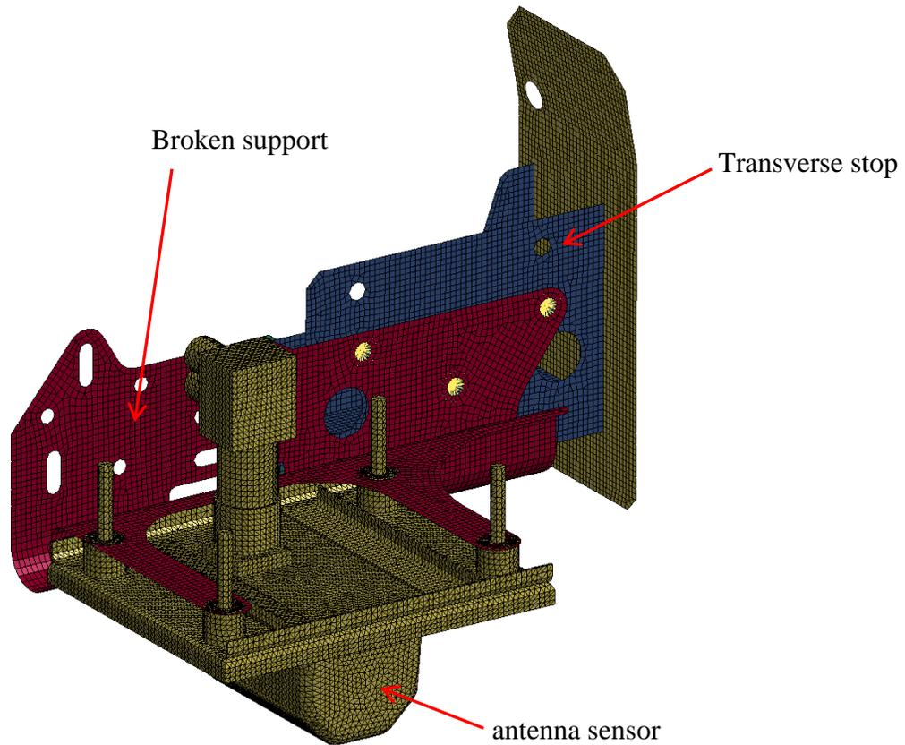
Figure 14 (a) – global view of support antenna model
