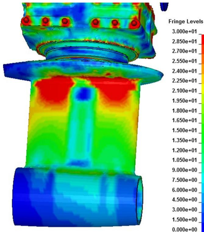
Figure 10 – 3D LS-DYNA simulation results - Von Mises stress results on POD principal parts
