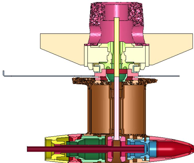
Figure 3 – Preliminary LS-DYNA 3D model – Internal transmission system elements
