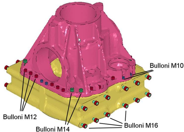
Figure 6 – Connection bolts models
