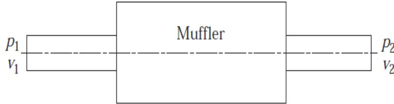
Figure 2. The four-pole method
