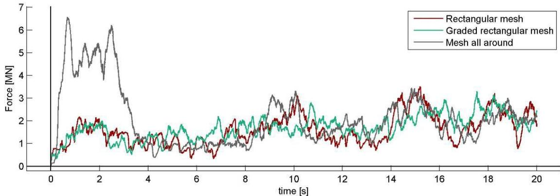
Figure 7: Force levels obtained with different meshes and also one where the ice encloses the lighthouse (mesh all around).
