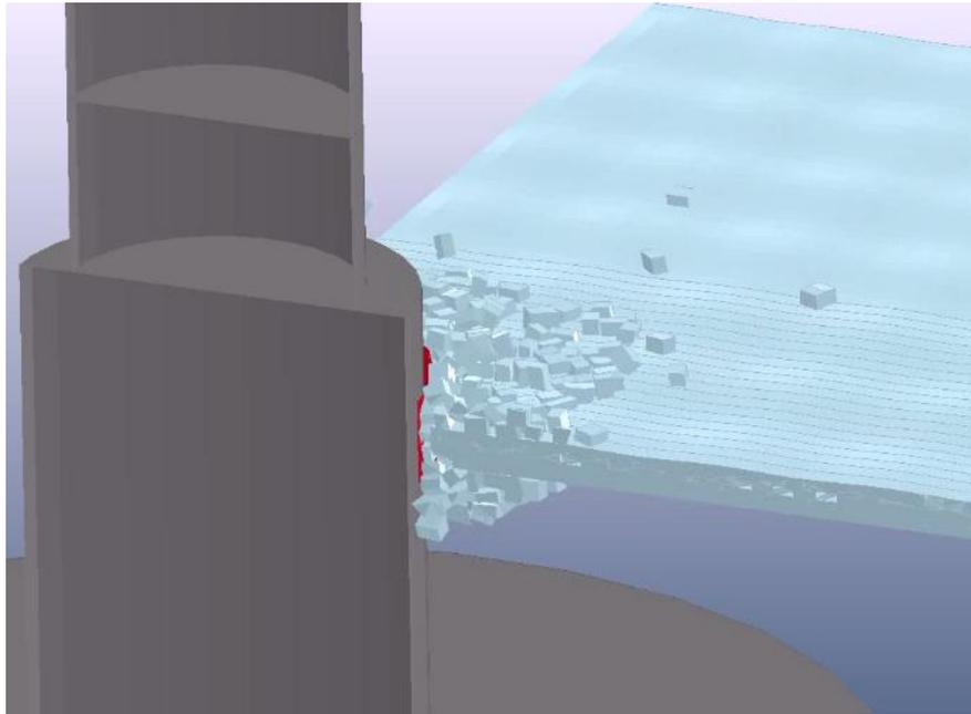
Figure 6: Typical situation in front of lighthouse in the simulation. Crushed ice piles up in front of lighthouse above and beneath the ice sheet. This is similar to what was observed in the field.
