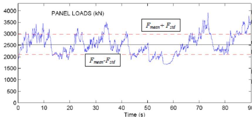
Figure 8: Measured total force applied on the lighthouse during a continuous crushing event.
