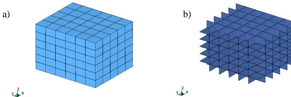
Figure 2: A block of ice built up by elastic hexahedral elements is shown to the left. To the right the cohesive elements that hold together the hexahedral elements in the block are shown.
