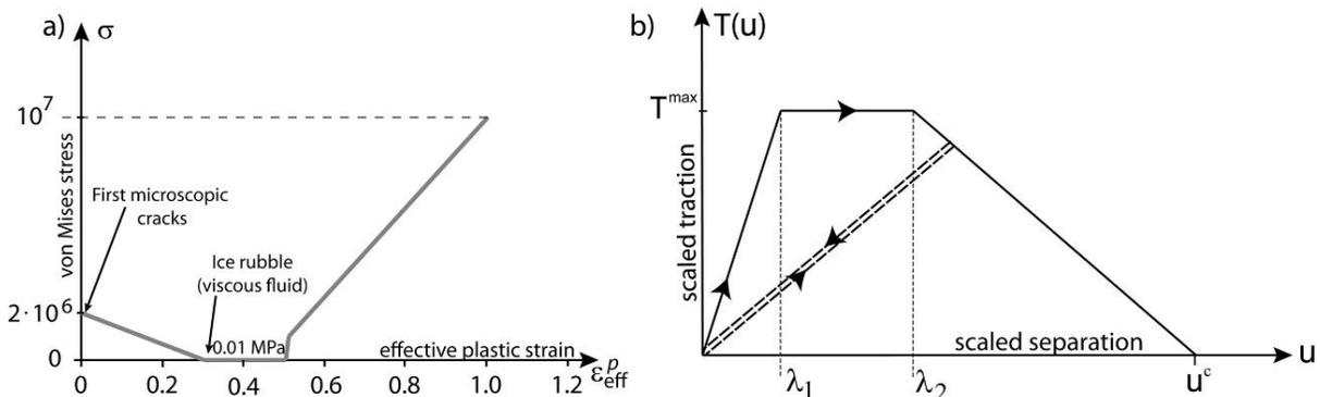
Figure 1: a) Schematic of the yield curve of the ice material, with von Mises stress plotted against effective plastic strain; and b) Non-reversible traction separation law for the ice cohesive elements.
