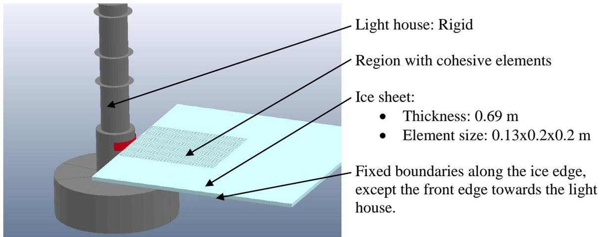
Figure 4. Model with light house and ice sheet. The force measurement panels are shown in red.
