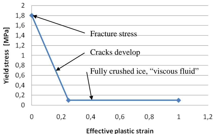
Figure 3: Schematic hardening curve for ice elements with a homogenized crack model.
