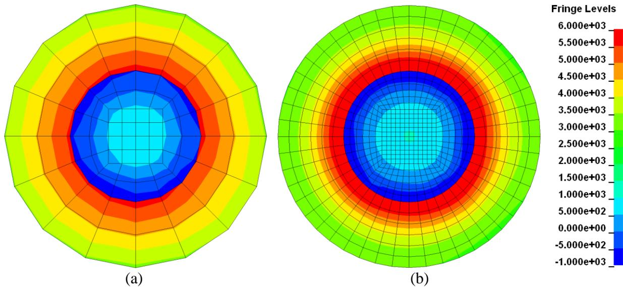
Figure 14. Contours of first principal stress in (a) the coarse mesh and (b) the refined mesh at the end of the dynamic relaxation phase using `NODES_TO_SURFACE_SMOOTH` in conjunction with a thermal load.
