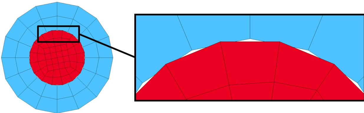
Figure 9. Incompatible mesh on the journal bearing and shaft can cause locking with NODE\_TO\_SURFACE contact.
