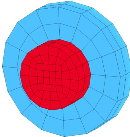
Figure 3. Mapped hexahedral mesh used in the journal bearing example problem.
