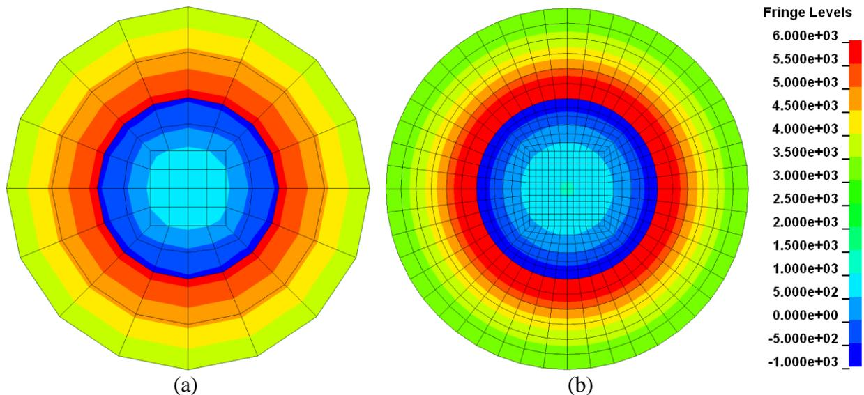
Figure 13. Contours of first principal stress in (a) the coarse mesh and (b) the refined mesh at the end of the dynamic relaxation phase using NODES\_TO\_SURFACE\_INTERFERENCE.
