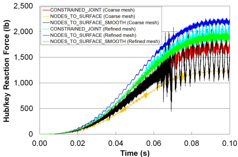
Figure 17. Reaction force on the key for various contact options.
