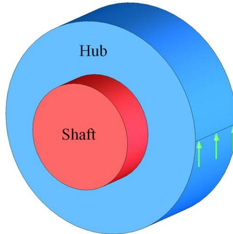
Figure 1. Example problem of an 8-inch diameter hub mounted on a 4-inch diameter shaft with a tangentially applied load.
