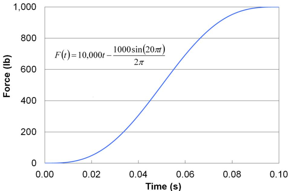
Figure 2. The magnitude of the applied load as a function of time.
