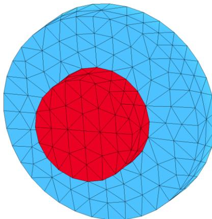
Figure 7. Tetrahedral mesh used in the journal bearing example problem.
