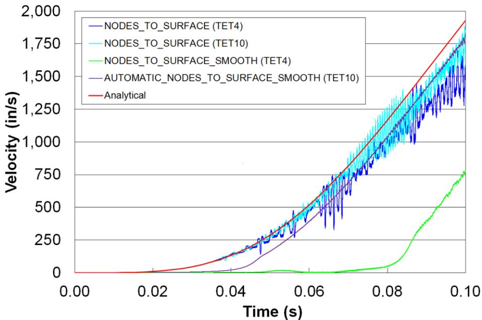
Figure 8. Velocity of the outside diameter of the journal bearing for an automatically generated tetrahedral mesh.
