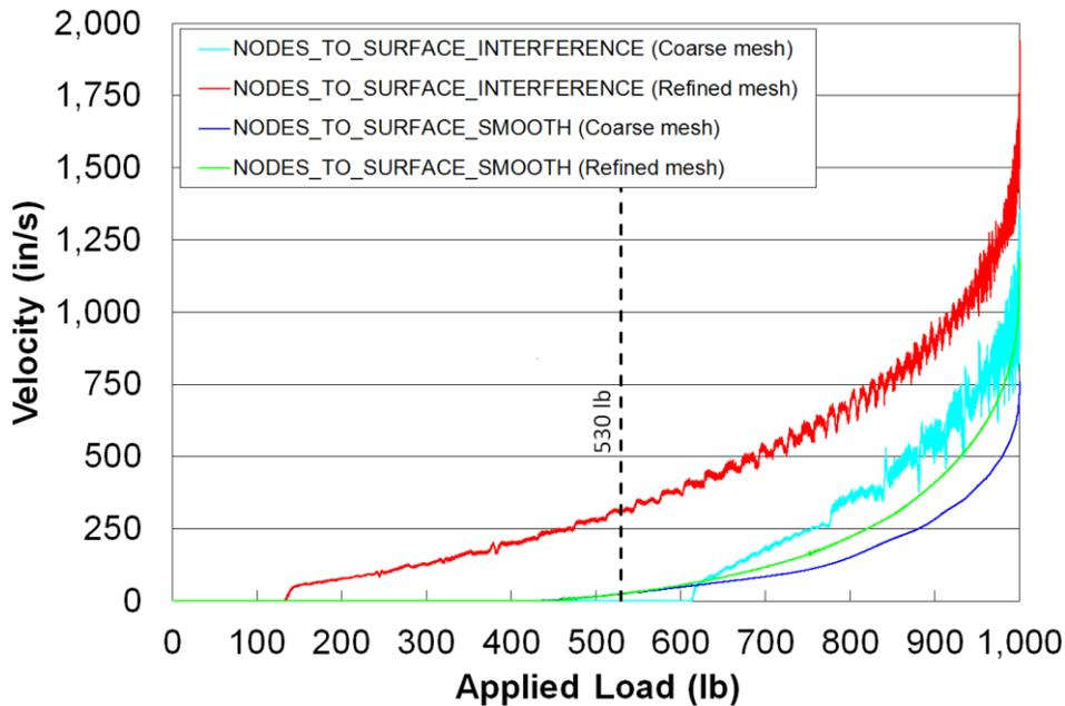
Figure 15. Velocity of the outside diameter of the press fit hub for various penalty-based contacts and element sizes.
