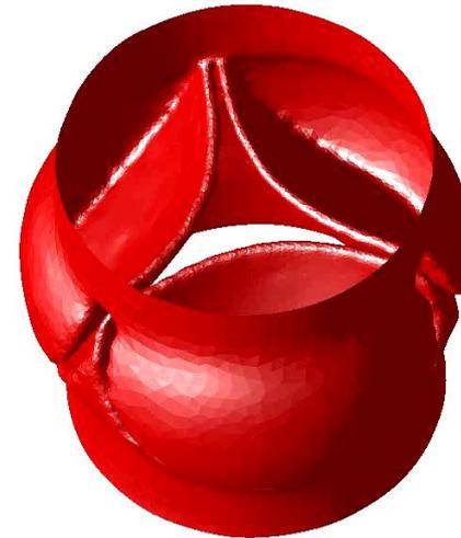
Simulation of synthetic heart valve. Density of Solid and Fluid (blood) very close: complex FSI strong coupling case.
