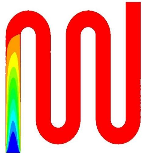
Steady state fluid temperature (cut plane through the section)
