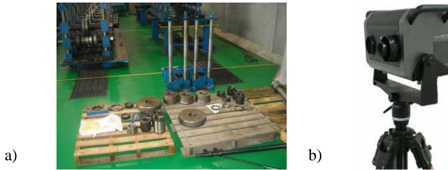
Figure 2. (a) Disassembled stand (b) and the Konica RANGE 7 equipment utilized for the optical measurements.
