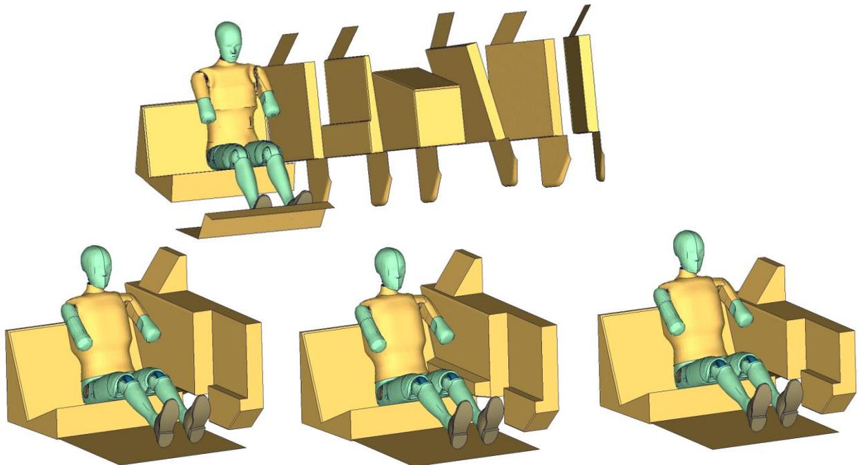
Figure 13: ES-2 / ES-2re validation sled tests.
