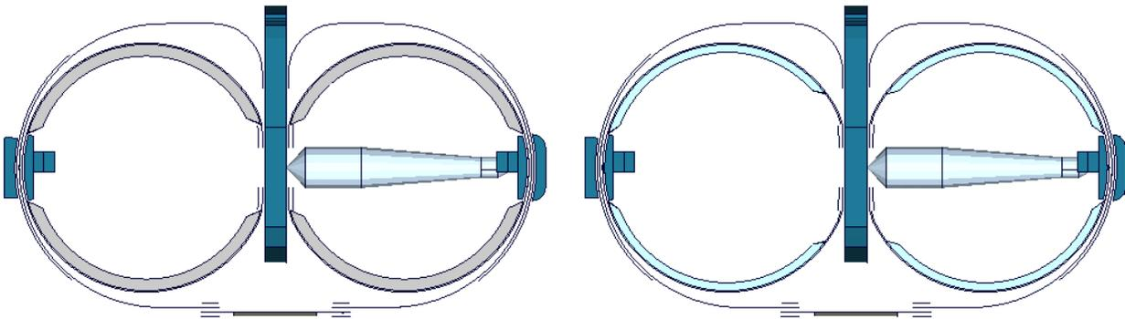
**Figure 21:** WorldSID 50% shoulder rib; comparison of old “gray” damping material (left) and new “blue” damping material (right).
