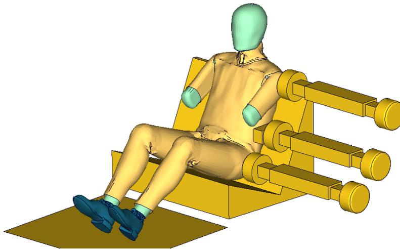
**Figure 10:** WorldSID 50% pendulum test target points.
