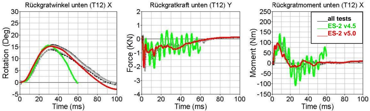
**Figure 18:** Lumbar spine bending test (left: T12 rotation; middle: T12 y-force; right: T12 x-moment).
