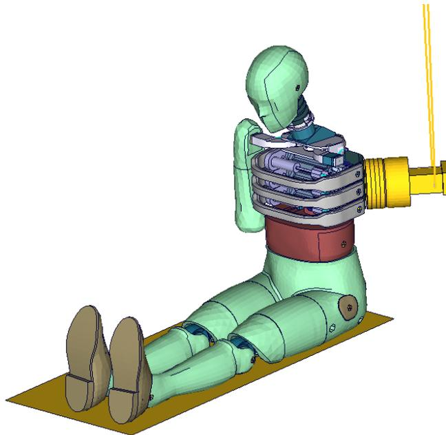
**Figure 11:** ES-2re additional pendulum test for rib extension validation.
