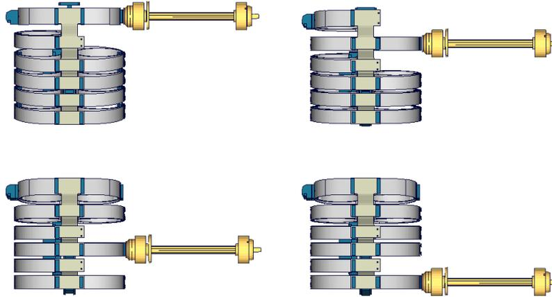
**Figure 22:** Different lateral impact locations of WorldSID 50% ribs. Top left: shoulder rib, top right: 1<sup>st</sup> thorax rib, bottom left: 3<sup>rd</sup> thorax rib, bottom right: 2<sup>nd</sup> abdomen rib.
