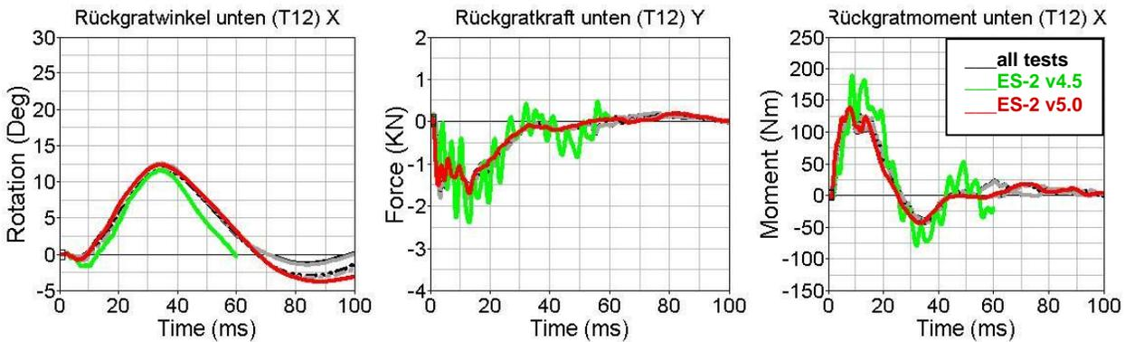
**Figure 19:** Lumbar spine shear test (left: T12 rotation; middle: T12 y-force; right: T12 x-moment).
