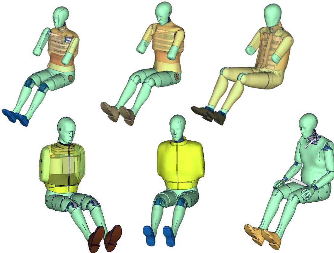
**Figure 1:** FAT and PDB dummy models of DYNAmore.
