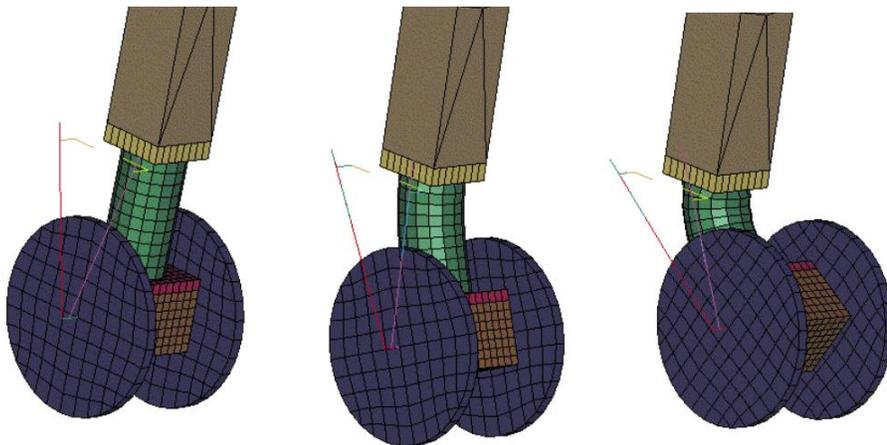
**Figure 15:** Deformation of lumbar spine (green) in calibration tests at different times.
