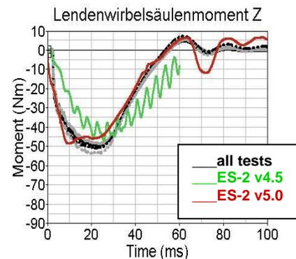
**Figure 20:** Lumbar spine torsion test (T12 Z-moment).
