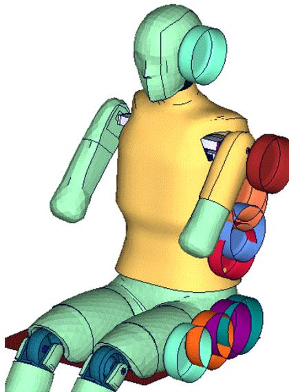
**Figure 9:** ES-2 pendulum test target points.
