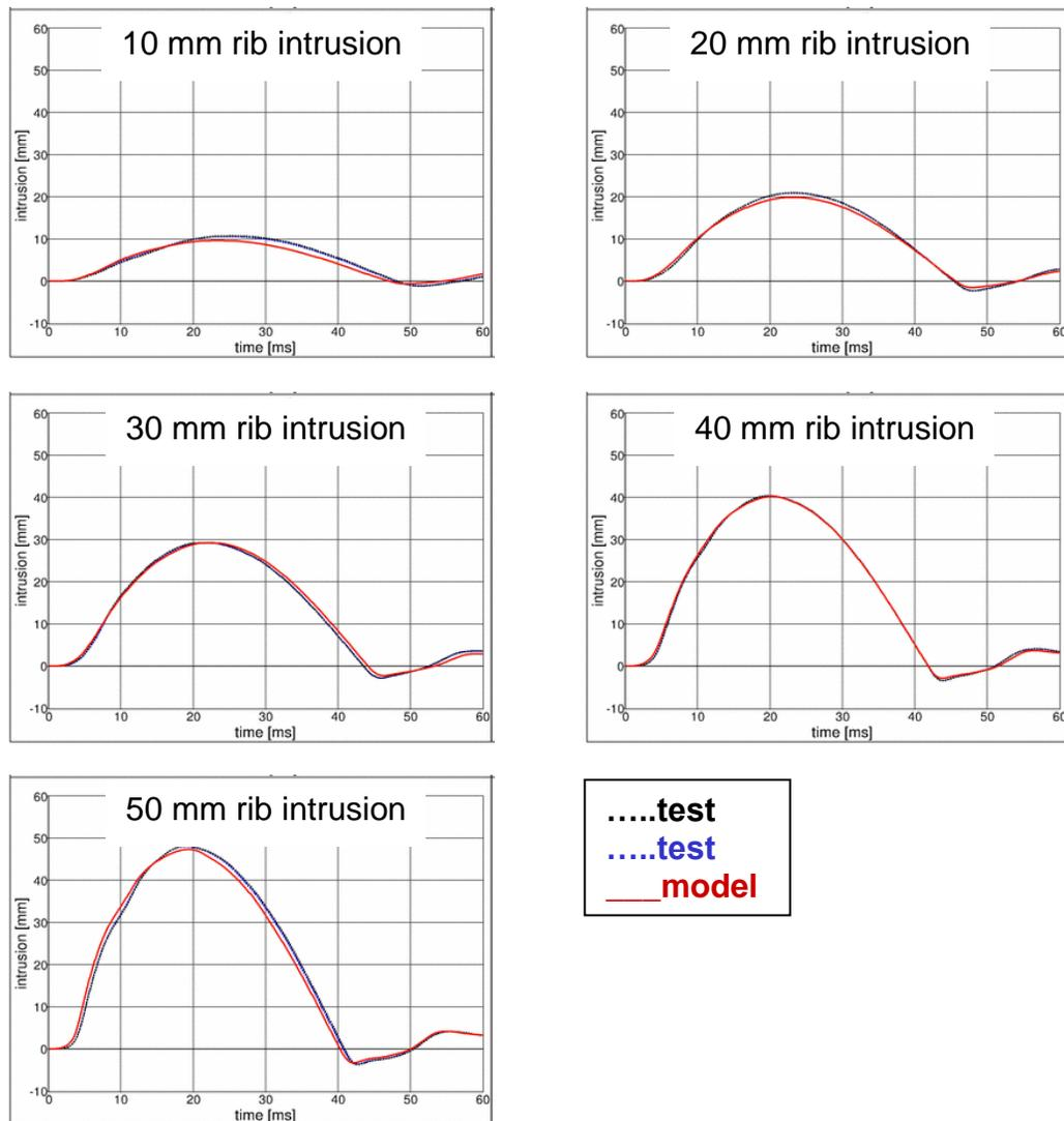
**Figure 6:** Rib deflection results of ES-2 for different pendulum speeds.
