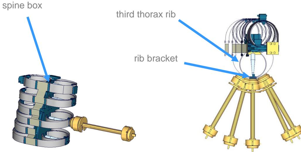
Figure 7: WorldSID 50% rib design and various pendulum angles.
