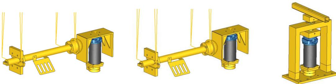
**Figure 17:** New component tests for ES-2 lumbar spine (left: bending; middle: shear; right: torsion).
