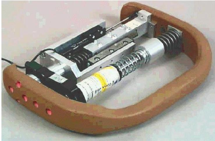
**Figure 4:** Rib assembly of ES-2.
