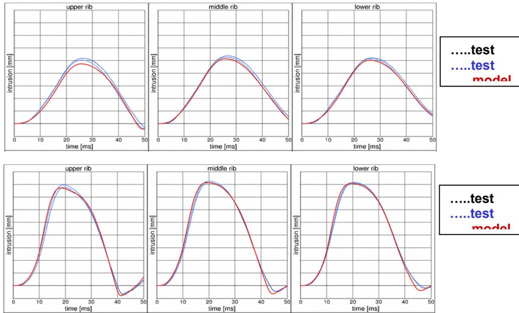
Figure 12: Results of ES-2re rib extension pendulum test.
