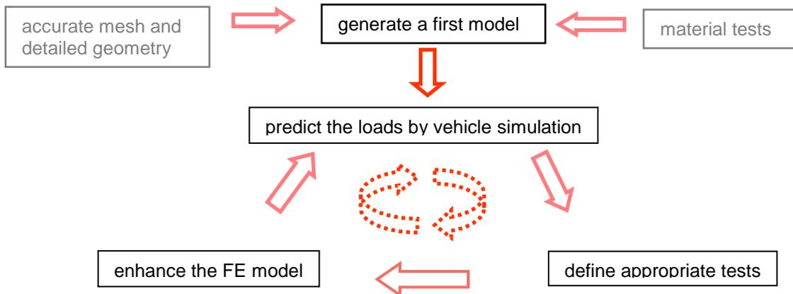
**Figure 16:** Validation process of FAT and PDB dummy models.
