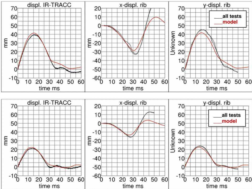
Figure 8: Third thorax rib component test of WorldSID 50%.
