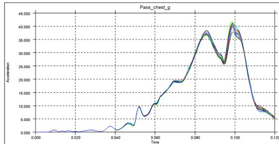
Figure 9. Dummy chest accelerations from thirty improved models
