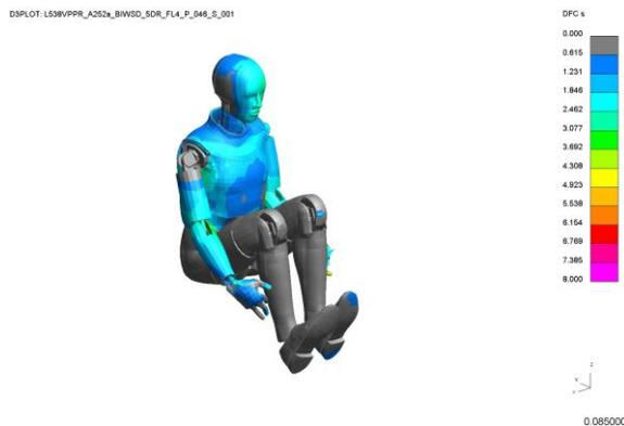
Figure 6. Dispersion in nodal coordinates of dummy at 85ms
