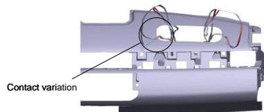
Figure 2. Airbag contact variability at 23ms
