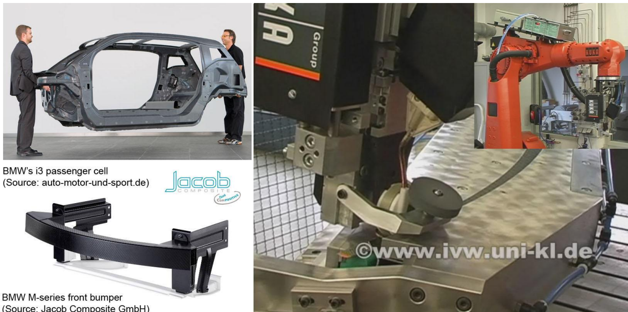
Figure 1: Examples of automotive components that could or have already benefitted from induction welding (left). Induction welding Kuka robot at the Institute für Verbundwerkstoffe (right) joining the two thermoformed components of the BMW M-series front bumper beam
