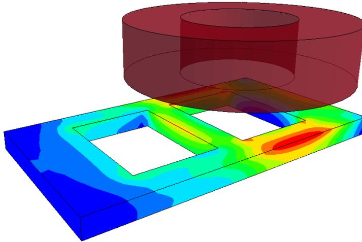
Figure 8 Uniform current in Multiturn Coil inducing current in a plaque
