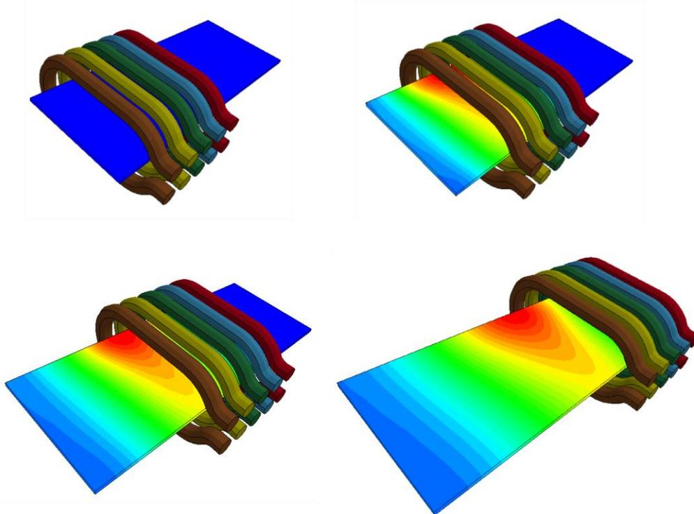
Figure 3 Temperature fringes of an inductive heating example
