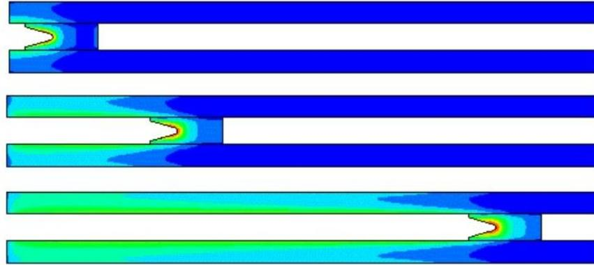
Figure 5 Rail gun model : Current flowing between rails and projectile generates magnetic field (fringes) and Lorentz forces that accelerate the projectile
