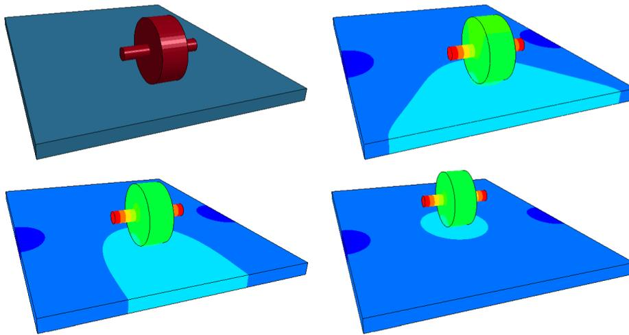
Figure 4 Scalar Potential fringes of conductive wheel in contact with conductive plate
