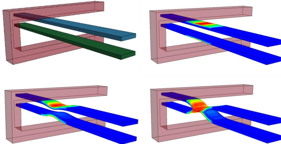
Figure 6 Current density fringes of a Welding test case between two metal pieces. Conducted in collaboration with the University of Waterloo, Canada
