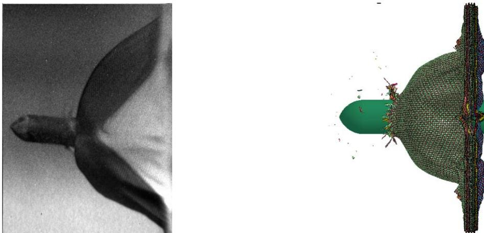
Fig. 8 Results of a ballistic test with 4-layered composite.
