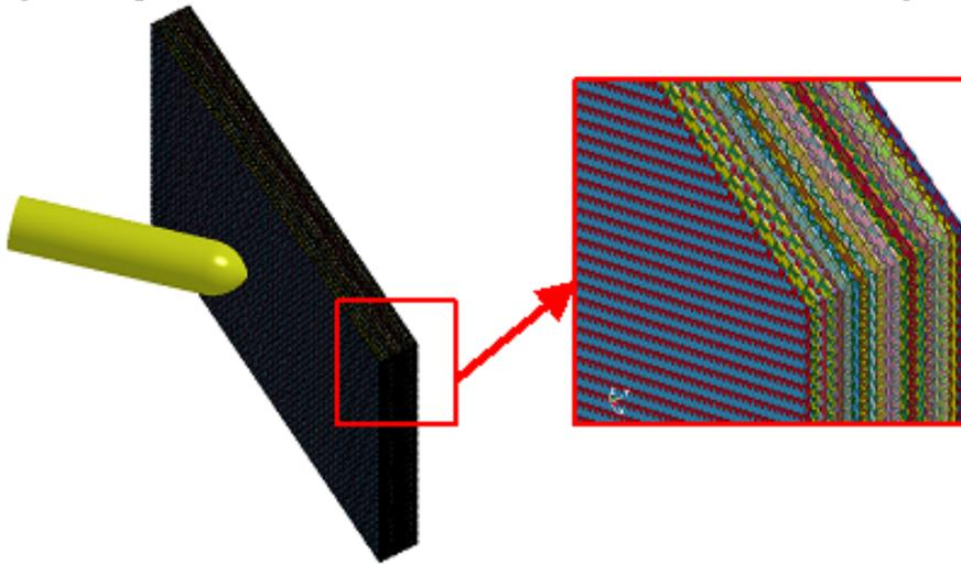
Fig. 7 Full-scale FE model for ballistic angular test with 20-layer package.
