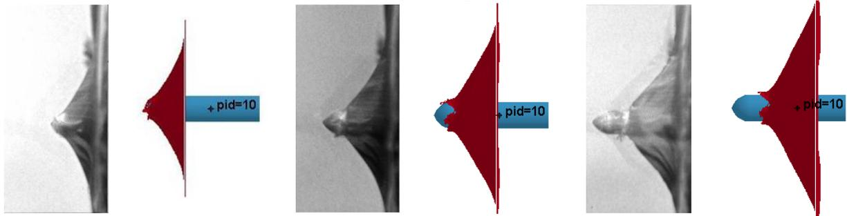
Fig. 11. 4-layer composite. Initial velocity is 266 mps.
