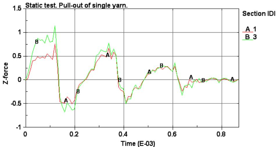
Fig. 6 Friction curve obtained in the simulation of the pull out tests.
