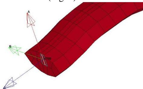
Fig. 3 FE model of an individual yarn.
