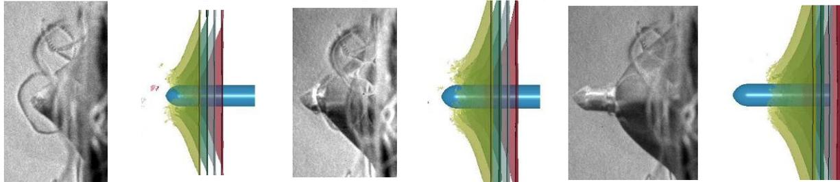
Fig. 12. 40-layer composite. Impact velocity is 380 mps.
