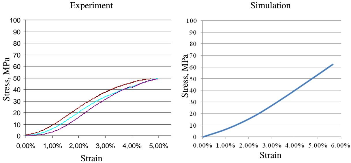
Fig. 5 Stress-strain curves in tensile tests with 8-layer package.
