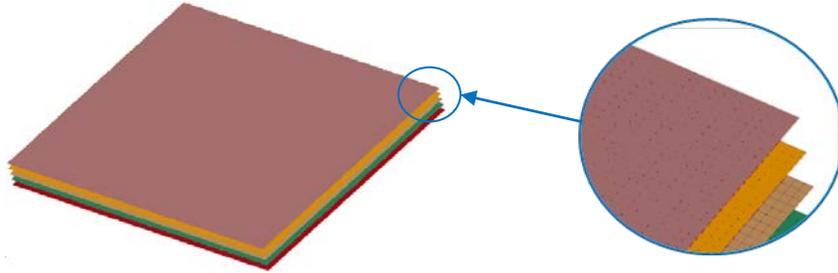
Fig. 1 FE reduced model of a multilayered woven composite.
