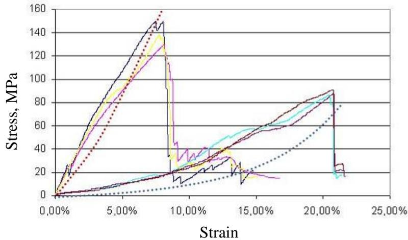
Fig. 4 Stress-strain curve in tensile tests with a single-layer fiber.
