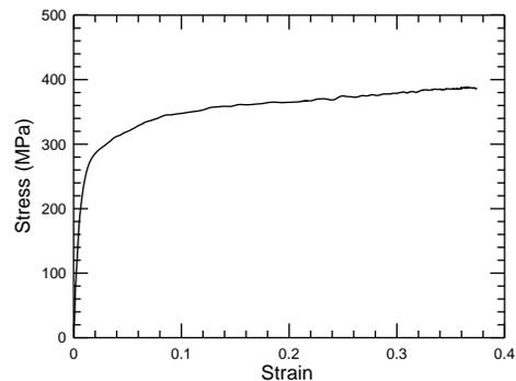
Fig. 12 Axial strain measured with DIC in a compression test. Fig. 13 Stress strain curve for 6061-T6 aluminum.
