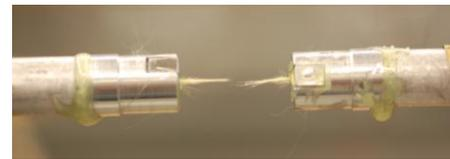
Fig. 6 Kevlar yarn following a tensile SHB test.
