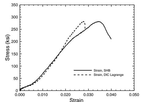
Fig. 8 Tensile stress strain curve for Kevlar cloth.
