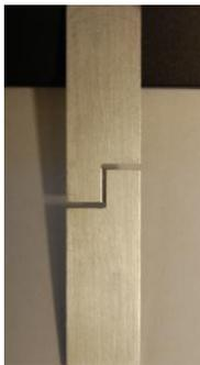
Fig. 2 Shear sheet metal specimen.
