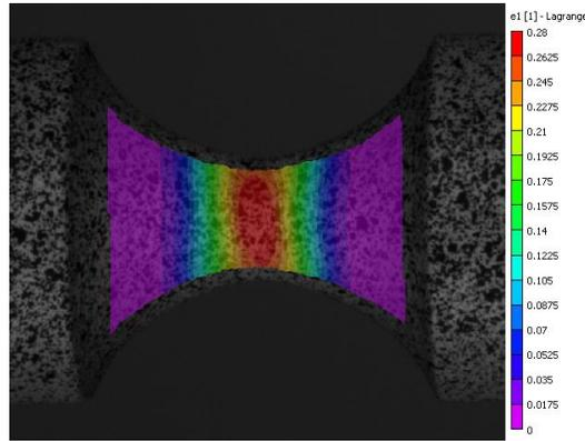
Fig. 1 DIC strains in tensile test of notched round specimen.
