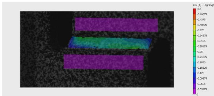
Fig. 3 DIC shear strains in sheet metal specimen.
