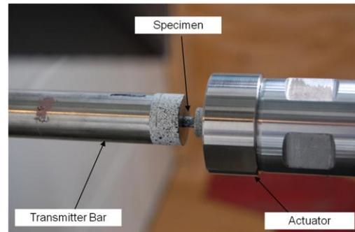
Fig. 11 Intermediate strain rate apparatus.
