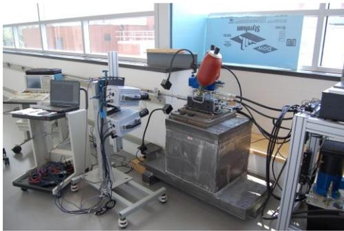
Fig. 10 Intermediate strain rate apparatus.
