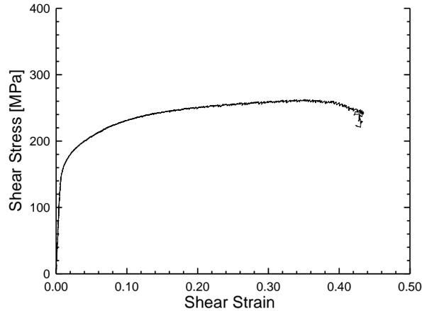
Fig. 4 Shear stress strain curve for 2024-T351 aluminum.
