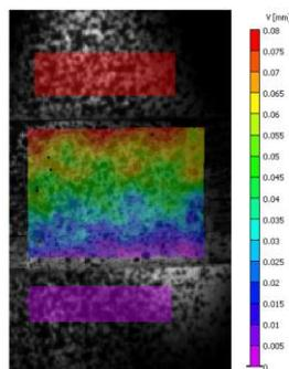
Fig. 7 DIC data from a tensile SHB test on Kevlar cloth.
