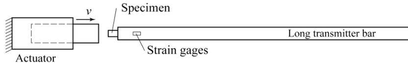
Fig. 9 Schematic of the intermediate strain rate apparatus.
