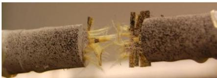
Fig. 5 Kevlar cloth following a tensile SHB test.
