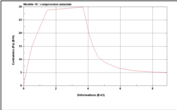
**Figure 6 :** Uniaxial Compressive Sample Test for material model 16
