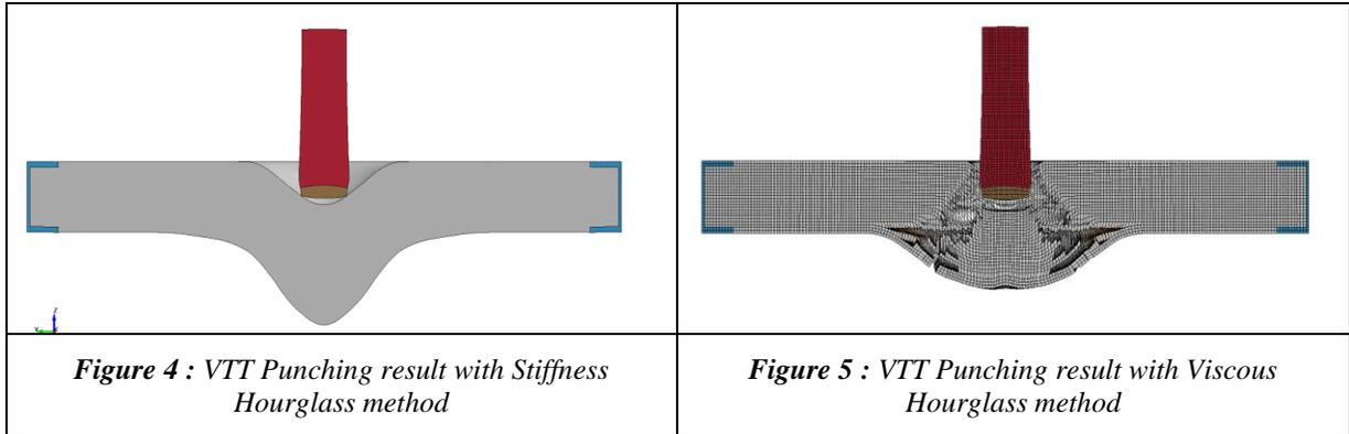
Concerning the mesh size, results are not very mesh-dependent for a non perforation test (models have regularization schemes) but for a perforation test like the VTT Punching case, a fine mesh is crucial to obtain a good erosion cone and spalling area.
