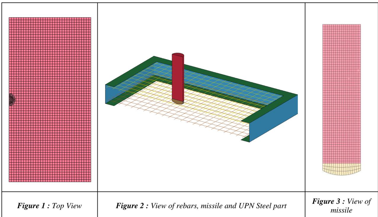
The constitutive law of steel elements is a \*MAT\_PIECEWISE\_LINEAR\_PLASTICITY able to model the behavior of steel with a complex plasticity curve and to include strain rate effects. Engineer values are changed into true values up to striction and then interpolated using a swift law. Without stress-strain curves for different strain rates, a simple way to take into account strain rate effects is to add a Cowper-Symonds law.
