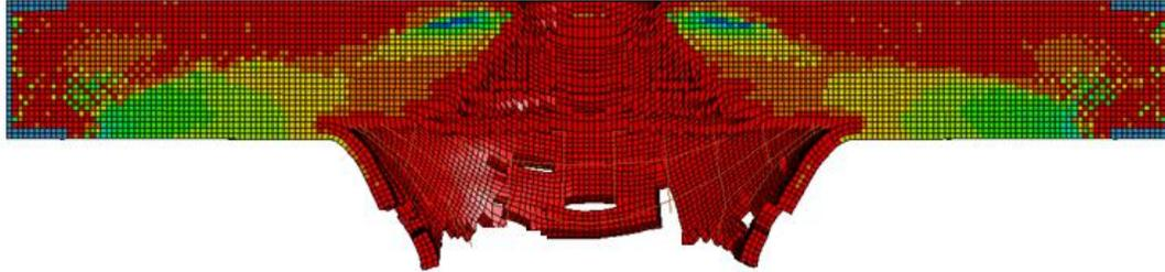
*Figure 11 : View of final damage of the slab (material 72r3)*
