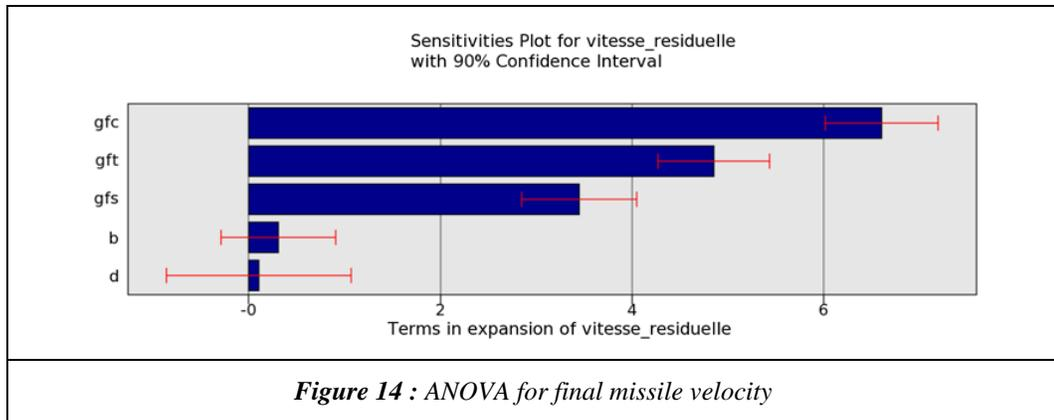
Results of this Monte Carlo analysis show that each of the fracture energy parameters can probably be used for optimization. To have the best chance to fit the experimental value, we choose to take the Gfc parameter as variable for the optimization.
