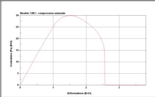
**Figure 7 :** Uniaxial Compressive Sample Test for material model 72r3
