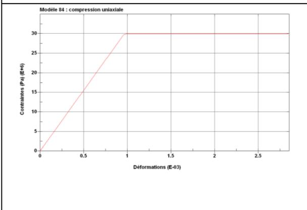
**Figure 8 :** Uniaxial Compressive Sample Test for material model 84
