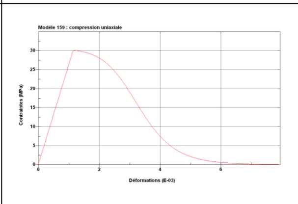
**Figure 9 :** Uniaxial Compressive Sample Test for material model 159
