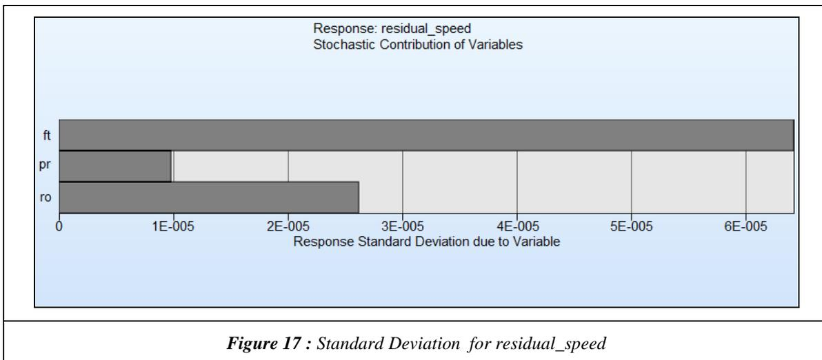
The analysis of this last sensitivity about important physical parameters shows that the optimal solution obtained after the optimization run has limited significance. Considering the natural variability of concrete parameters (two concretes are never identical and testing facilities accuracy may be unknown) affects a change of 25 % on the response, the optimal solution found before is not robust; we cannot expect to get a result with high accuracy.
