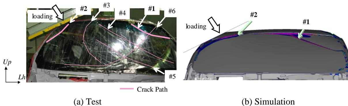
Figure 9. Comparison of glass crack propagation paths after roof strength test between test and numerical simulation.
