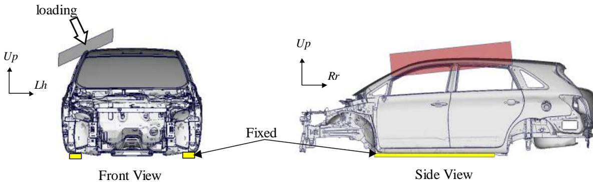
Figure 8. Roof strength model boundary condition.
