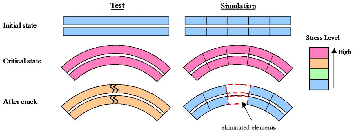
Figure 12. Schematic cross section of windshield under bending in three states.
