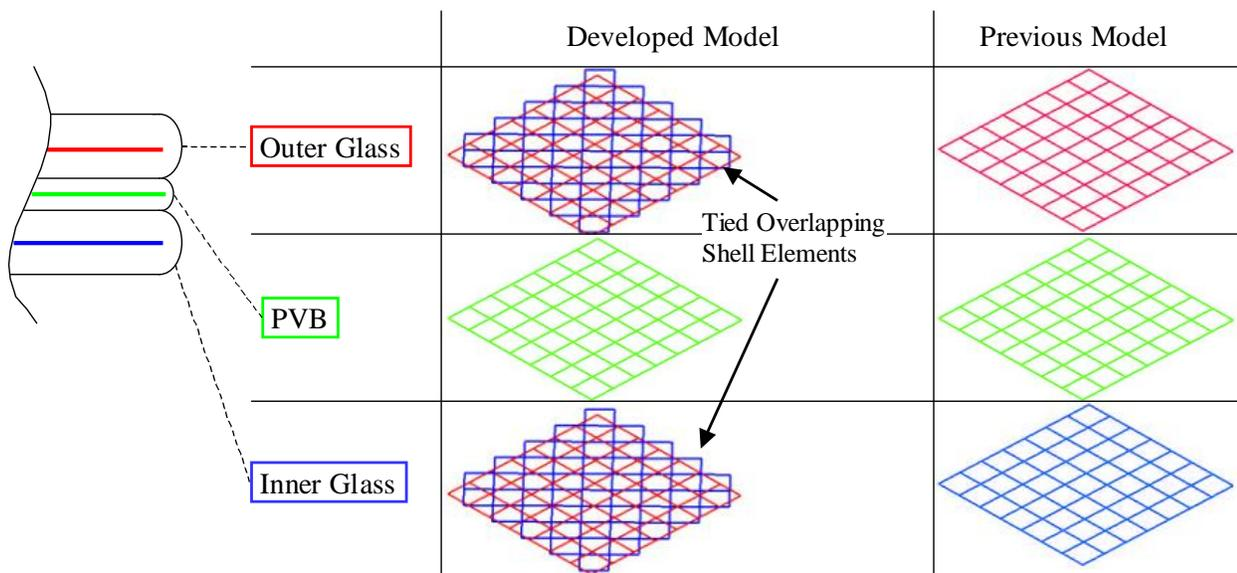
Figure 4. Comparison of laminated safety glass model.
