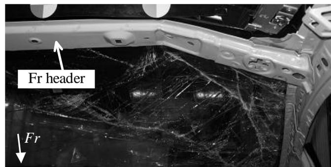
Figure 5. Inside view around front header after test.
