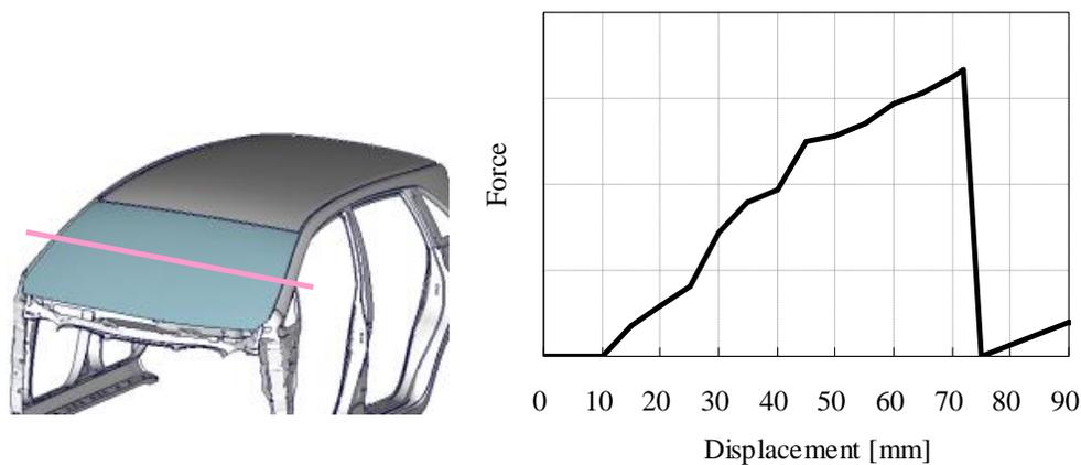
Figure 11. Windshield force versus displacement (simulation).
