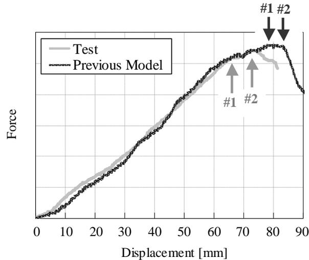
Figure 2. Comparison of force versus displacement during roof strength test between test and numerical simulation.
