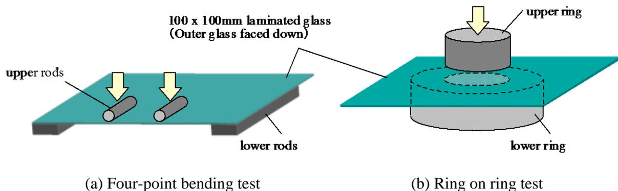
Figure 6. Comparison of test methods.
