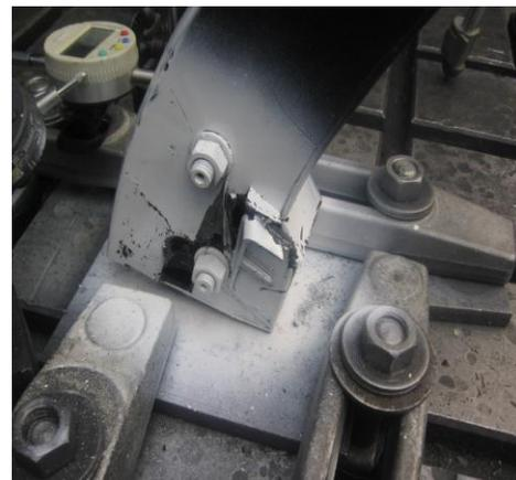
Figure 18 Failure due to Compression
