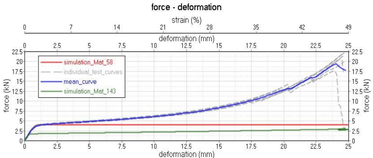
Fig.9: Force - deformation diagram for compression in tangential direction (TR and TL).
