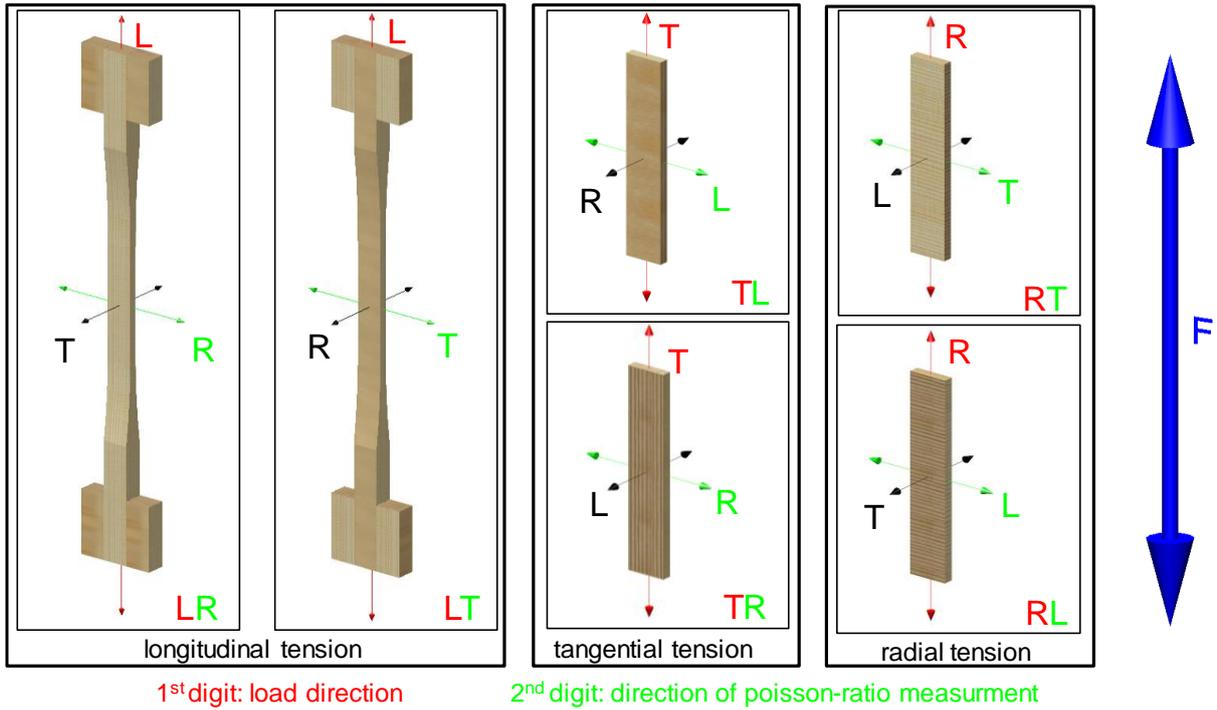
Fig.1: Samples for tension tests in all its six anatomical directions.
