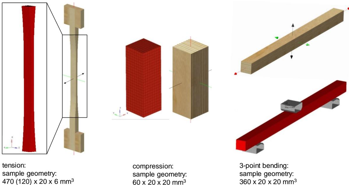
Fig.4: Modelling of the samples: tension (left), compression (middle), bending (right).
