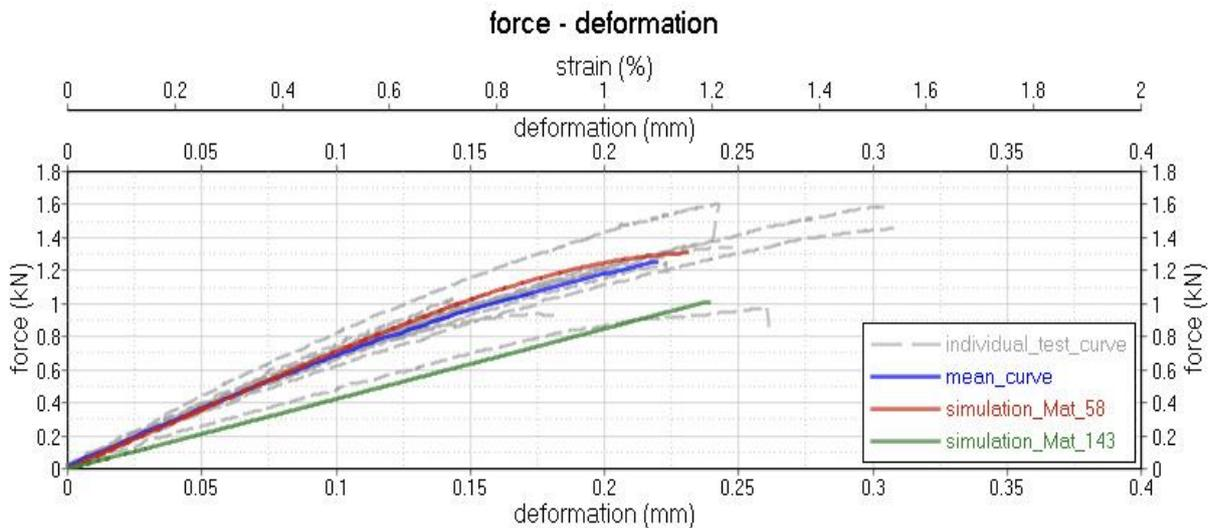
Fig.7: Force - deformation diagram for tension in radial direction (RL and RT).
