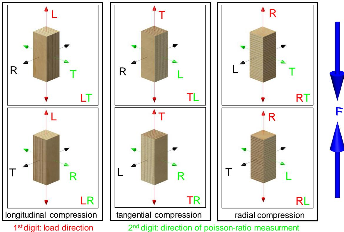
Fig.2: Samples for compression tests in all its six anatomical directions.
