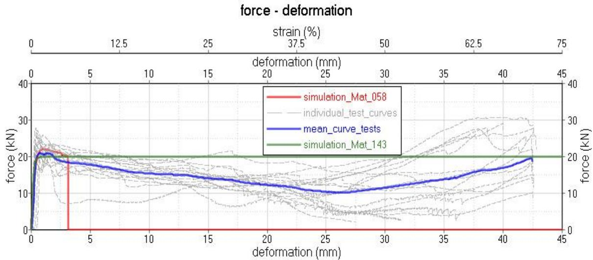
Fig.8: Force - deformation diagram for compression in longitudinal direction (LR and LT).
