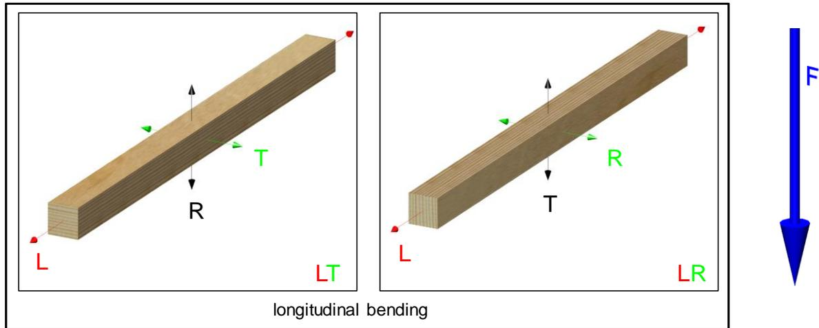
1<sup>st</sup> digit: direction of the beam axis      2<sup>nd</sup> digit: sample width (perpendicular to load direction)
