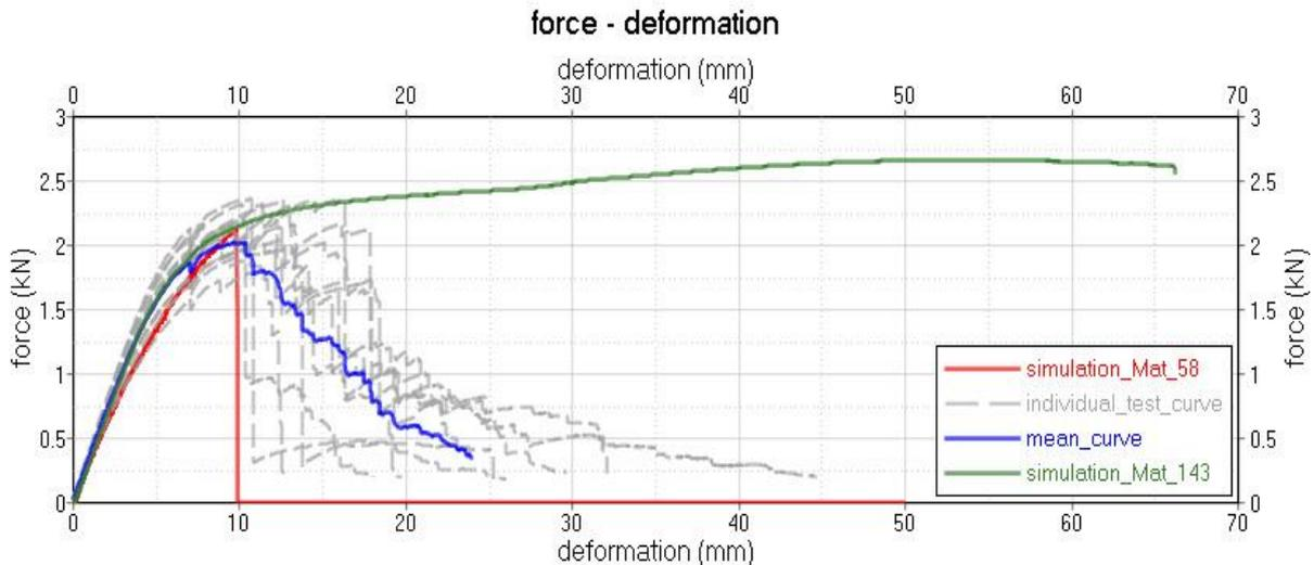
Fig.11: Force - deformation diagram for 3-point bending (LR and LT).
