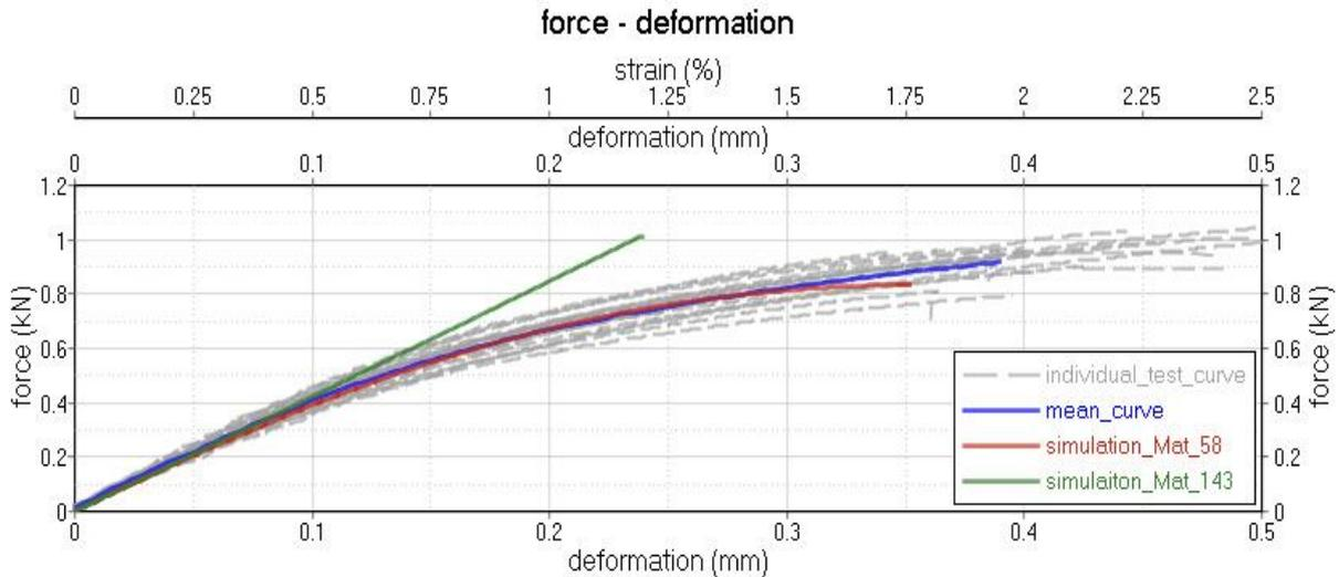
Fig.6: Force - deformation diagram for tension in tangential direction (TR and TL).
