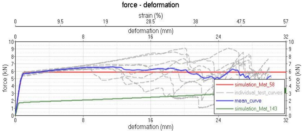
Fig.10: Force - deformation diagram for compression in radial direction (RL and RT).
