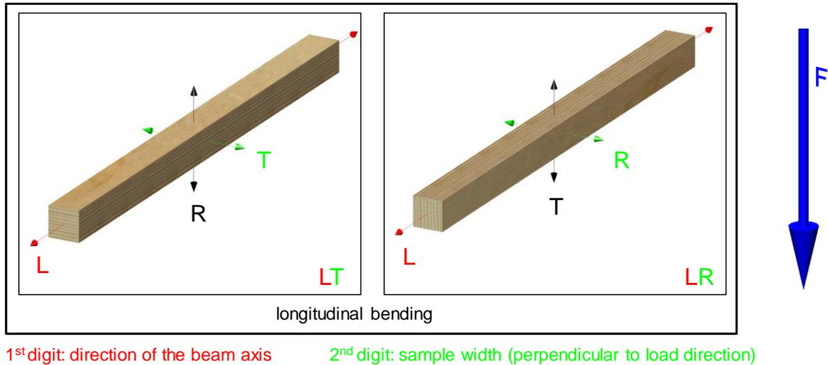
1<sup>st</sup> digit: direction of the beam axis      2<sup>nd</sup> digit: sample width (perpendicular to load direction)
