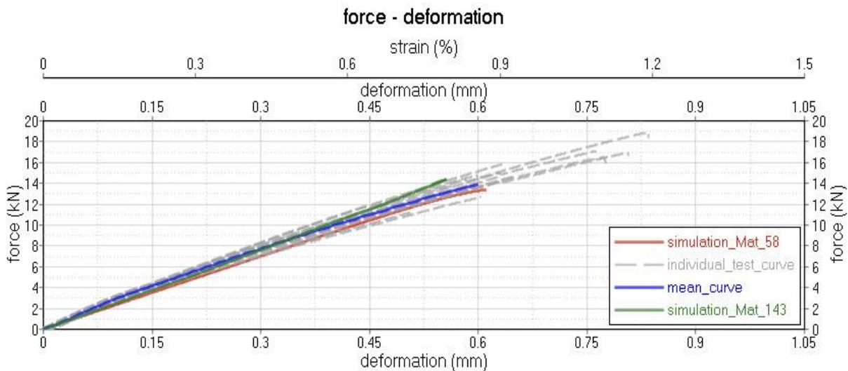
Fig.5: Force - deformation diagram for tension in longitudinal direction (LR and LT).
