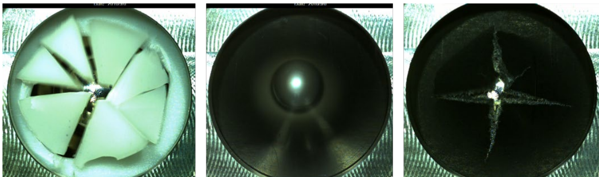
Fig.2: different failure modes: left – POM (brittle), middle- PC/PET (ductile), right – PPLGF30
