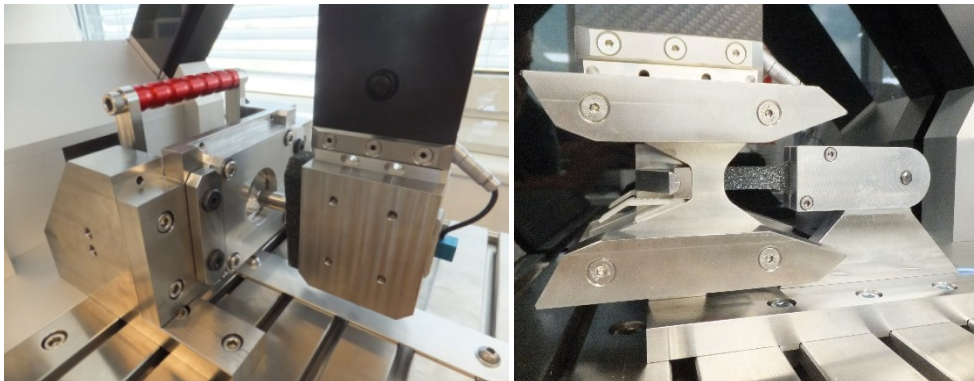
Fig.1: left – puncture test, right – new test method in IMPETUS™: dynamic tensile test
