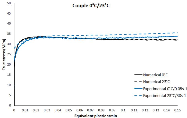
Fig. 11. Correlation study: Couple tested at 0°C and +23°C
