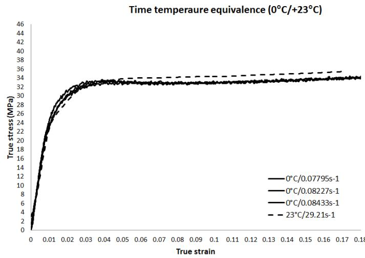
Fig. 8. Couples tested at 0°C and +23°C
