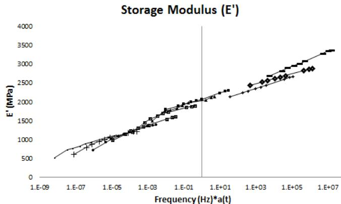
Fig. 3. Storage modulus of the master curve versus frequency range\*shift factors
