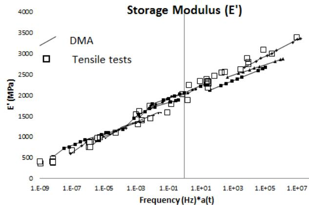
Fig. 4. Determination of the elastic modulus from two test methods: DMA and tensile tests
