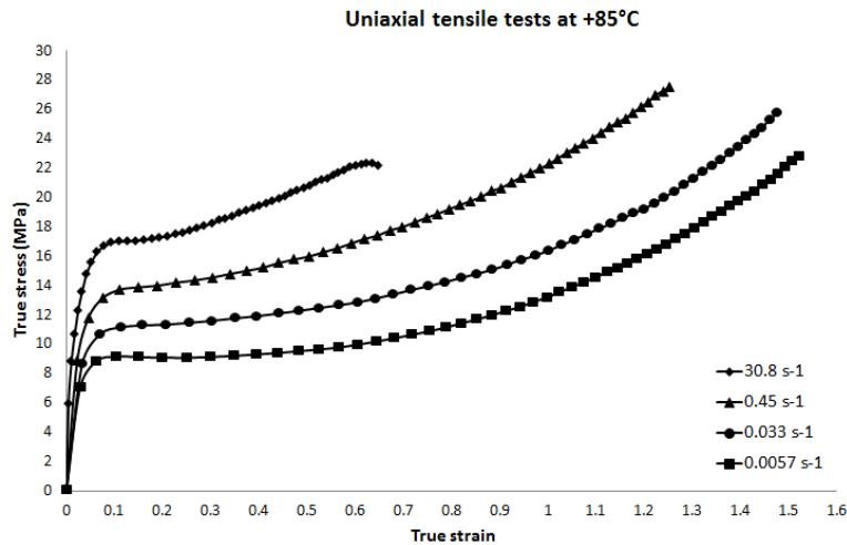
Fig. 5. Uniaxial tensile tests at  $+85^\circ\text{C}$
