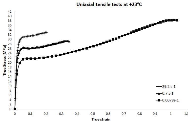
Fig. 6. Uniaxial tensile tests at +23°C
