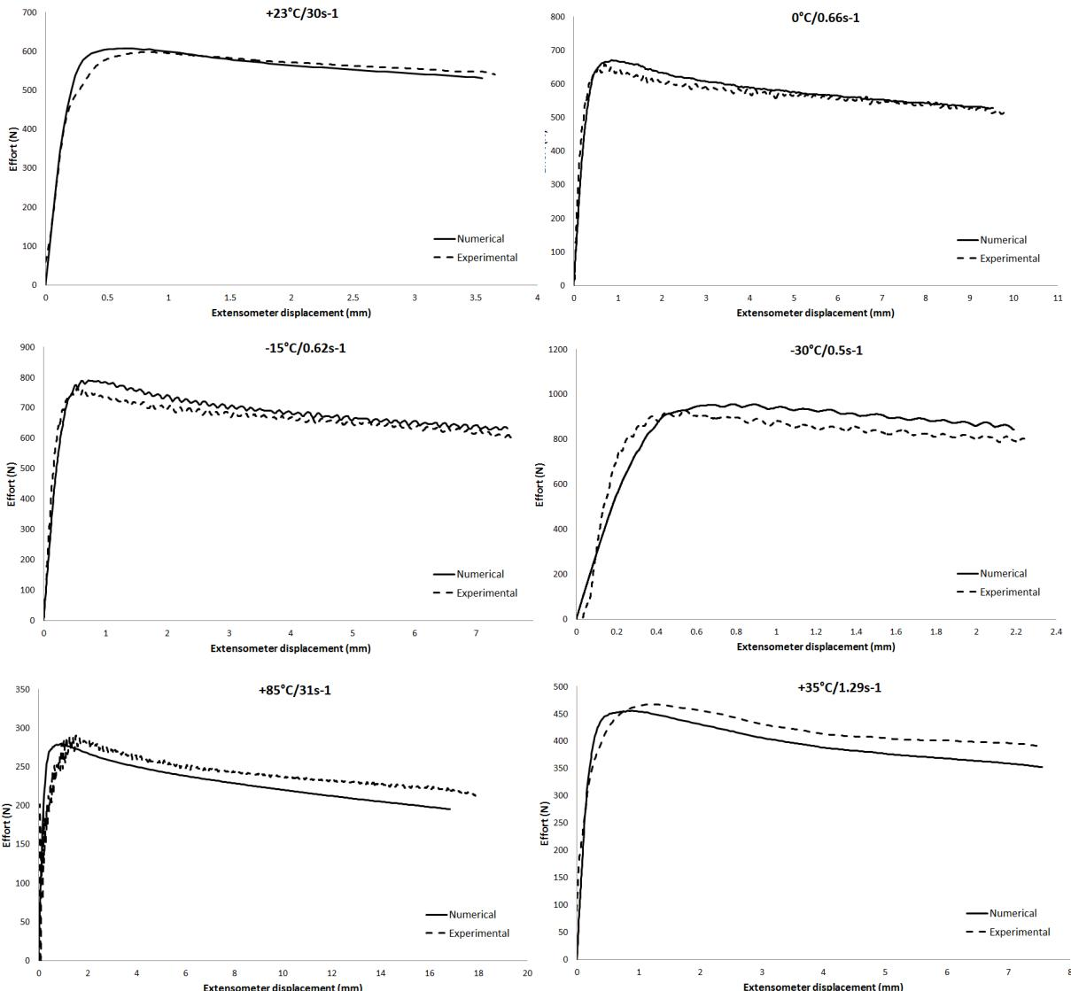
Fig. 10. Correlation study at different strain rates and temperatures
