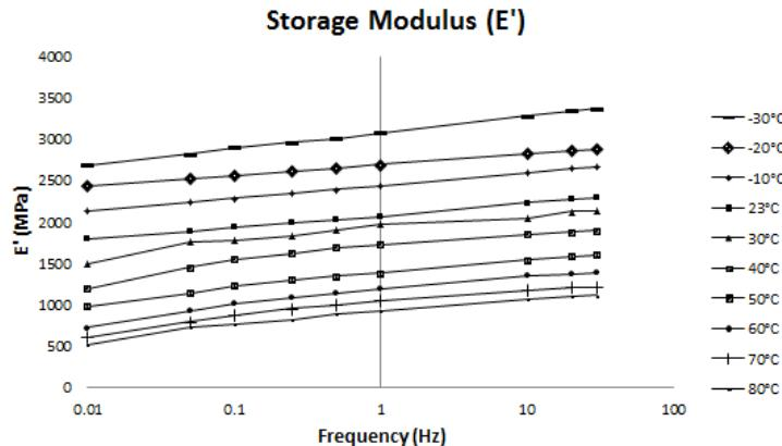
Fig. 2. Storage modulus versus frequency at different temperatures.
