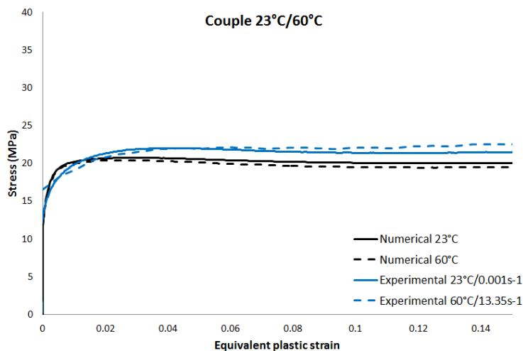
Fig. 12. Correlation study: Couple tested at 23°C and +60°C
