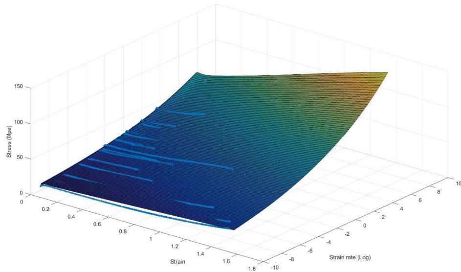
Fig. 7. 3D behavior surface of the P/E-MD15 impact modified
