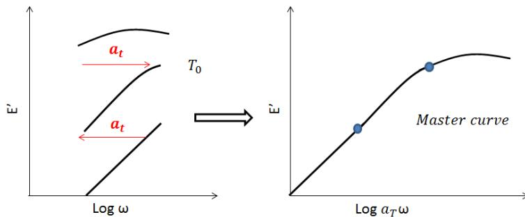
Fig. 1. Building of a master curve
