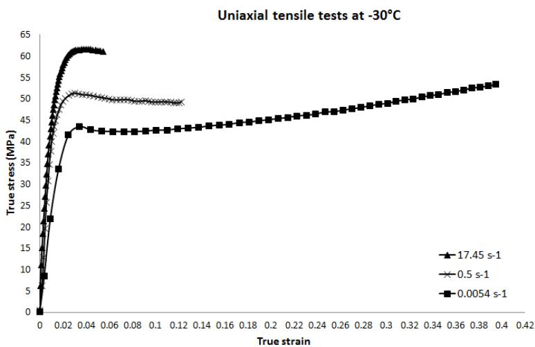
Fig. 7. Uniaxial tensile tests at -30°C
