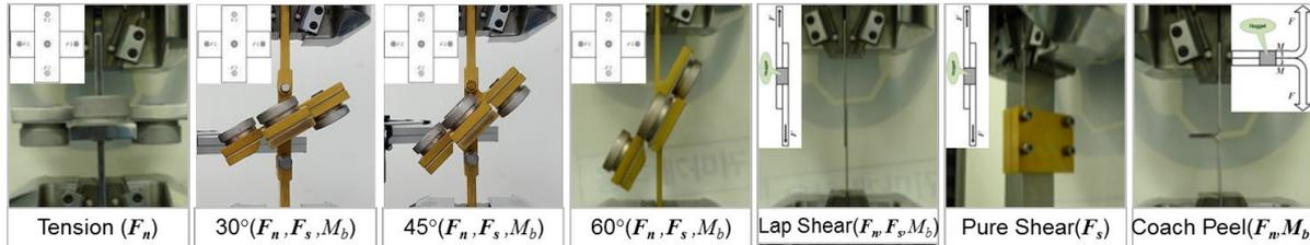
Fig.2: Failure test procedure for newly proposed failure model
