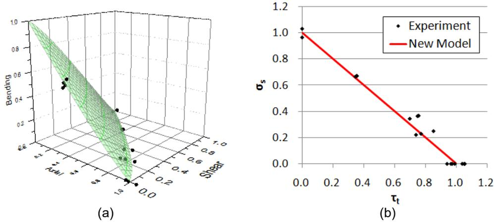
Fig.7: Failure surface of DQ steel: (a) Wung model; (b) New model.
