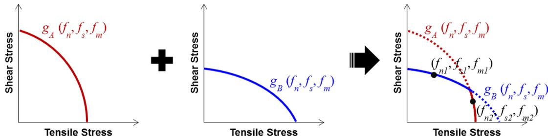
Fig.9: Consideration of fracture surface for dissimilar stack-up.
