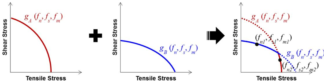
Fig.9: Consideration of fracture surface for dissimilar stack-up.
