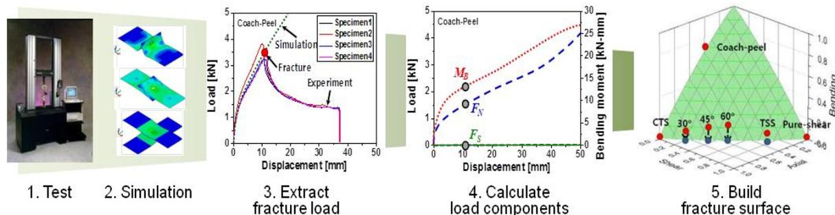
Fig.3: Hybrid method to obtain the failure load with respect to test conditions
