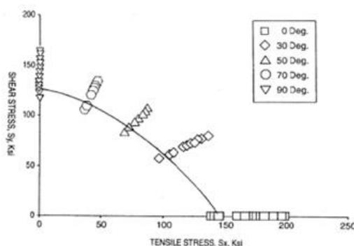
Fig. 1: Spot weld failure model proposed by Lee et al. [9]
