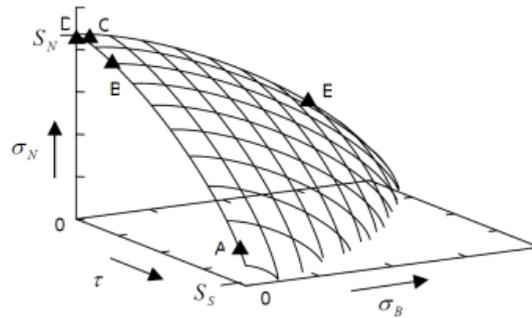
Fig.4: Spot weld failure model proposed by Seeger et al. [13], [14]
