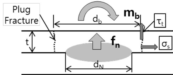
Fig.5: Schematic diagram for load components of a spot weld.
