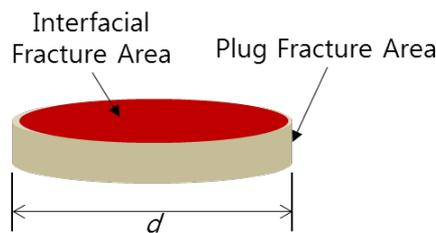
Fig.6: Schematic diagram for fracture area of a spot weld
