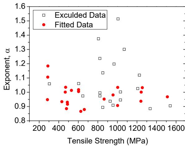
Fig.8: Variation of shape parameter,  $\alpha$  with respect to the tensile strength.
