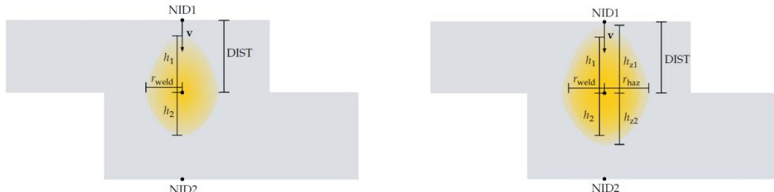
*Fig.8: Visualization of the input parameters of **\*BOUNDARY\_TEMPERATURE\_RSW**. On the left, only the weld nugget is specified; on the right also a HAZ is defined*
