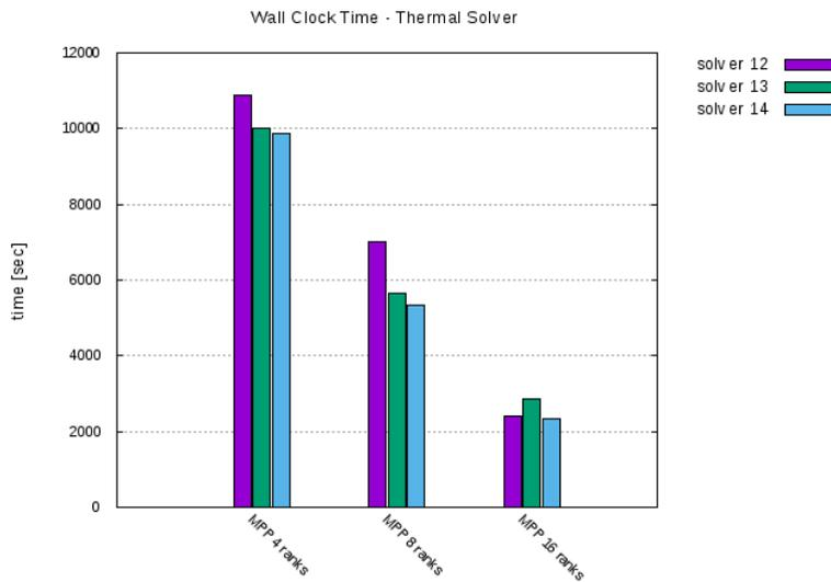
Fig. 6: Wall clock time details – time spent in thermal solver algorithm
