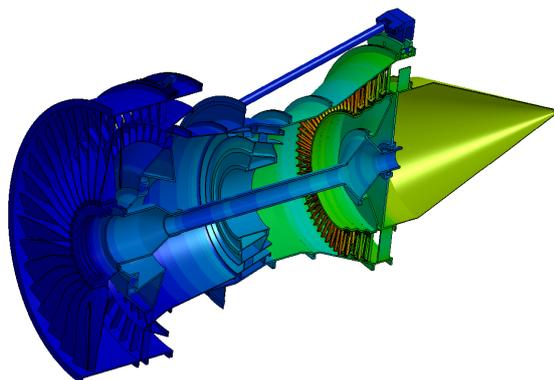
Fig. 1: Rolls Royce Representative Engine Model
