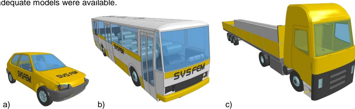
Fig.4: Vehicle FEM models: a) passenger car, b) bus, c) articulated truck
