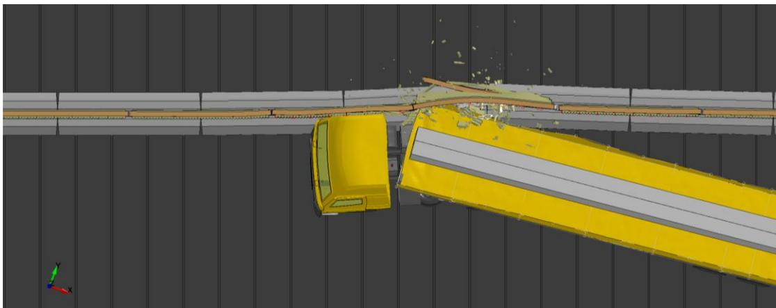
Fig.10: TB81 crash test: major failure of the barrier
