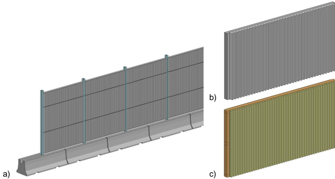
Fig.3: Barrier FEM model: a) whole barrier, b) concrete panel, c) Velox panel with wooden frame
