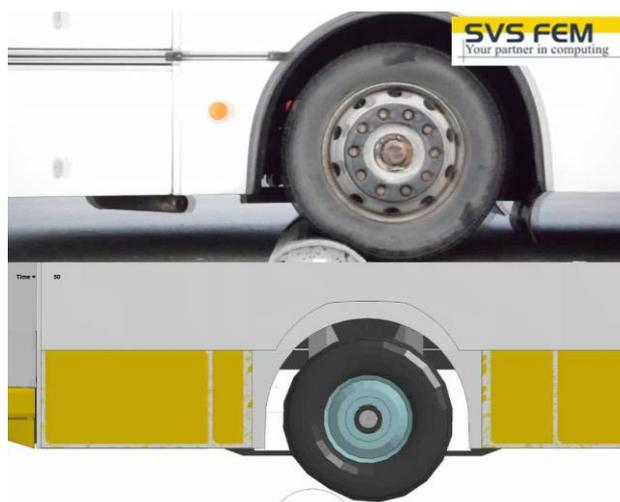
Fig.5: Vehicle FEM model testing: Bus model curb test
