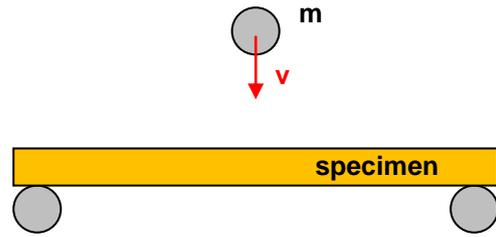
Fig.7: Bar impact test
