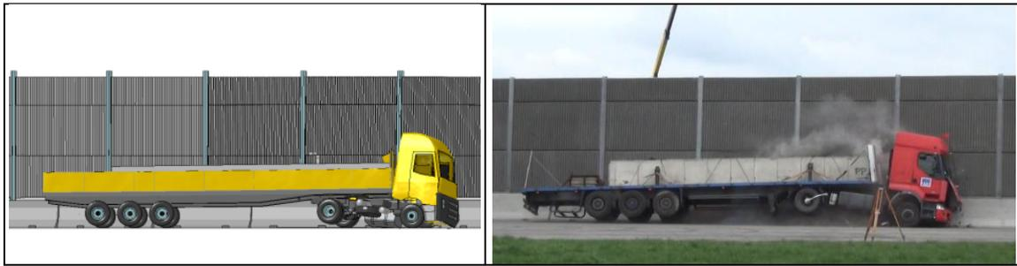
Fig.9: TB81 crash test: simulation – experiment comparison
