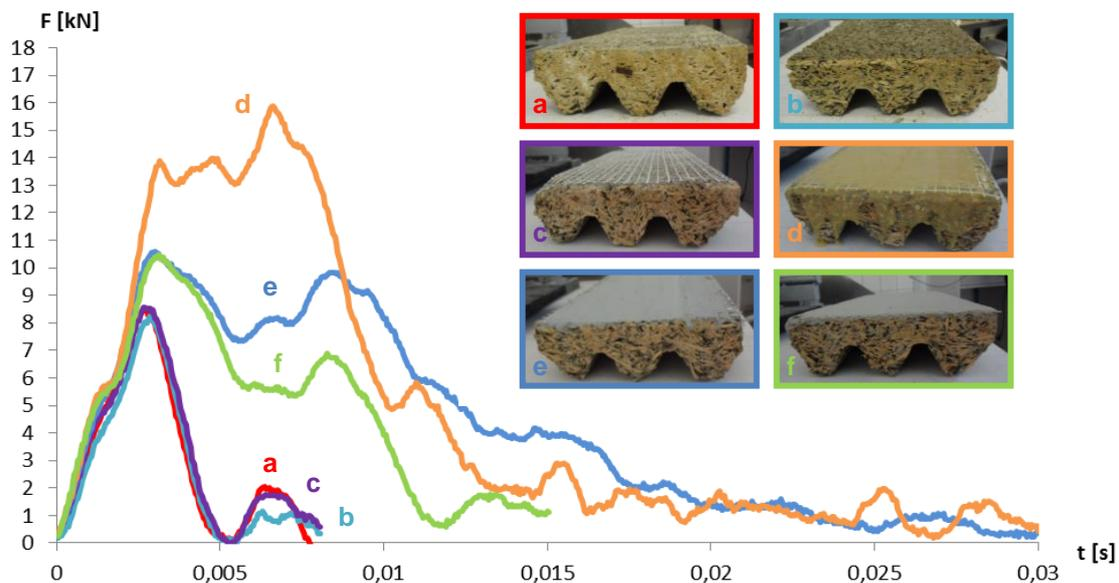
Fig. 11: Impact resistance of proposed Velox back face treatments: a) Velox, b) Velox + epoxy glue, c) Velox + fiberglass mesh, d) Velox + fiberglass mesh + polyurethane resin, e) Velox + fiberglass mesh + polyurea, f) Velox + fiberglass mesh + common wall coating
