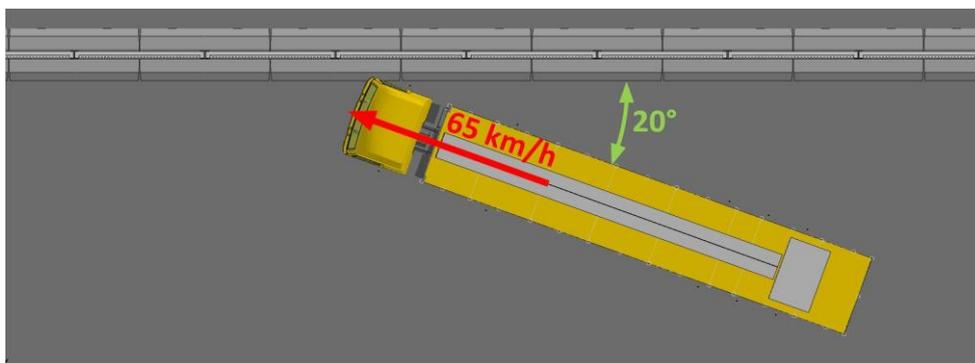
Fig.2: TB81 crash test scheme
