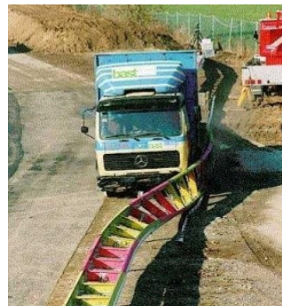
Fig. 3 Real test of a vehicle restraint system with a lorry.
