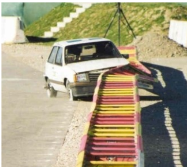
Fig. 2: Real test of a vehicle restraint system with a car.
