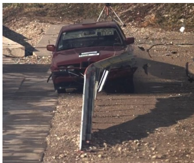
Fig. 4: Real test of a barrier ESP 2.0. BAST, TB32 2011-7D-01.
