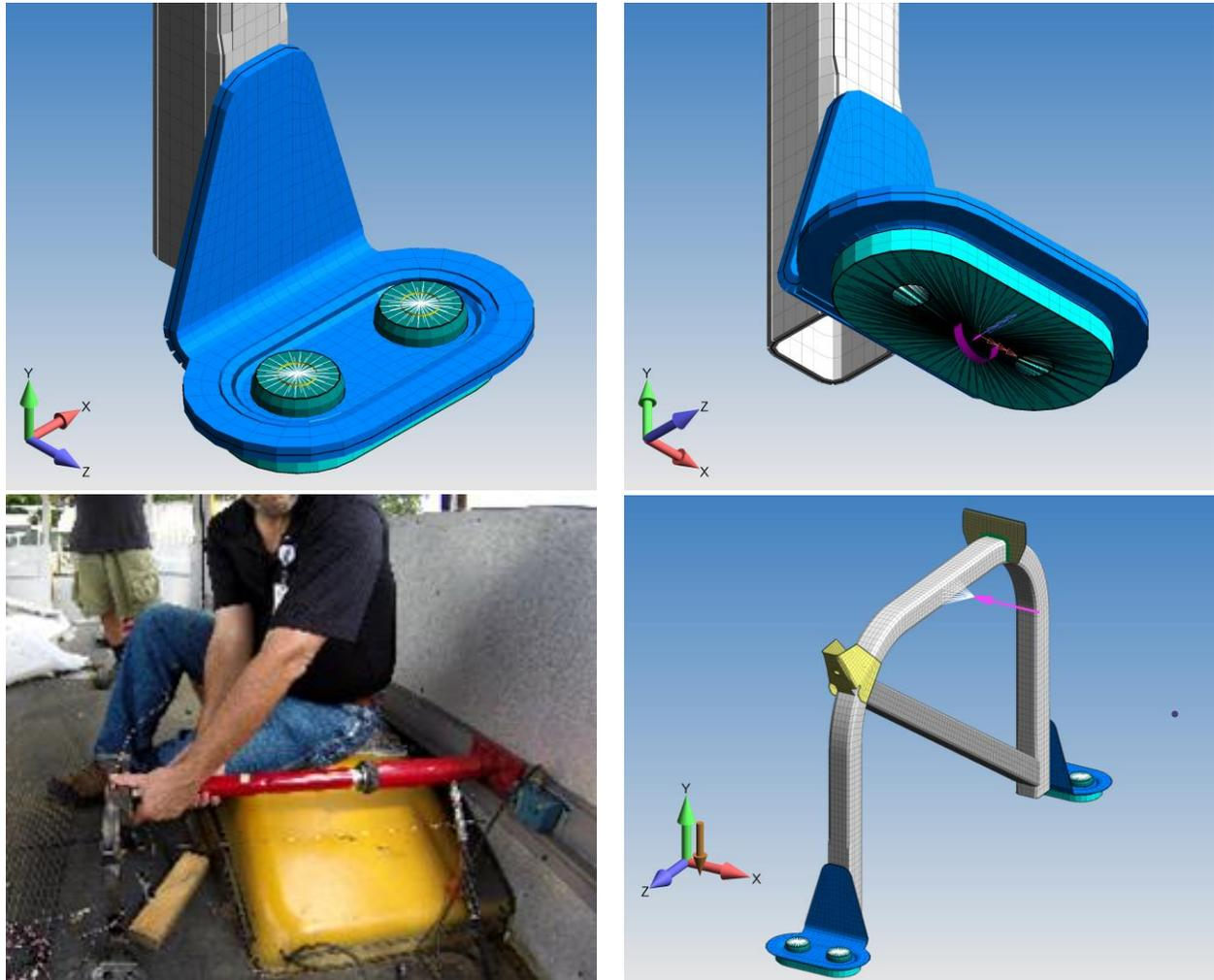
Fig.5: Seat foot / bus floor interface stiffness testing
