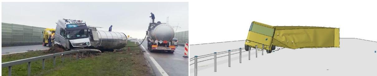
Fig.13: Comparison of numerical simulation 38/65/07/s (right) and a real road accident (left). (photo source: General Director for National Roads and Motorways – GDDKiA, Poland)
