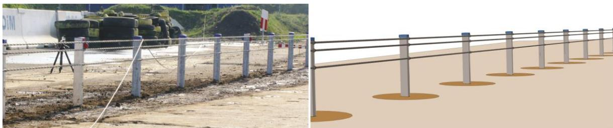
Fig.8: Full-scale structure (left) and its computational model (right).
