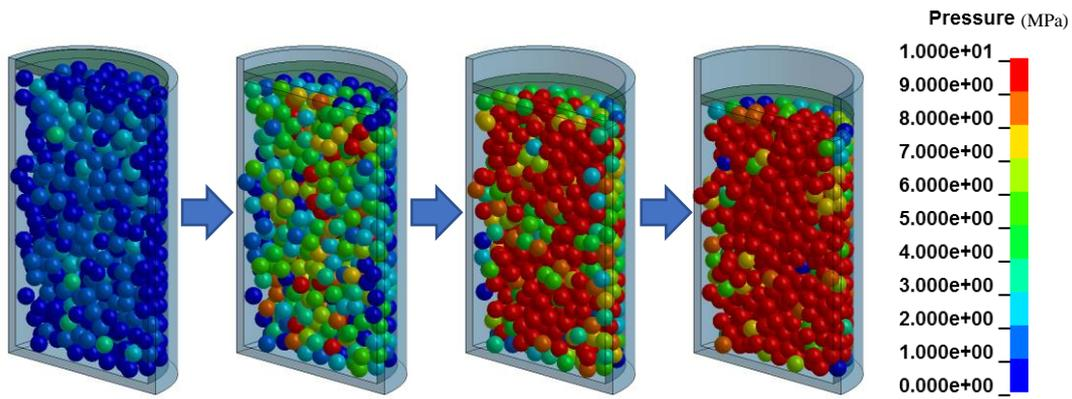
Fig.1: Simulation of polymer pellet compression (cross section view)
