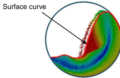
Fig.7: Surface curve of the original ( $r=1.0$  mm) model as target curve of parameter identification
