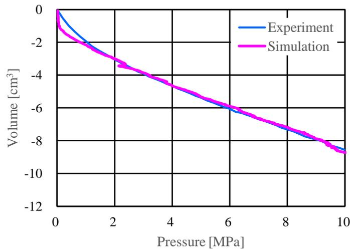
Fig.2: Pressure-volume relations for experiment and simulation
