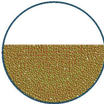
Fig.3: Example of generated DEM particles in the specified packed region
