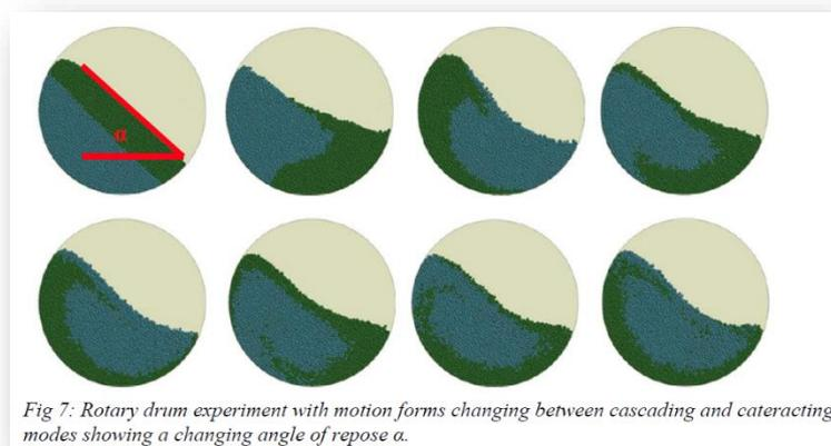
Fig 7: Rotary drum experiment with motion forms changing between cascading and cateracting modes showing a changing angle of repose  $\alpha$ .
