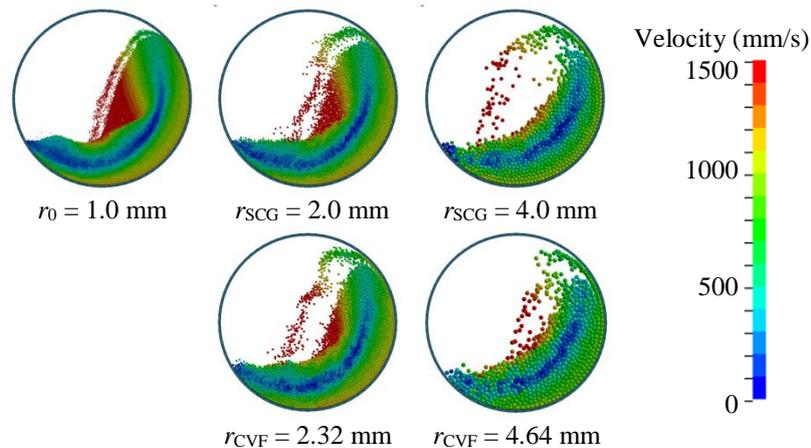
Fig.4: Comparison of shape of particles for the original, SCG and CVF model
