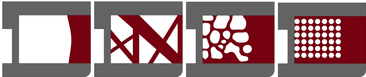
Fig.6: Selected optimal topologies. These are given the names from the left LS-TaSC 0.3, Topobox, LS-TaSC 0.45 and Hole lattice.
