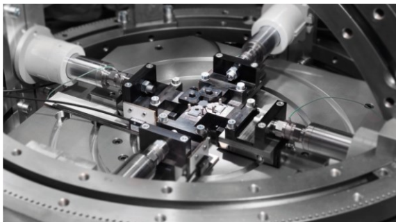
Fig.6: Biaxial tensile testing setup.
