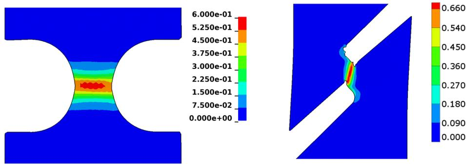
Fig.5: Strain fields optically measured for a notched and a shear specimen in 90° (equivalent strain).
