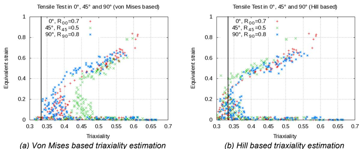
Fig.2: Strain-triaxiality paths based on the triaxiality estimation of the tensile test in three directions. All diagram data were calculated exclusively from the strain fields obtained experimentally.
