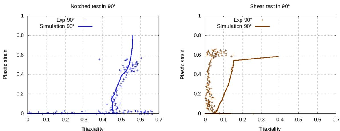
Fig.7: Strain-triaxiality paths for the notched and shear specimens: Comparison between estimation (Hill-based) and simulation (\*MAT\_036E with HOSF=1).
