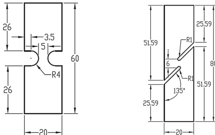
Fig.4: Dimensions of the notched and shear specimens.
