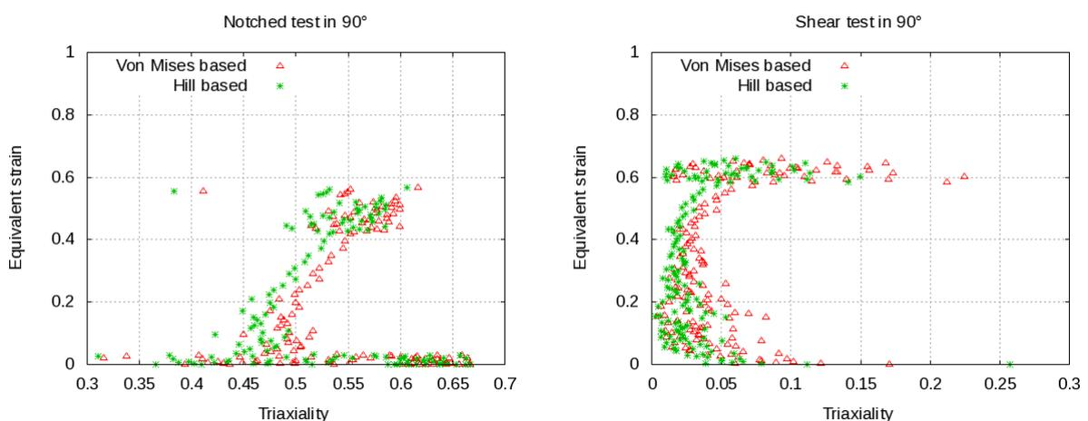
Fig.6: Strain-triaxiality paths from experimental data. The triaxiality was calculated using the von Mises (Equation 9a) and transversal Hill (Equation 13) based relations for the notched and shear test in the 90° direction.
