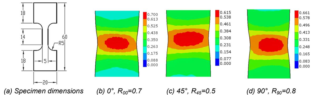
Fig.1: Tensile test: Geometry and optically measured strain fields close to failure (equivalent strain).
