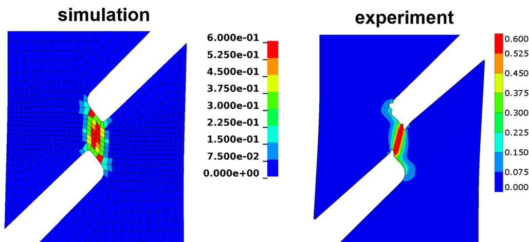
Fig.8: Comparison of the strain field (eq. strain) in the simulation and measured by the optical system
