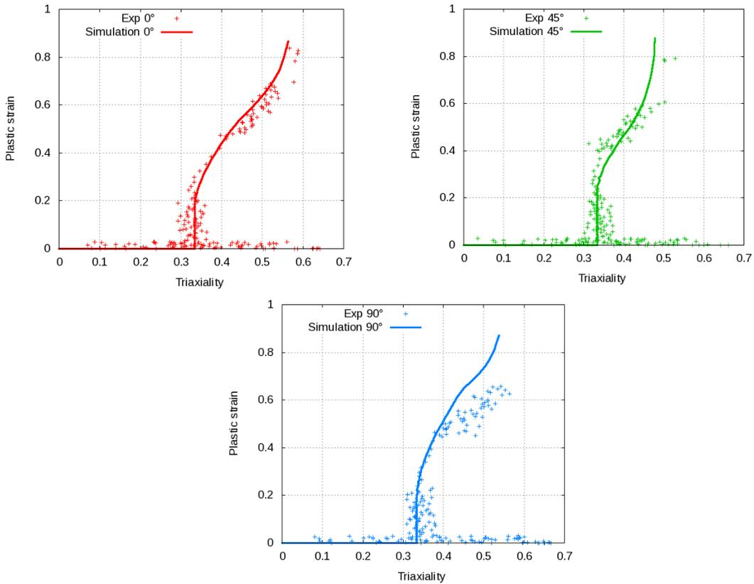
Fig.3: Comparison of the strain-triaxiality paths between experimental estimation (Hill based) and simulated values with \*MAT\_036E with HOSF=1. Note that the experimentally estimated values of the triaxiality were calculated only using the strain fields from the optical measurement.
