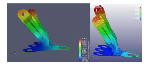
Fig.11: Left: Simulation results of full IGA assembly in Coreform Process, Right: Simulation results of an analogous linear analysis in LS-DYNA
