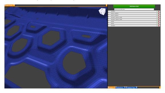
Fig.8: Ford hood geometry as a linear U-Spline in Coreform Process
