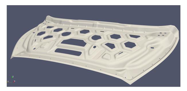
Fig.9: Ford Hood constructed as a P=2,  $C^1$  dominant U-Spline
