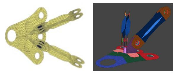
Fig.10: Left: Linear model in LS-DYNA, Right: P2 U-Spline model in Coreform Process
