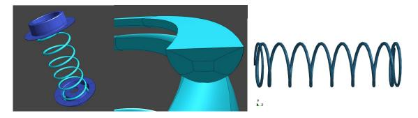
*Fig.6:* Left to right: Spring contact assembly in Coreform Process, Spring modeled with U-Spline cross section, solid spring geometry in LS-PrePost after export via **\*IGA INCLUDE BEZIER**.
