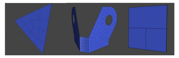
Fig.12: Unstructured meshes read into LS-DYNA. From left to right: P=2 mesh with an extraordinary point, P=2 mixed element types and mixed continuity, P=3 C2 mesh with T-junction.
