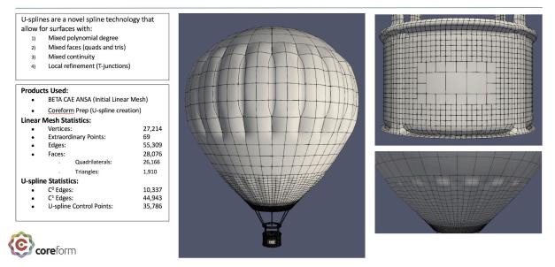
Fig.1: Example of a U-spline model, showcasing the flexible U-spline smoothness and refinement properties critical for success in simulations.
