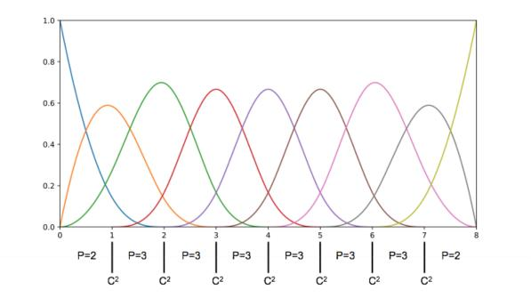
*Fig.2:* Non-uniform degree U-Spline in one dimension. Novel spline technology permits the construction of bases with varying degree while maintaining properties of partition of unity, linear independence, and positive local support. The U-Spline shown in this figure has been modified at the ends to reduce degree from P=3 to P=2 while maintaining C<sup>2</sup> continuity.
