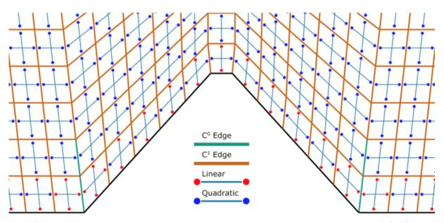
*Fig.5:* Modified quadratic U-Spline layout. Elements near boundaries (in black) or near C<sup>0</sup> edges (in green) were modified to decrease the degree and increase the characteristic length near the edges. Edges near corners were crease to C<sup>0</sup> to maintain geometric exactness.
