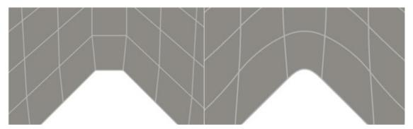
*Fig.4:* Notch geometry comparison, left: linear finite elements (*P*=1), right: U-splines with modified degree near the boundary (*P*=2).
