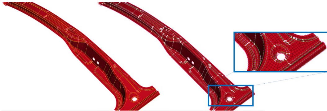
Fig.1: B Pillar CAD geometry and resulting FE Mesh.
