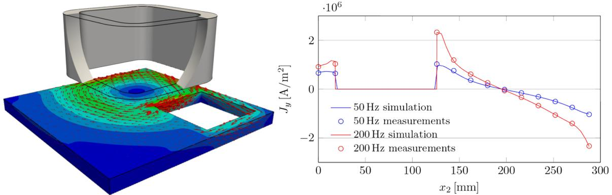
Fig.1: TEAM 7 problem: induced eddy currents (left) and comparison of numerical and measured data (right).
