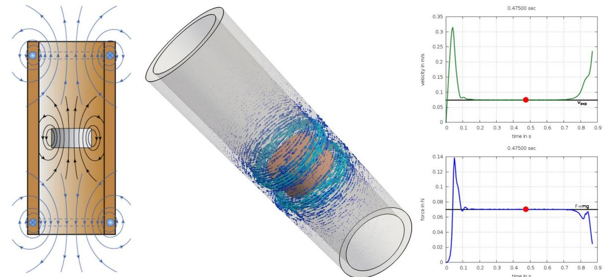
Fig.2: Magnet falling through a copper pipe: concept (left), computed eddy currents (middle), falling velocity and magnetic force (right).
