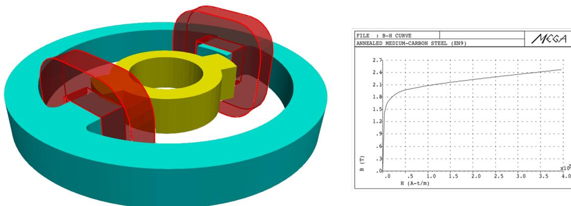
Fig.3: TEAM 24 benchmark problem: geometry (left) with coils (red), stator (blue) and rotor (yellow); nonlinear B-H curve (right).
