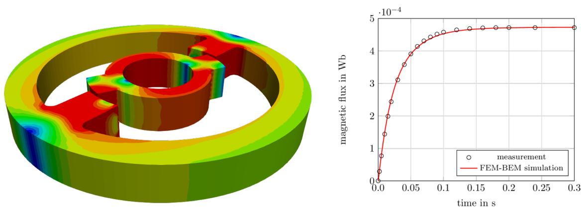
Fig.4: Numerical solution of TEAM 24 benchmark problem: magnetic flux density at the final time step (left) and flux through a specified surface with measurement data (right).
