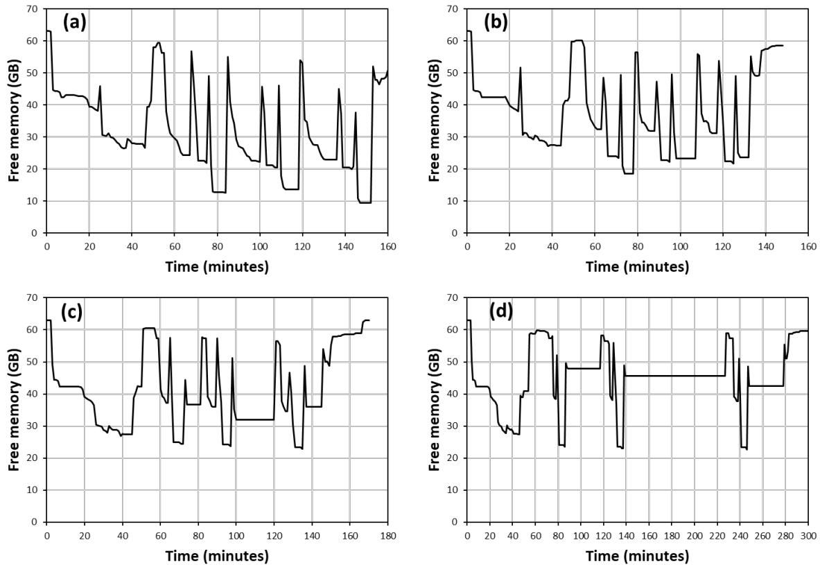
Fig.2: Available memory versus time when running the SREM on Blue Waters, with MPI ranks of 256 (a), 512 (b), 1024 (c), and 2048 (d).
