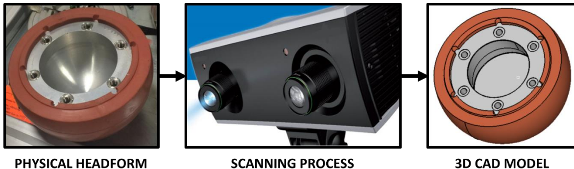
Figure 4:1 Comparison between Physical Headform Impactor and its 3D CAD Model
