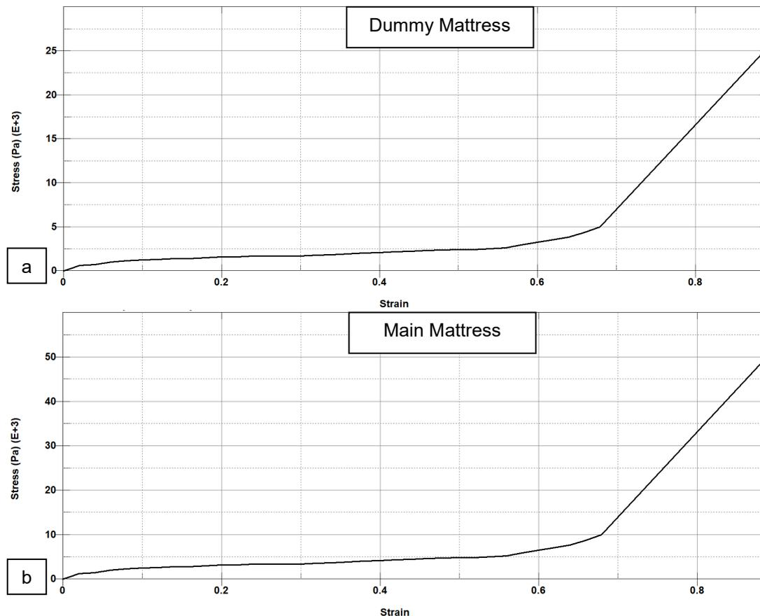
Fig.4: a) Dummy Mattress and b) main mattress load curves (stress-strain curves)
