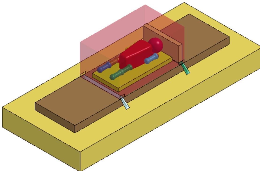
Fig.3: Wall padding added to the model
