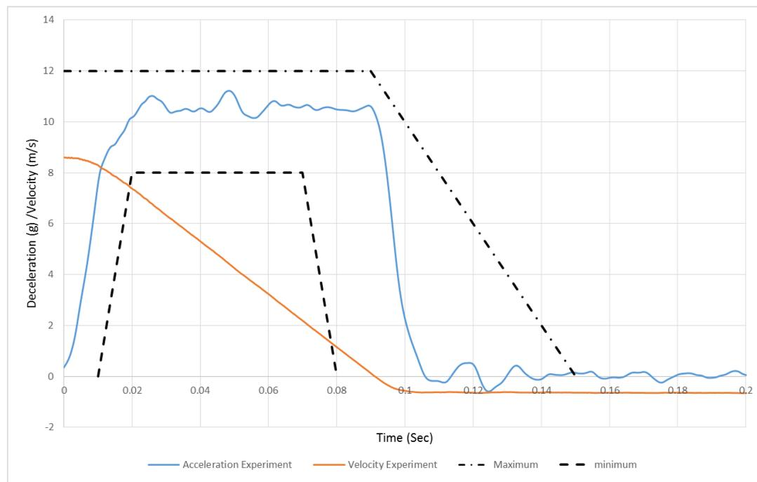
Fig.1: Acceleration (g) and velocity (m/s) against time obtained experimentally, maximum and minimum acceleration (g) against time in comply with BS EN 1789 [4]
