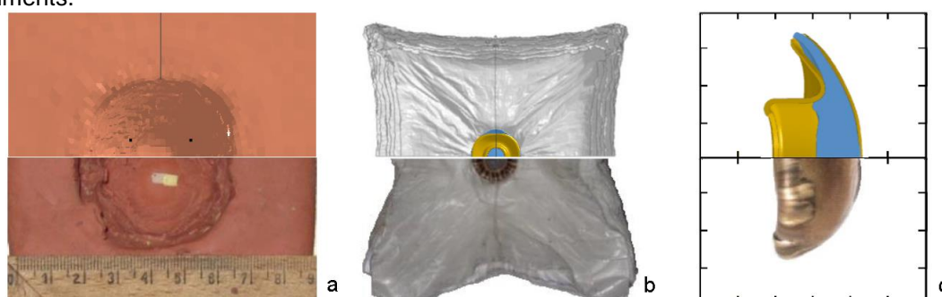
Fig.5: The results of simulations and experiments of the 9x19 mm Parabellum projectile impact into the 16 UHMWPE layers: a – indentation in clay; b – front of the sample; c – projectile after the test
