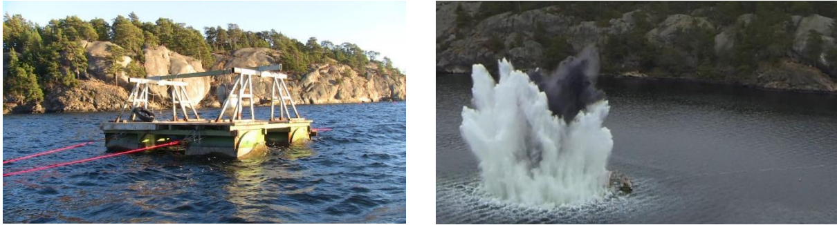
Fig.4: UNDEX experiments: steel raft for specimen carriage (left) and wave puncture at the surface (right). The experiment was conducted by the Swedish Defence Materiel Administration (FMV) in Muskö, Sweden.
