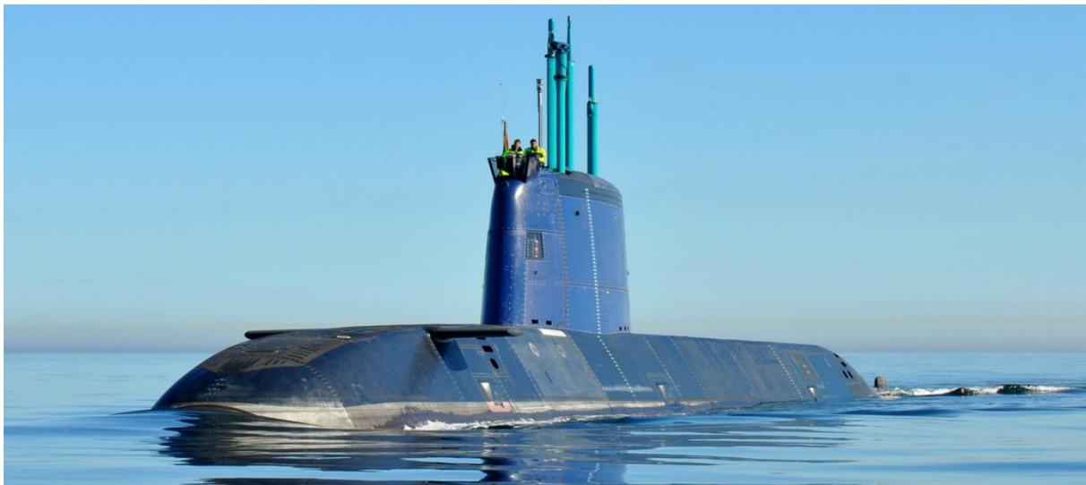
Fig. 1: A state-of-the-art conventional submarine with an upper deck consisting of mostly composite components
