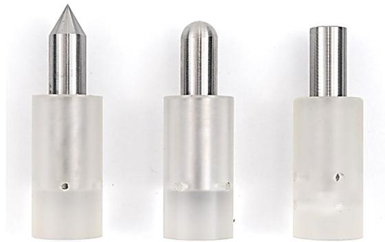
Fig. 2: Strikers with different nose shapes used in the test.
